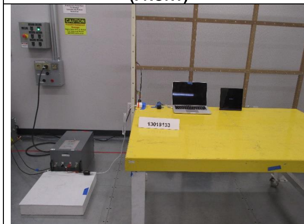
AC LINE CONDUCTED WITH HOST (FRONT)
