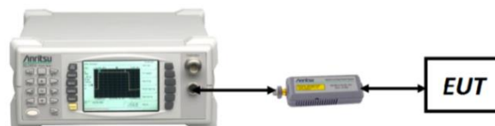
Figure 7-2. Radiated Measurement Setup for Power Meter Measurements
