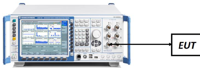
Figure 7-4. Conducted Power Measurement Setup
