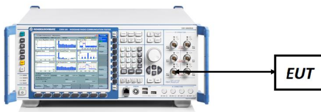
Figure 7-7. ERP/EIRP Measurement Setup
