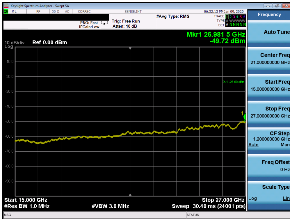
Plot 7-153. Conducted Spurious Plot (Band 7 – 20.0MHz QPSK – RB Size 1, RB Offset 0 – Low Channel)
