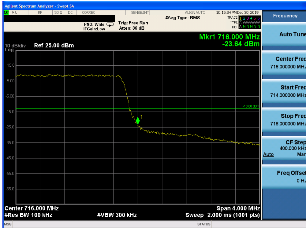
Plot 7-178. Upper Band Edge Plot (Band 17 – 5.0MHz QPSK – RB Size 25)
