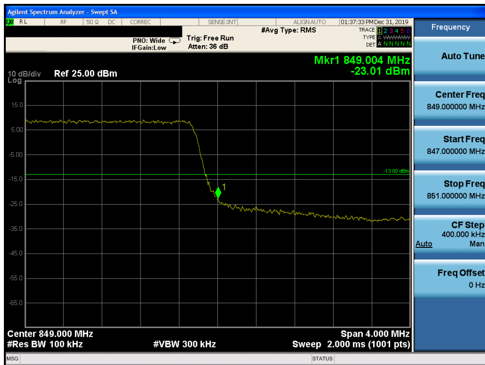
Plot 7-202. Upper Band Edge Plot (Band 26 - 5.0MHz QPSK - RB Size 25)
