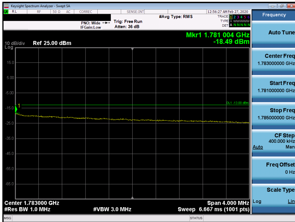
Plot 7-244. Upper Extended Band Edge Plot (Band 66 – 10.0MHz QPSK – RB Size 50)
