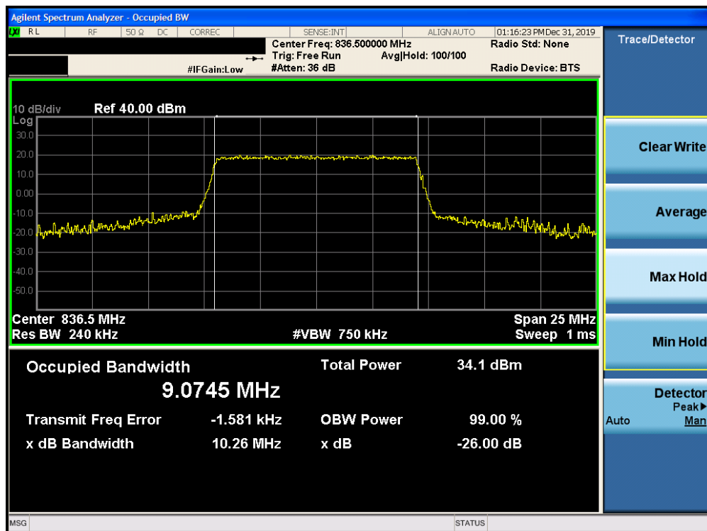
Plot 7-28. Occupied Bandwidth Plot (Band 26/5 – 10.0MHz QPSK – RB Size 50)
