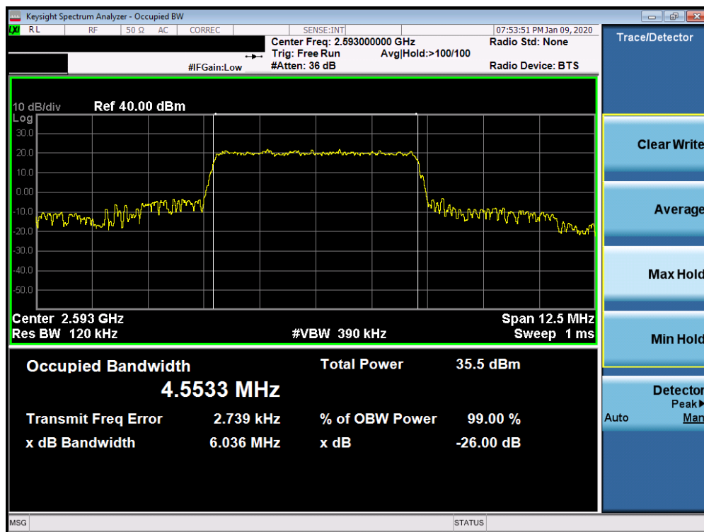
Plot 7-86. Occupied Bandwidth Plot (Band 41 – 5.0MHz 16-QAM – RB Size 25)
