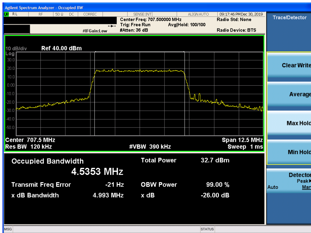
Plot 7-8. Occupied Bandwidth Plot (Band 12/17 – 5.0MHz 16-QAM – RB Size 25)
