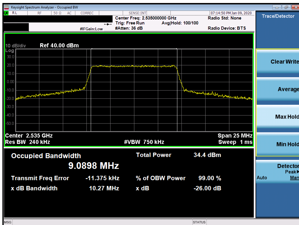
Plot 7-76. Occupied Bandwidth Plot (Band 7 – 10.0MHz QPSK – RB Size 50)
