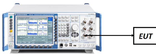
Figure 7-5. ERP/EIRP Measurement Setup
