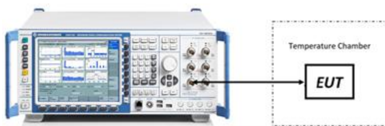
Figure 7-6. Test Instrument & Measurement Setup
