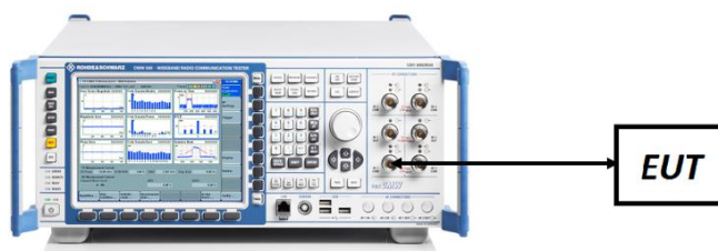
Figure 7-4. ERP/EIRP Measurement Setup
