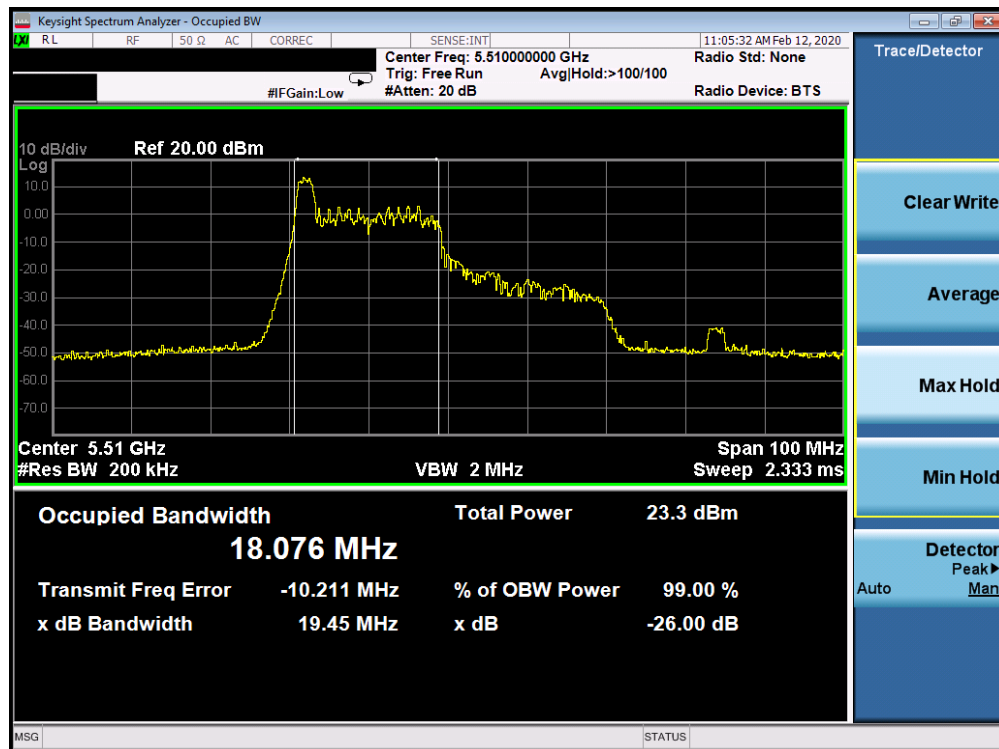
Plot 7-61. 26dB Bandwidth Plot SISO CORE 0 (40MHz BW 802.11ax Index 0 – RU26 (UNII Band 2C) – Ch. 102)
