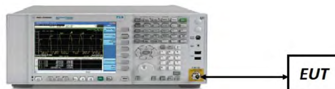
Figure 7-1. Test Instrument & Measurement Setup
