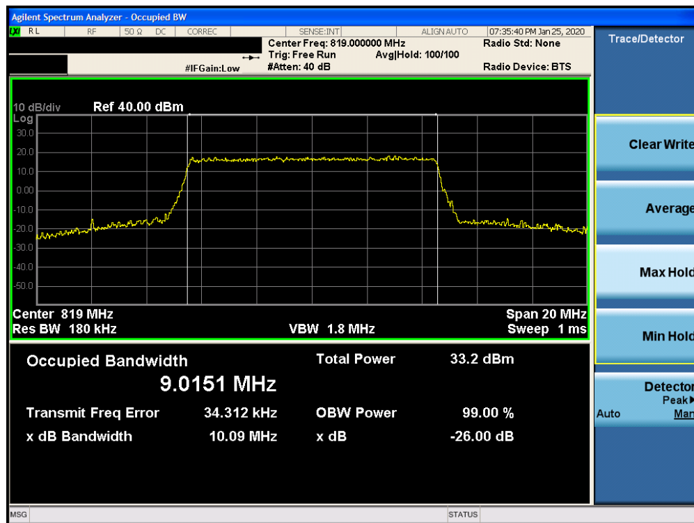
Plot 7-2. Occupied Bandwidth Plot (LTE Band 26 - 10MHz 16-QAM - Full RB Configuration)
