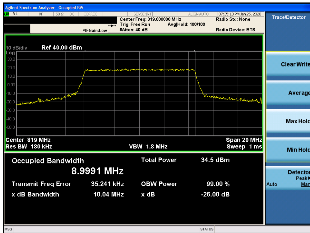
Plot 7-1. Occupied Bandwidth Plot (LTE Band 26 - 10MHz QPSK - Full RB Configuration)
