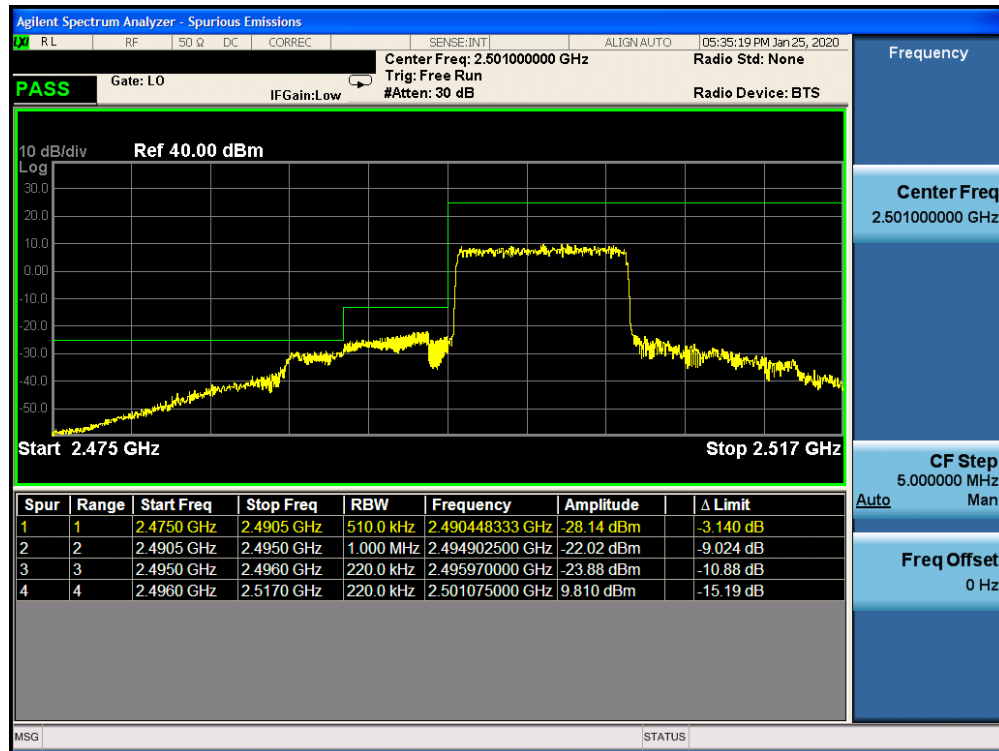
Plot 7-319. Lower ACP Plot (Band 41 – 10.0MHz QPSK – RB Size 50)
