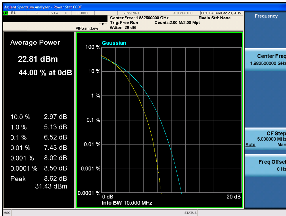
Plot 7-390. PAR Plot (Band 25 – 10.0MHz 64-QAM – RB Size 50)
