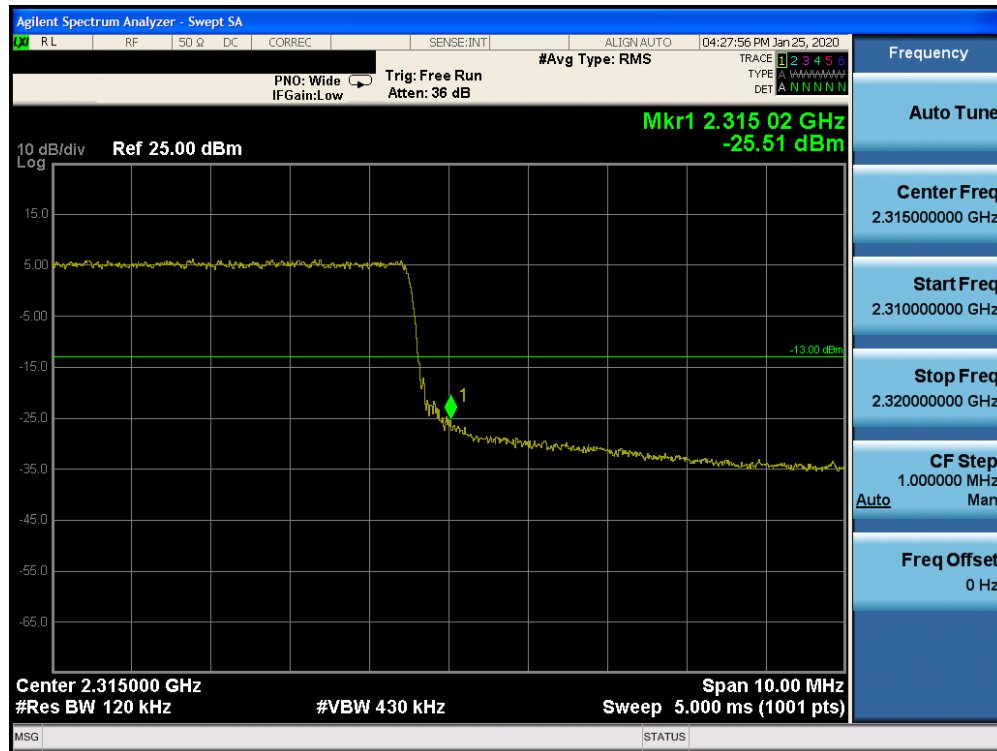
Plot 7-307. Upper Band Edge Plot (Band 30 – 10.0MHz QPSK – RB Size 50)
