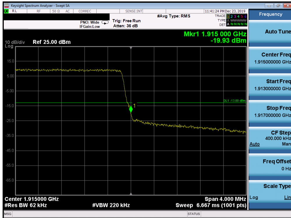
Plot 7-283. Upper Band Edge Plot (Band 25 – 3.0MHz QPSK – RB Size 15)
