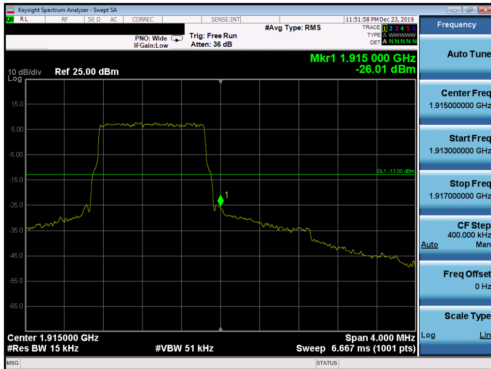
Plot 7-279. Upper Band Edge Plot (Band 25 – 1.4MHz QPSK – RB Size 6)
