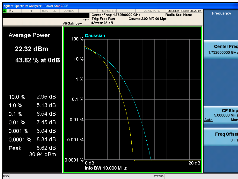
Plot 7-336. PAR Plot (Band 4 – 10.0MHz 64-QAM – RB Size 50)
