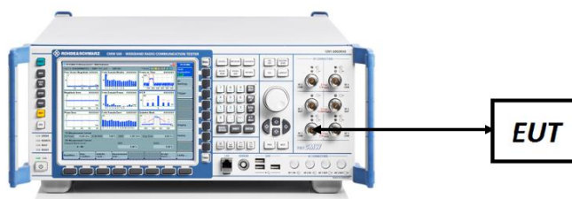
Figure 7-5. ERP/EIRP Measurement Setup
