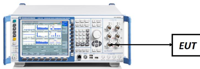
Figure 7-4. ERP/EIRP Measurement Setup
