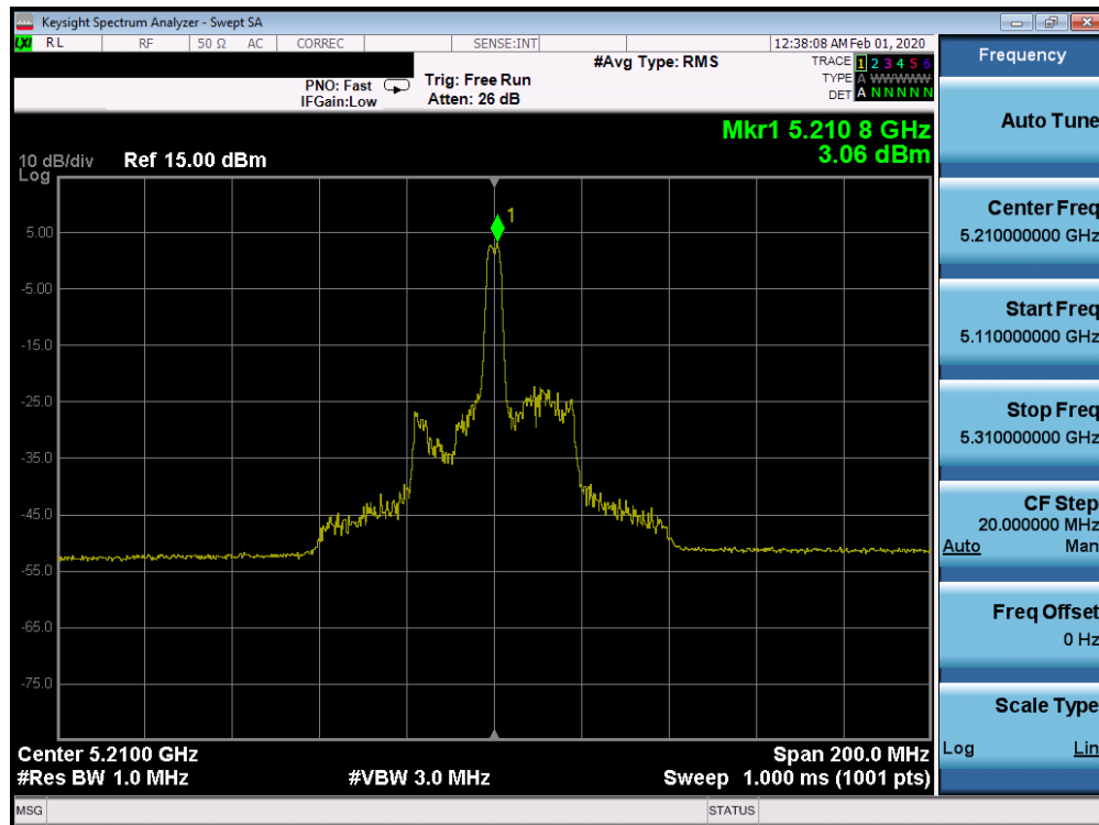
Plot 7-438. Power Spectral Density Plot ISSED SISO CORE 1 (80MHz BW 802.11ax Index 18 – RU26 (UNII Band 1) – Ch. 42)
