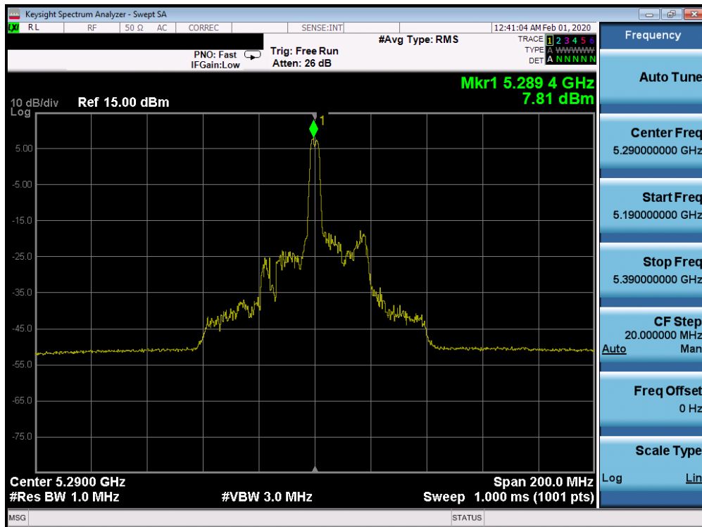
Plot 7-382. Power Spectral Density Plot SISO CORE 1 (80MHz BW 802.11ax Index 18 – RU26 (UNII Band 2A) – Ch. 58)
