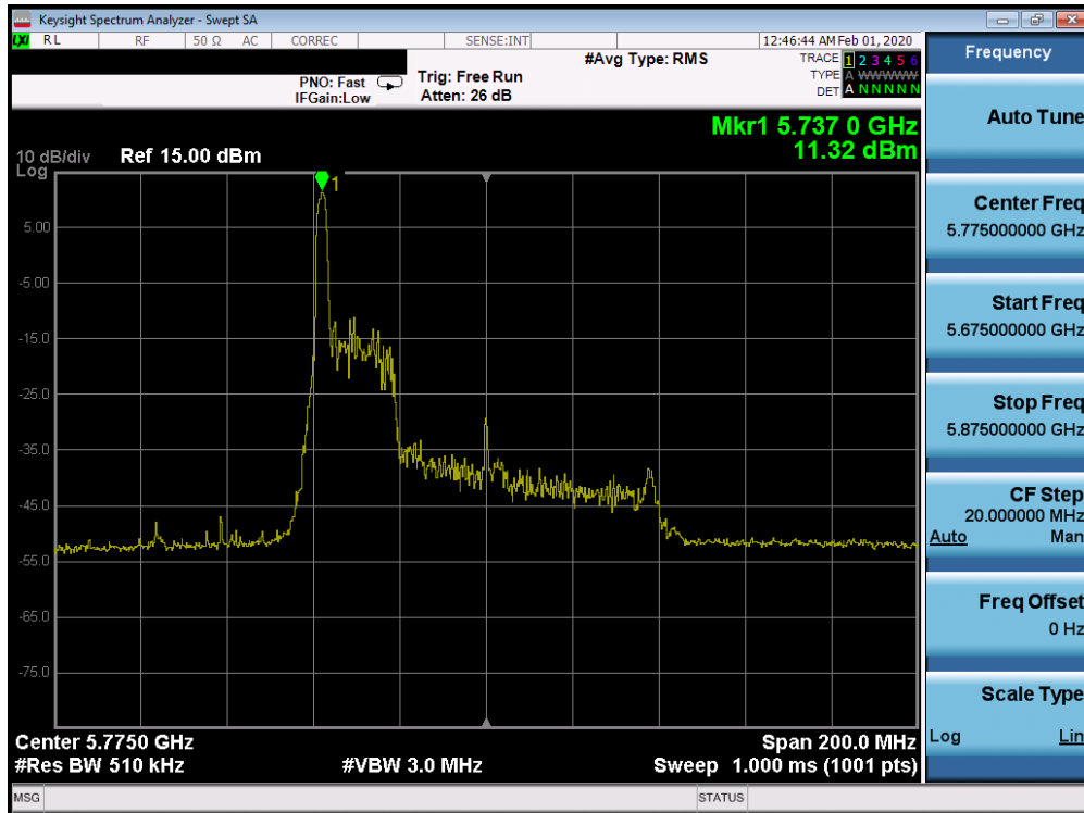
Plot 7-461. Power Spectral Density Plot SISO CORE 1 (80MHz BW 802.11ax Index 0 – RU26 (UNII Band 3) – Ch. 155)
