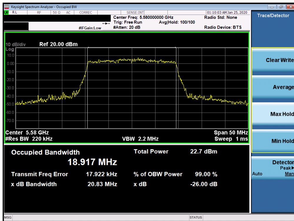
Plot 7-59. 26dB Bandwidth Plot SISO CORE 0 (20MHz BW 802.11ax– RU242 (UNII Band 2C) – Ch. 116)
