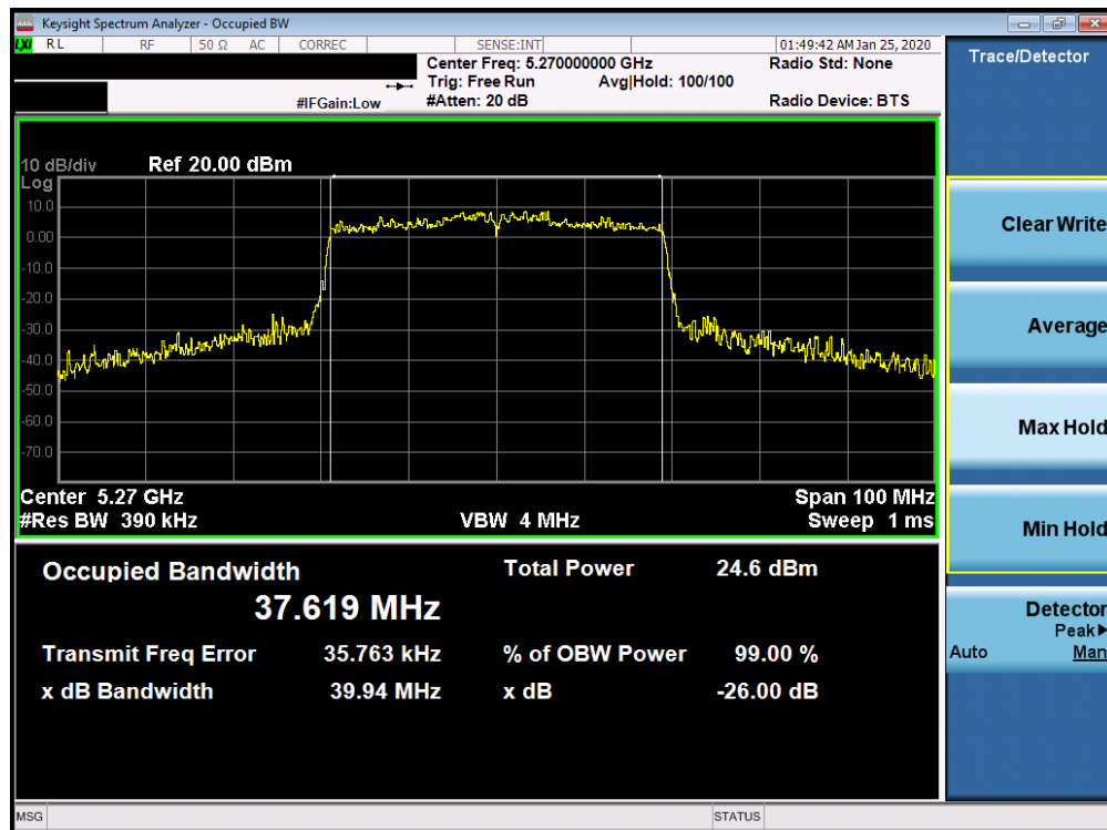
Plot 7-43. 26dB Bandwidth Plot SISO CORE 0 (40MHz BW 802.11ax - RU484 (UNII Band 2A) - Ch. 54)
