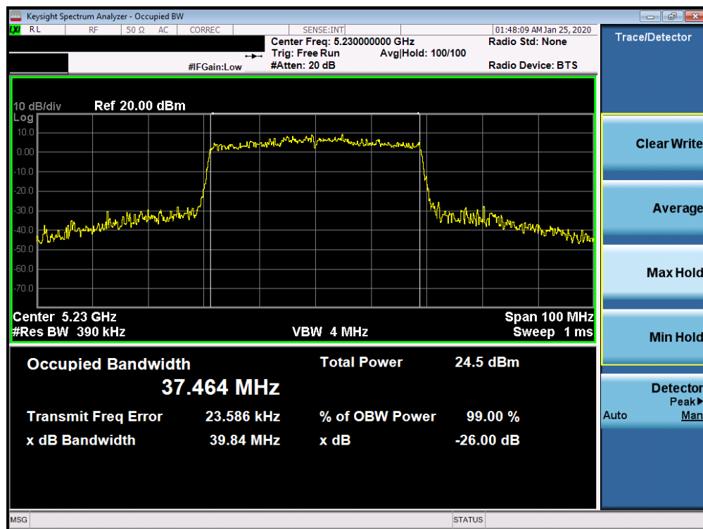
Plot 7-20. 26dB Bandwidth Plot SISO CORE 0 (40MHz BW 802.11ax – RU484 (UNII Band 1) – Ch. 46)
