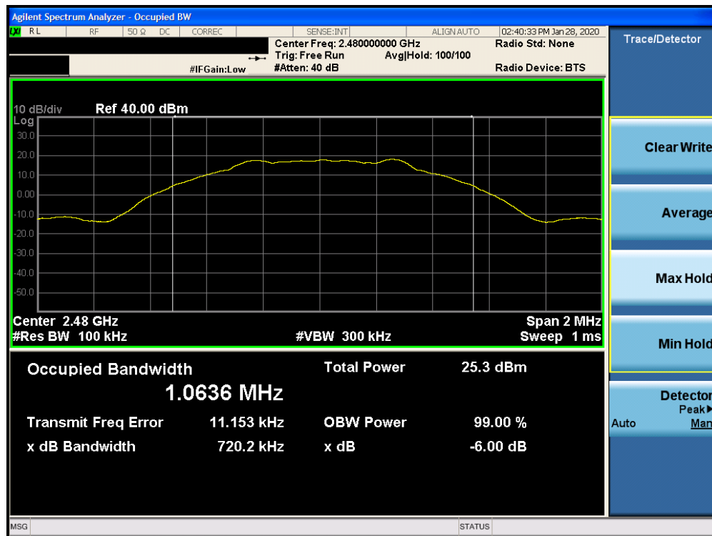
Plot 7-9. 6dB Bandwidth Plot Ant 2a (Bluetooth (LE), 1Mbps, ePA – Ch. 39)
