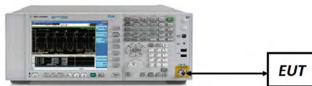
Figure 7-4. Test Instrument & Measurement Setup
