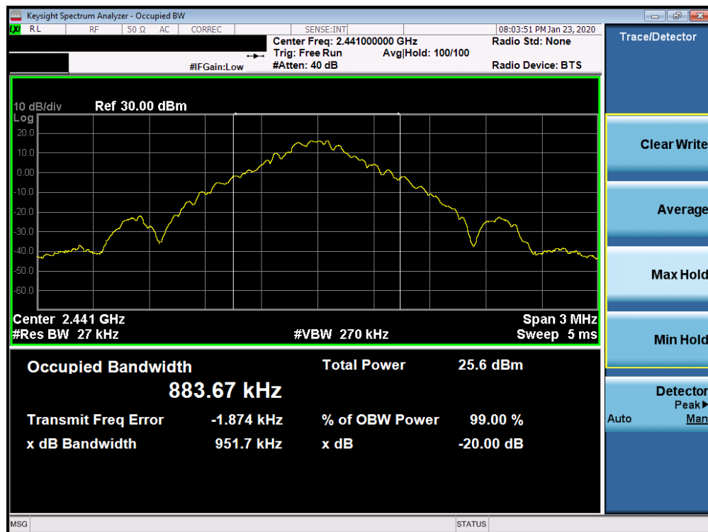
Plot 7-2. 20dB Bandwidth Plot Ant 4a (Bluetooth, GFSK, ePA – Ch. 39)
