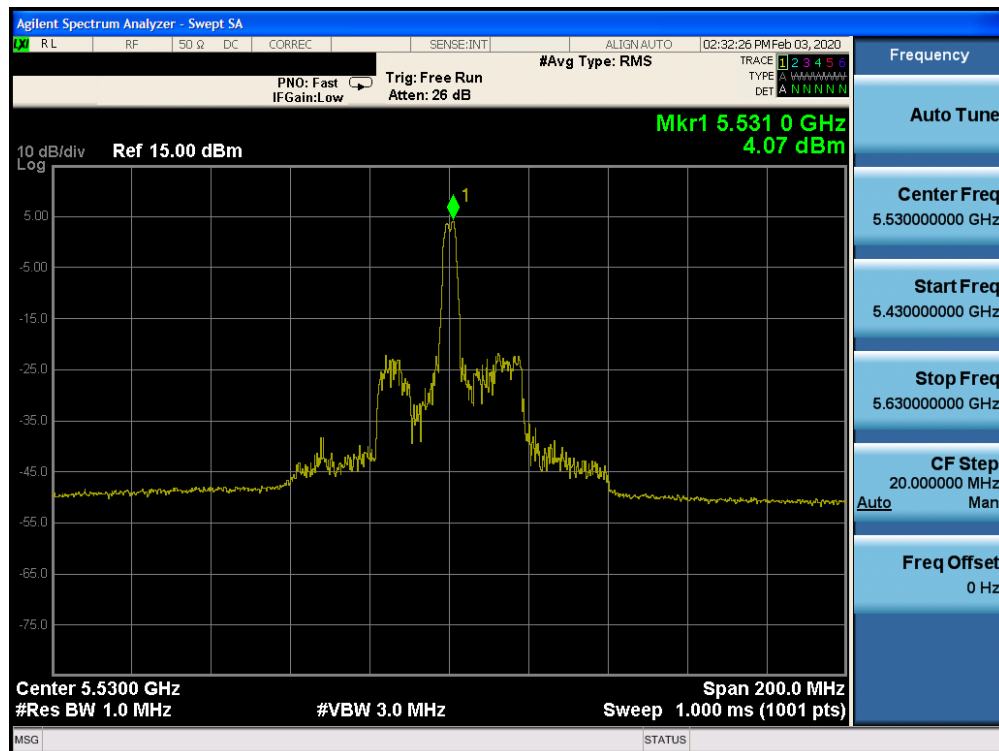
Plot 7-612. Power Spectral Density Plot SDM CORE 1 (80MHz BW 802.11ax Index 18 – RU26 (UNII Band 2C) – Ch. 106)
