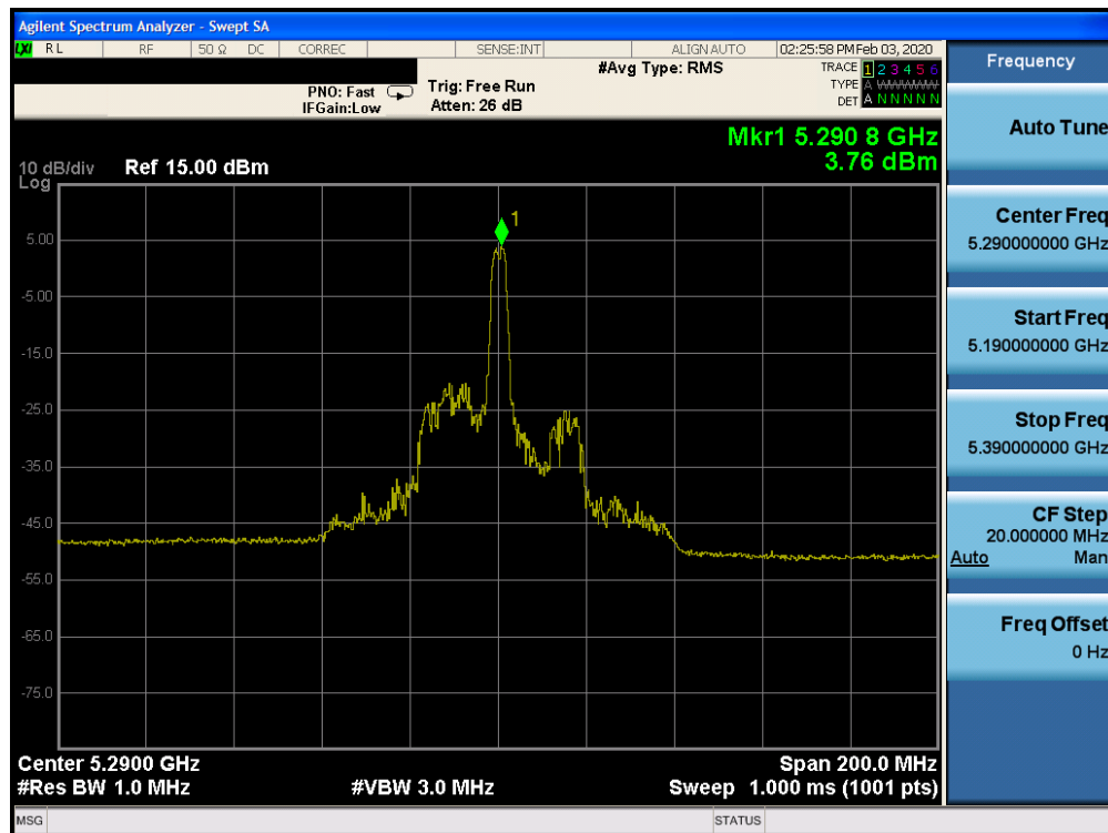
Plot 7-556. Power Spectral Density Plot SDM CORE 1 (80MHz BW 802.11ax Index 18 – RU26 (UNII Band 2A) – Ch. 58)
