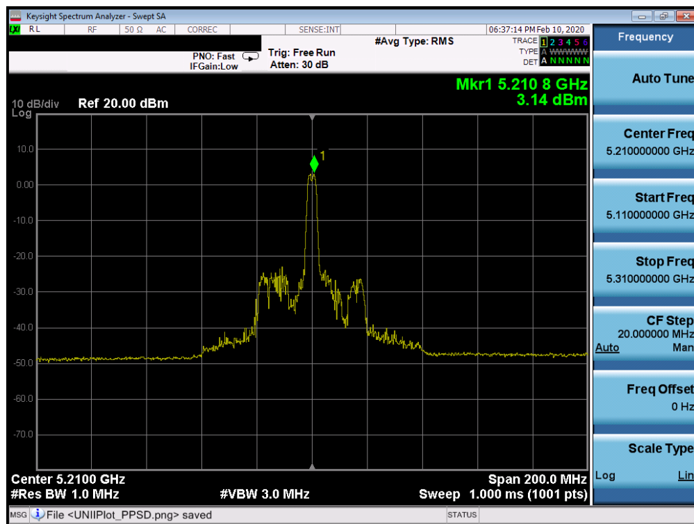
Plot 7-462. Power Spectral Density ISED Plot SISO CORE 1 (80MHz BW 802.11ax Index 18 – RU26 (UNII Band 1) – Ch. 42)
