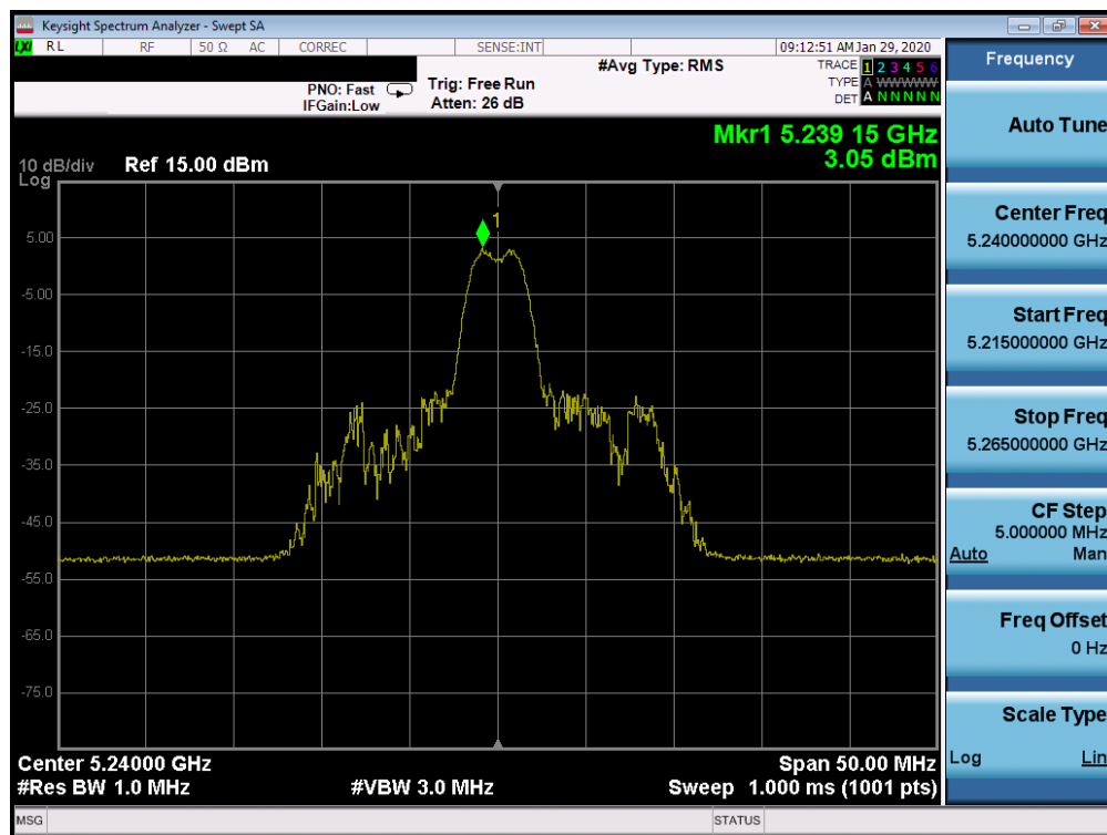
Plot 7-448. Power Spectral Density ISED Plot SISO CORE 1 (20MHz BW 802.11ax Index 4 – RU26 (UNII Band 1) – Ch. 48)
