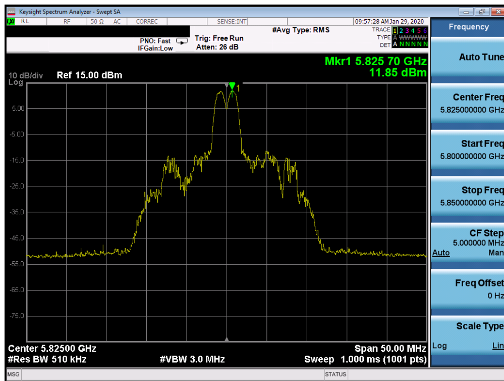
Plot 7-424. Power Spectral Density Plot SISO CORE 1 (20MHz BW 802.11ax Index 4 – RU26 (UNII Band 3) – Ch. 165)
