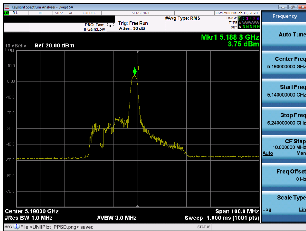
Plot 7-454. Power Spectral Density ISED Plot SISO CORE 1 (40MHz BW 802.11ax Index 8 – RU26 (UNII Band 1) – Ch. 38)
