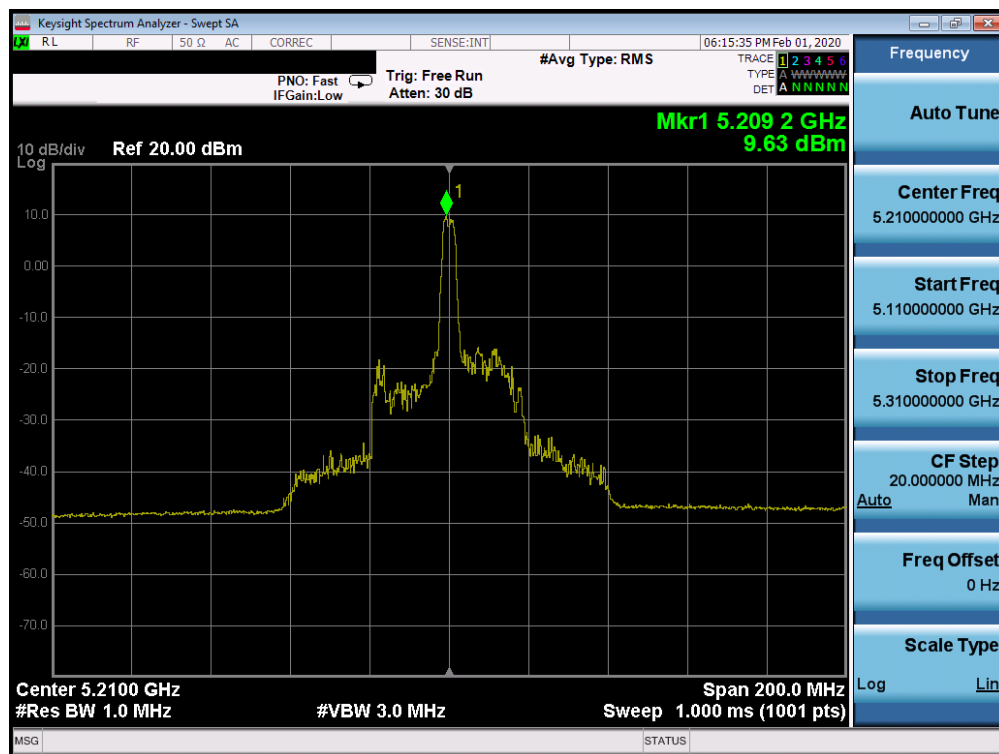
Plot 7-358. Power Spectral Density Plot SISO CORE 1 (80MHz BW 802.11ax Index 18 – RU26 (UNII Band 1) – Ch. 42)
