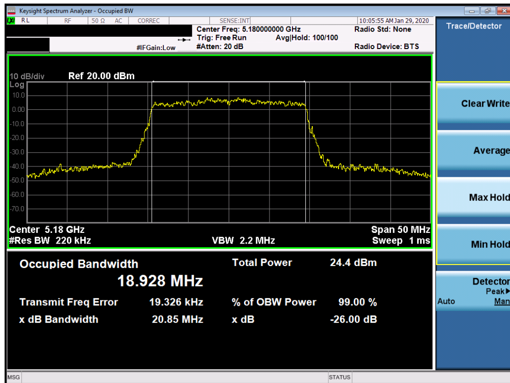
Plot 7-90. 26dB Bandwidth Plot SISO CORE 1 (20MHz BW 802.11ax– RU242 (UNII Band 1) – Ch. 36)
