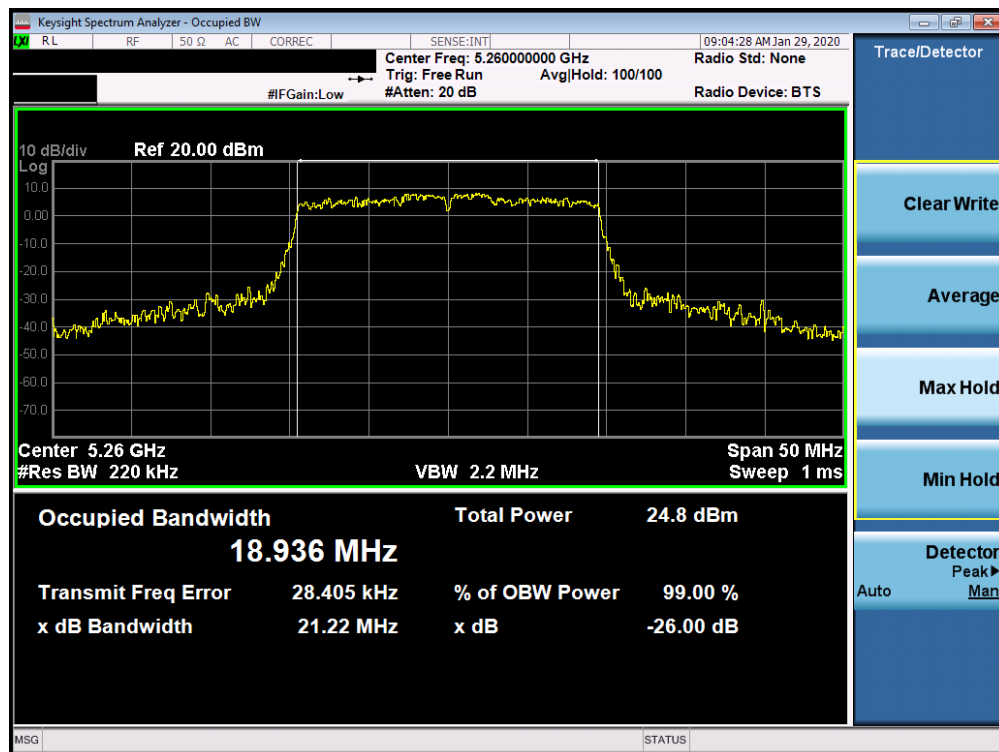
Plot 7-34. 26dB Bandwidth Plot SISO CORE 0 (20MHz BW 802.11ax – RU242 (UNII Band 2A) – Ch. 52)
