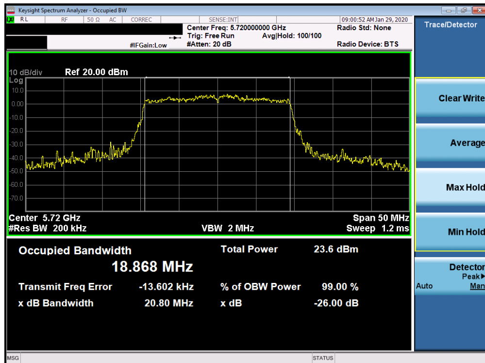
Plot 7-60. 26dB Bandwidth Plot SISO CORE 0 (20MHz BW 802.11ax– RU242 (UNII Band 2C) – Ch. 144)
