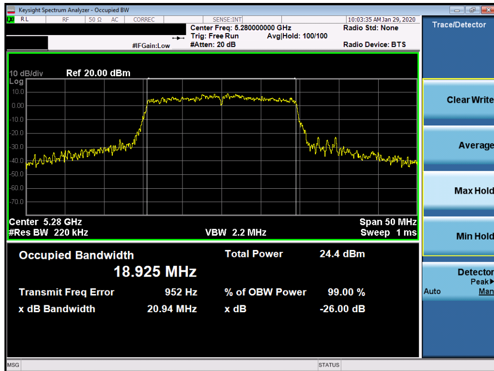
Plot 7-115. 26dB Bandwidth Plot SISO CORE 1 (20MHz BW 802.11ax- RU242 (UNII Band 2A) – Ch. 56)
