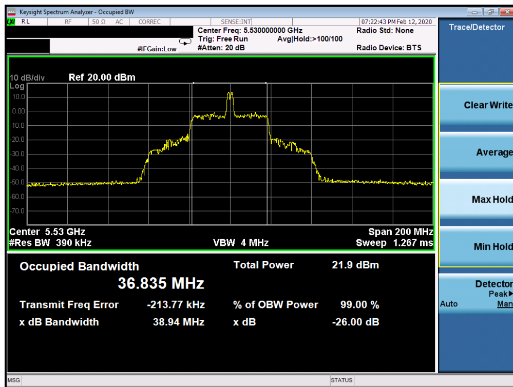
Plot 7-74. 26dB Bandwidth Plot SISO CORE 0 (80MHz BW 802.11ax Index 18 – RU26 (UNII Band 2C) – Ch. 106)
