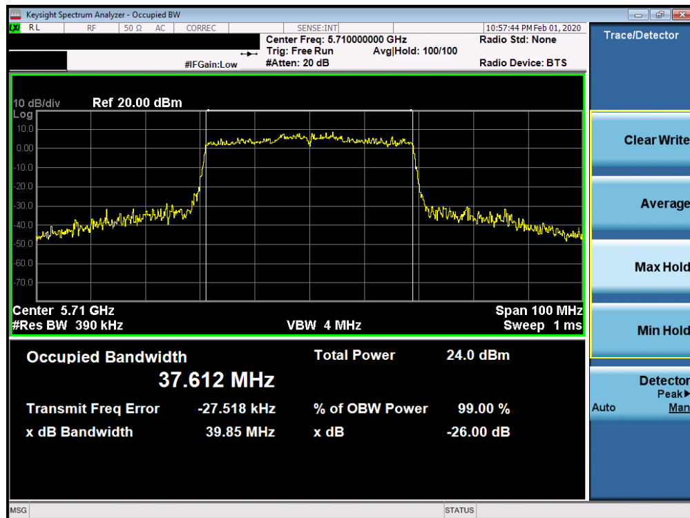
Plot 7-72. 26dB Bandwidth Plot SISO CORE 0 (40MHz BW 802.11ax – RU484 (UNII Band 2C) – Ch. 142)
