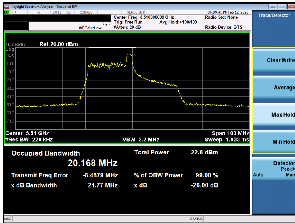
Plot 7-62. 26dB Bandwidth Plot SISO CORE 0 (40MHz BW 802.11ax Index 8 – RU26 (UNII Band 2C) – Ch. 102)
