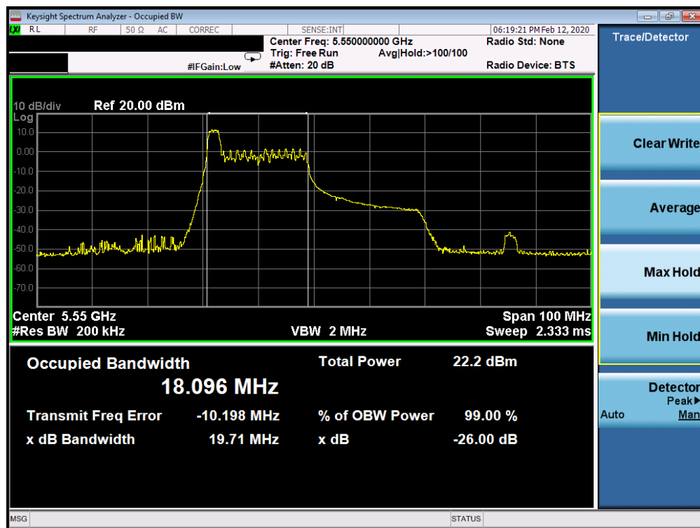
Plot 7-64. 26dB Bandwidth Plot SISO CORE 0 (40MHz BW 802.11ax Index 0 – RU26 (UNII Band 2C) – Ch. 110)
