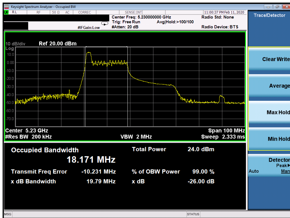
Plot 7-96. 26dB Bandwidth Plot SISO CORE 1 (40MHz BW 802.11ax Index 0 – RU26 (UNII Band 1) – Ch. 46)
