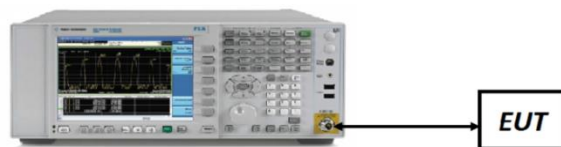
Figure 7-5. Test Instrument & Measurement Setup
