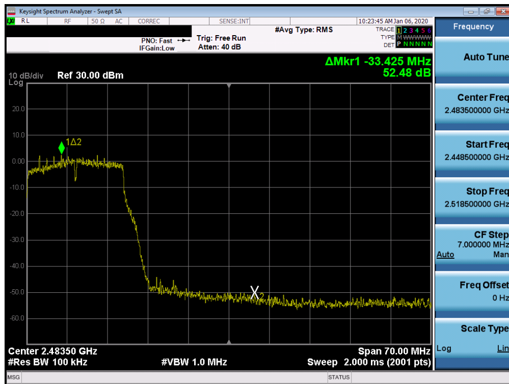
Plot 7-56. Band Edge Plot SISO CORE0 (802.11g - Ch. 10)
