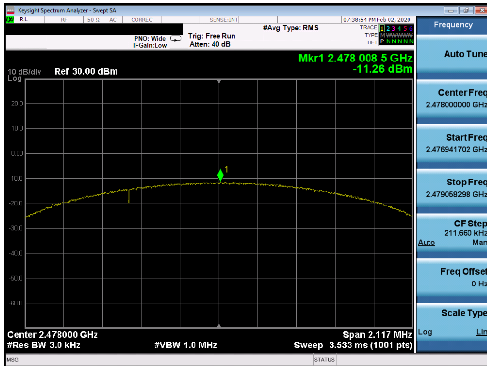
Plot 7-59. Power Spectral Density Plot Tx BF Ant WF8 (Bluetooth (LE), 2Mbps, iPA – Ch. 38)
