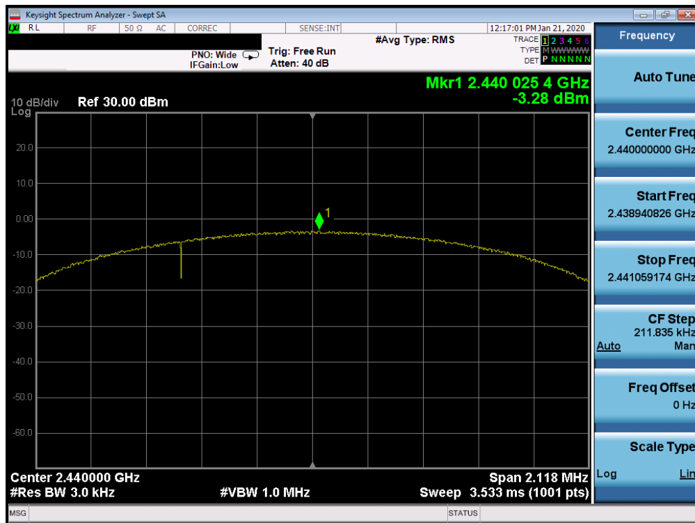
Plot 7-35. Power Spectral Density Plot Ant WF7 (Bluetooth (LE), 2Mbps, iPA – Ch. 19)
