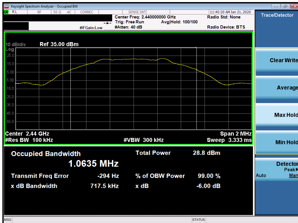
Plot 7-2. 6dB Bandwidth Plot Ant WF8 (Bluetooth (LE), 1Mbps, ePA – Ch. 19)
