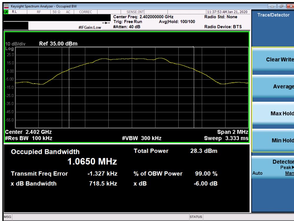
Plot 7-1. 6dB Bandwidth Plot Ant WF8 (Bluetooth (LE), 1Mbps, ePA – Ch. 0)
