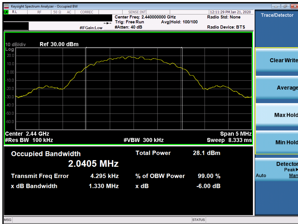
Plot 7-11. 6dB Bandwidth Plot Ant WF7 (Bluetooth (LE), 2Mbps, ePA – Ch. 19)
