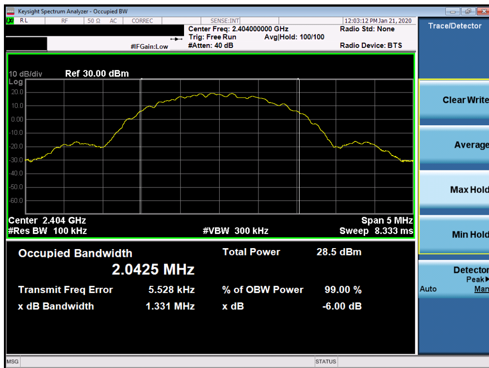
Plot 7-4. 6dB Bandwidth Plot Ant WF8 (Bluetooth (LE), 2Mbps, ePA – Ch. 1)
