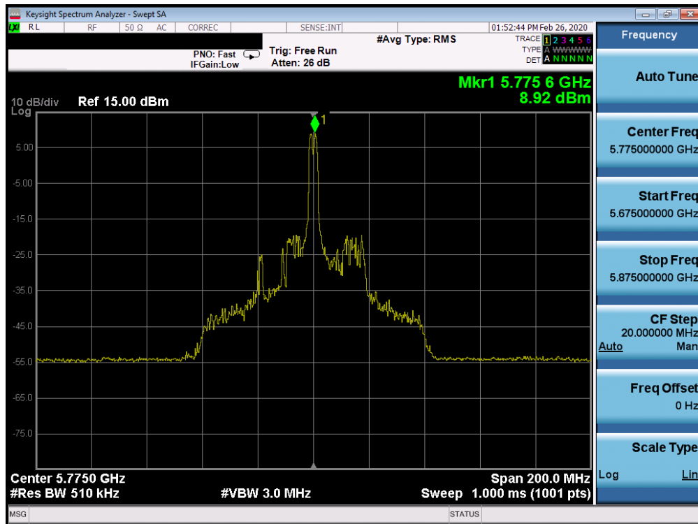
Plot 7-688. Power Spectral Density Plot CDD CORE 0 (80MHz BW 802.11ax Index 18 – RU26 (UNII Band 3) – Ch. 155)
