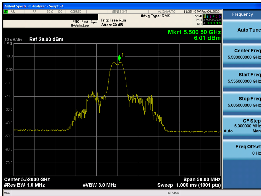
Plot 7-543. Power Spectral Density Plot SDM CORE 1 (20MHz BW 802.11ax Index 4 – RU26 (UNII Band 2C) – Ch. 116)
