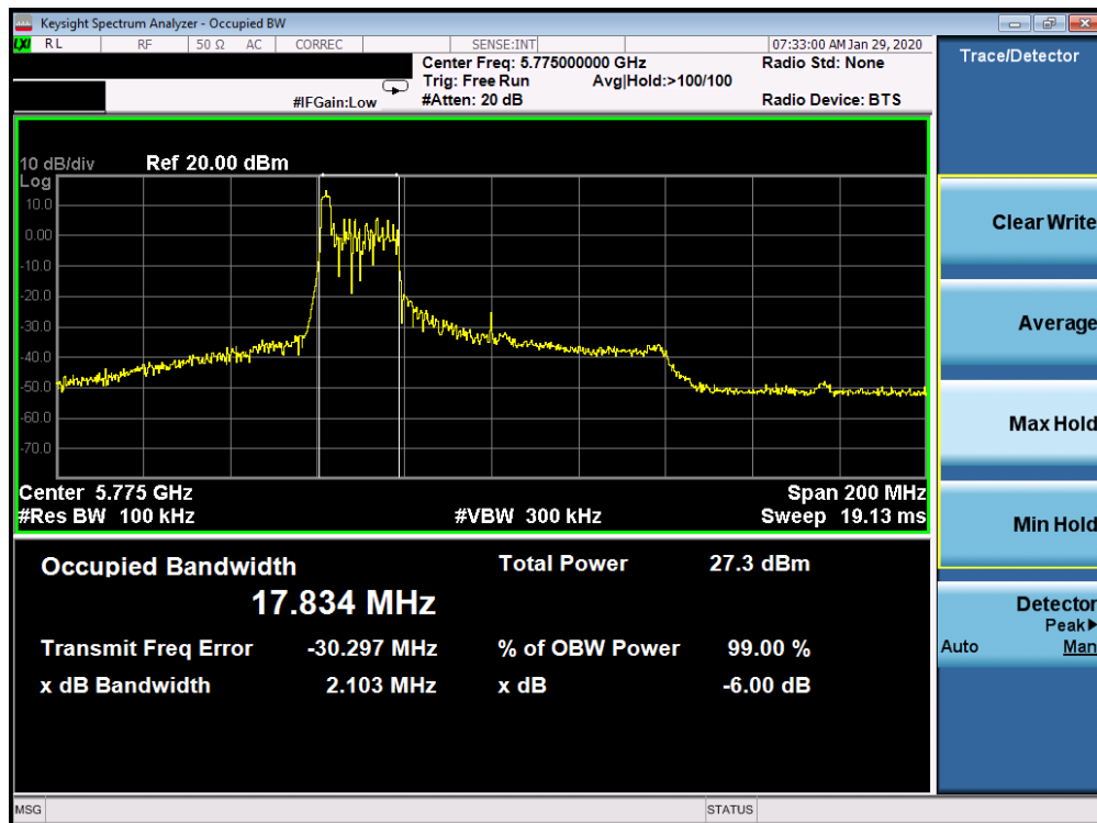
Plot 7-181. 6dB Bandwidth Plot SISO CORE 0 (80MHz BW 802.11ax Index 0 – RU26 (UNII Band 3) – Ch. 155)
