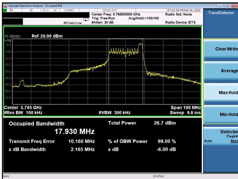
Plot 7-202. 6dB Bandwidth Plot SISO CORE 1 (40MHz BW 802.11ax Index 17 – RU26 (UNII Band 3) – Ch. 159)
