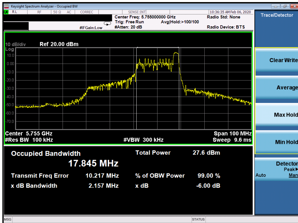
Plot 7-175. 6dB Bandwidth Plot SISO CORE 0 (40MHz BW 802.11ax Index 17 – RU26 (UNII Band 3) – Ch. 151)
