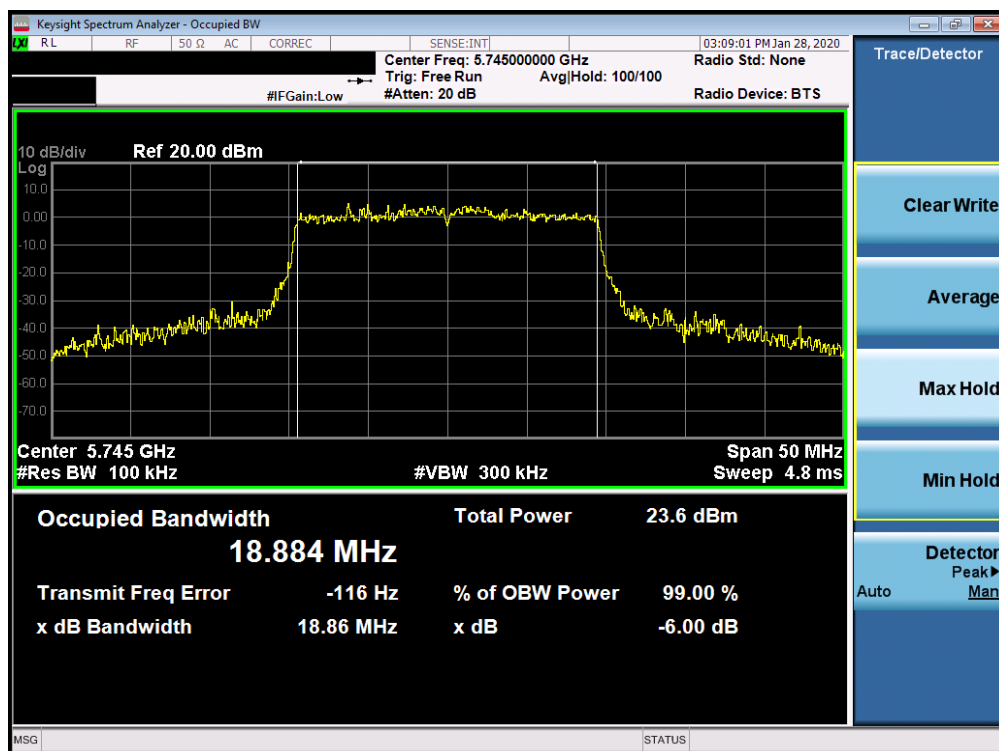
Plot 7-194. 6dB Bandwidth Plot SISO CORE 1 (20MHz BW 802.11ax– RU242 (UNII Band 3) – Ch. 149)
