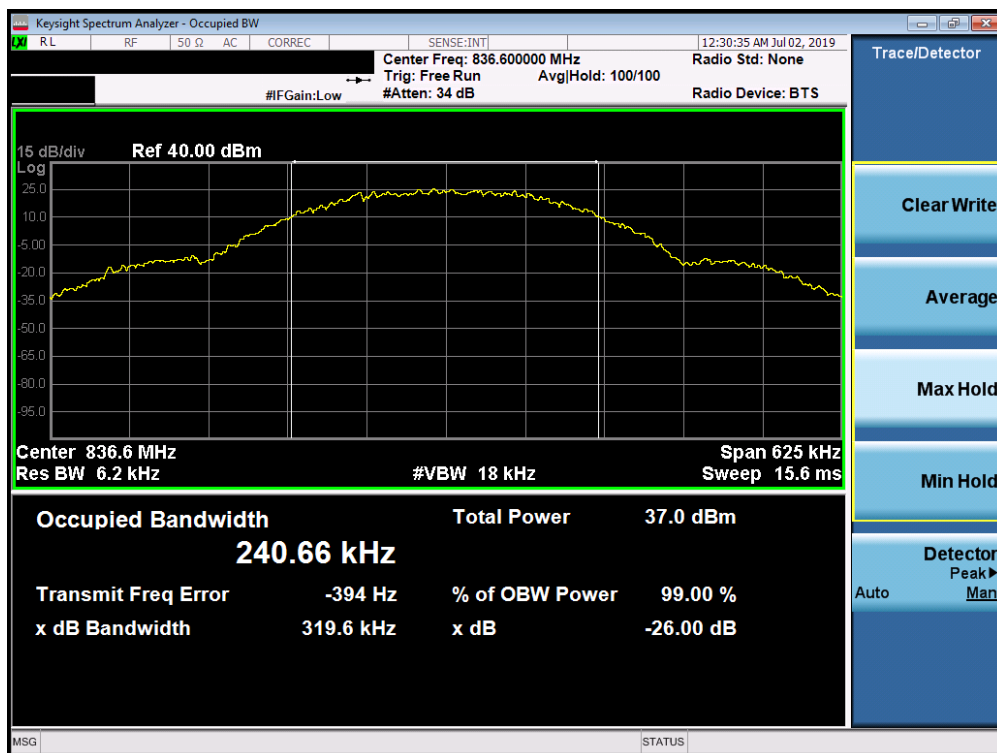
Plot 7-1. Occupied Bandwidth Plot (Cellular GPRS Mode)
