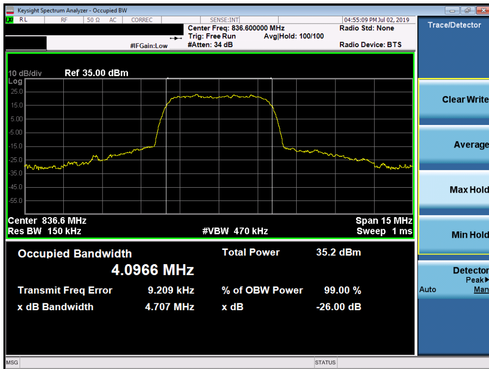
Plot 7-5. Occupied Bandwidth Plot (Cellular WCDMA Mode)
