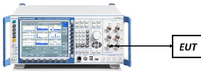
Figure 7-5. ERP/EIRP Measurement Setup
