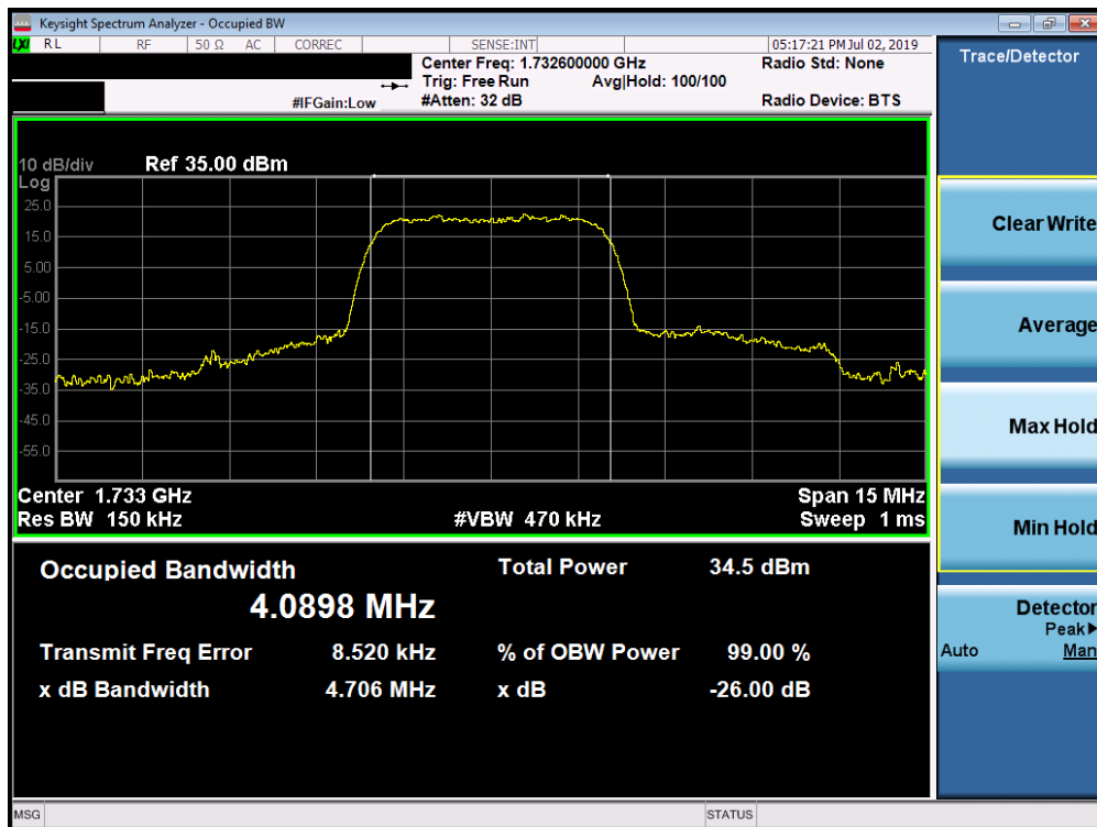
Plot 7-6. Occupied Bandwidth Plot (AWS WCDMA Mode)
