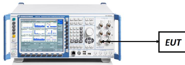
Figure 7-5. Conducted Power Measurement Setup
