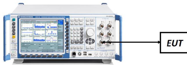
Figure 7-4. Conducted Power Measurement Setup
