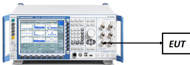
Figure 7-5. ERP/EIRP Measurement Setup
