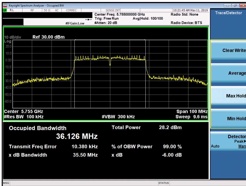
Plot 7-50. 6dB Bandwidth Plot SISO CORE 1 (40MHz BW 802.11n (UNII Band 3) – Ch. 151)
