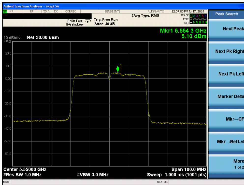
Plot 7-101. Power Spectral Density Plot SISO CORE 1 (40MHz BW 802.11n (UNII Band 2C) – Ch. 110)
