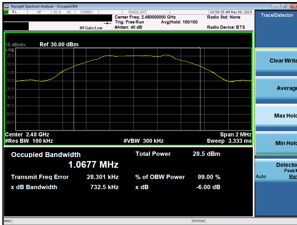
Plot 7-3. 6dB Bandwidth Plot (Bluetooth (LE), ePA – Ch. 39)
