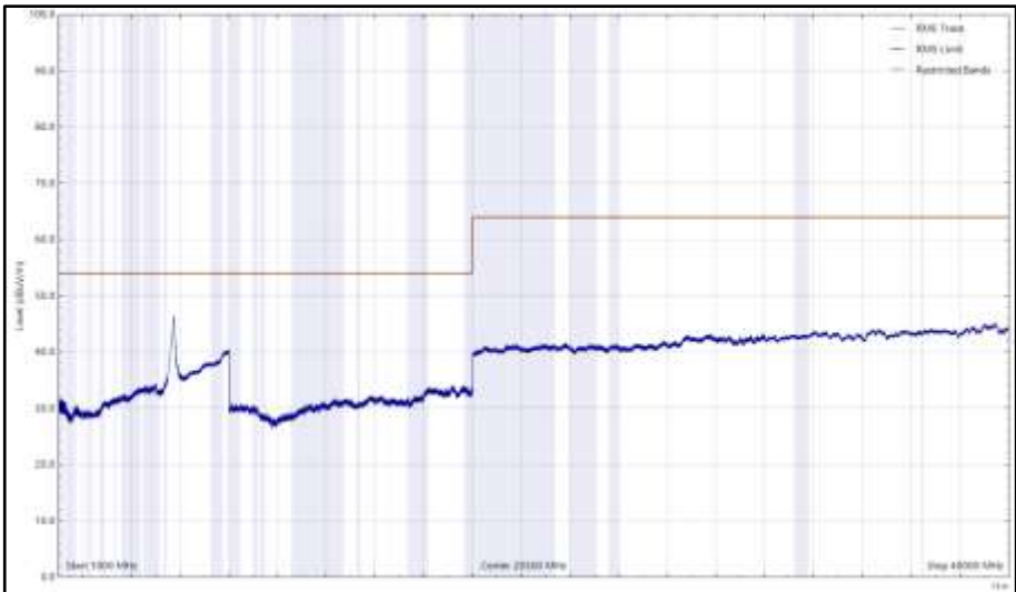
Figure 1002 - U-NII-2C - 5700 MHz (CH140), HT20, CDD, Core 0 + Core 1, 1 GHz to 40 GHz, Horizontal (RMS)
