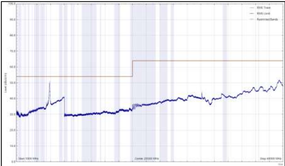
Figure 1014 - U-NII-3 - 5825 MHz (CH165), HT20, CDD, Core 0 + Core 1, 1 GHz to 40 GHz, Vertical (RMS)
