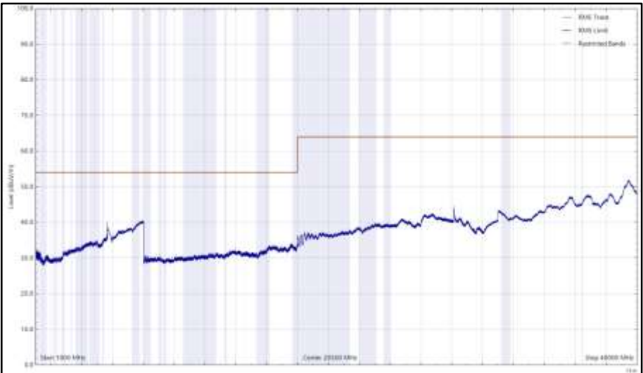
Figure 1024 - 5745 MHz (CH149), HE20, RU26-0, Core 0 + Core 1, 1 GHz to 40 GHz, Vertical (RMS)
