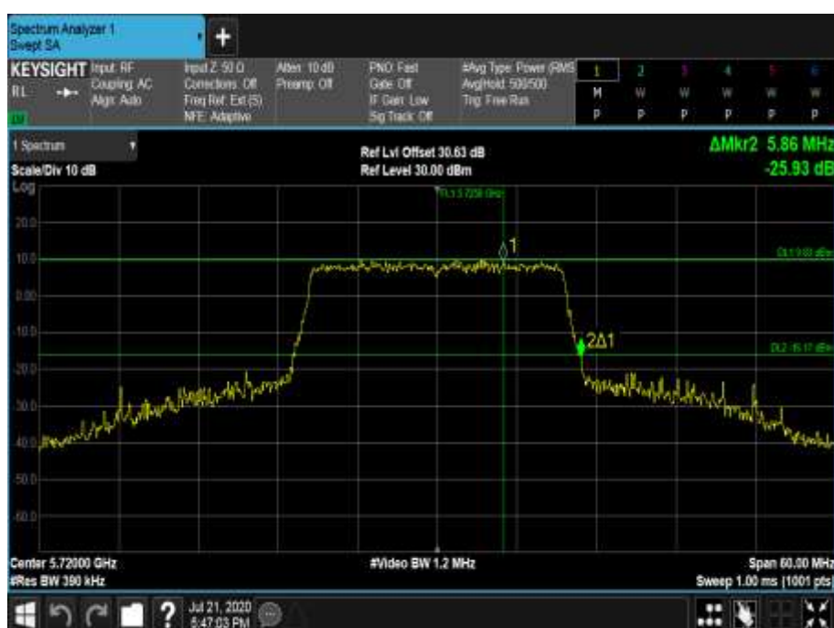
Figure 813 - 5720 MHz - 26 dB Emission Bandwidth
