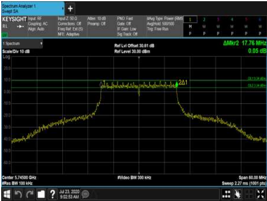
Figure 743 - 5745 MHz - 6 dB DTS Bandwidth
