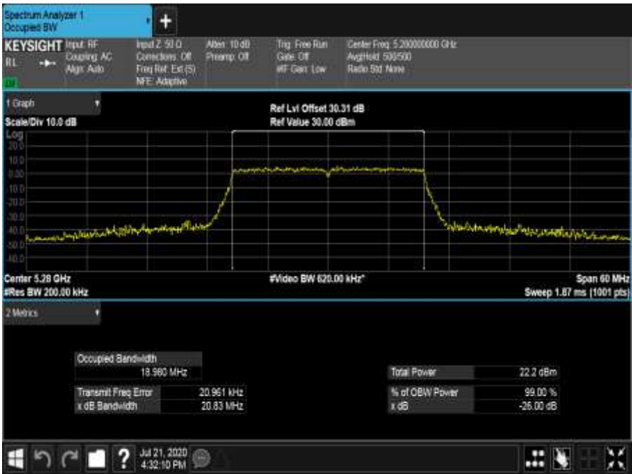
Figure 537 - 5280 MHz - 99% Occupied Bandwidth
