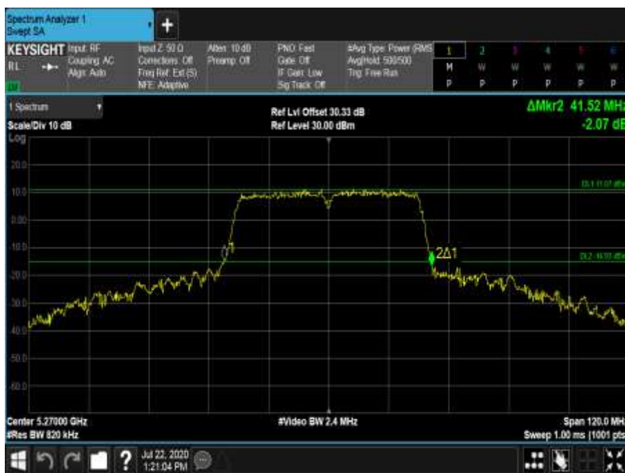
Figure 544 - 5270 MHz - 26 dB Emission Bandwidth
