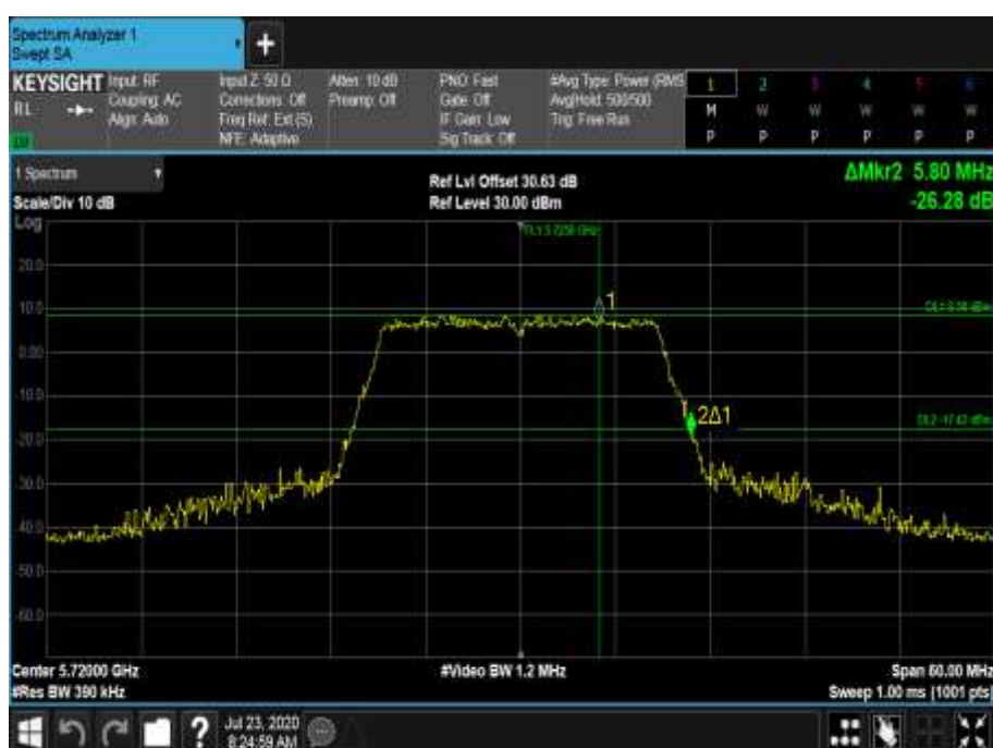
Figure 729 - 5720 MHz - 26 dB Emission Bandwidth
