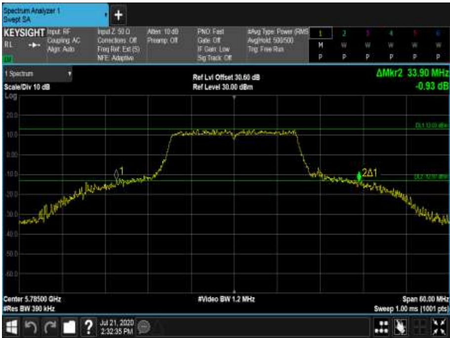
Figure 747 - 5785 MHz - 26 dB Emission Bandwidth
