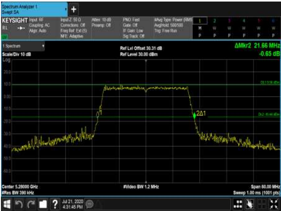
Figure 536 - 5280 MHz - 26 dB Emission Bandwidth
