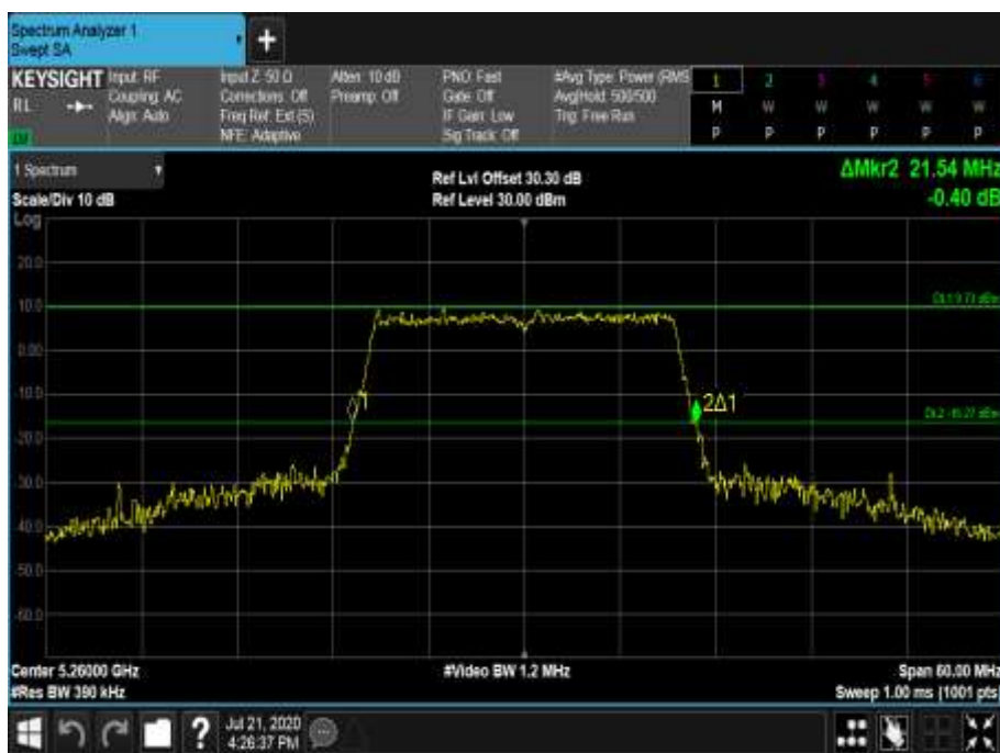
Figure 534 - 5260 MHz - 26 dB Emission Bandwidth
