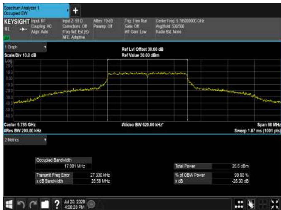
Figure 724 - 5785 MHz - 99% Occupied Bandwidth
