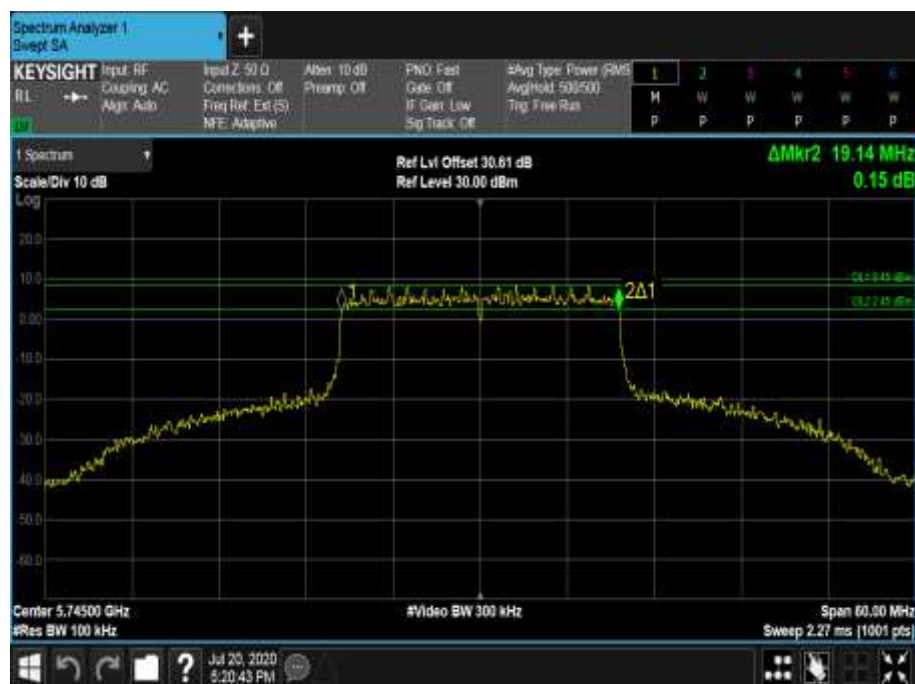
Figure 755 - 5745 MHz - 6 dB DTS Bandwidth
