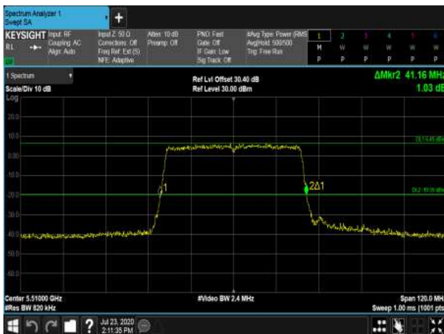
Figure 664 - 5510 MHz - 26 dB Emission Bandwidth
