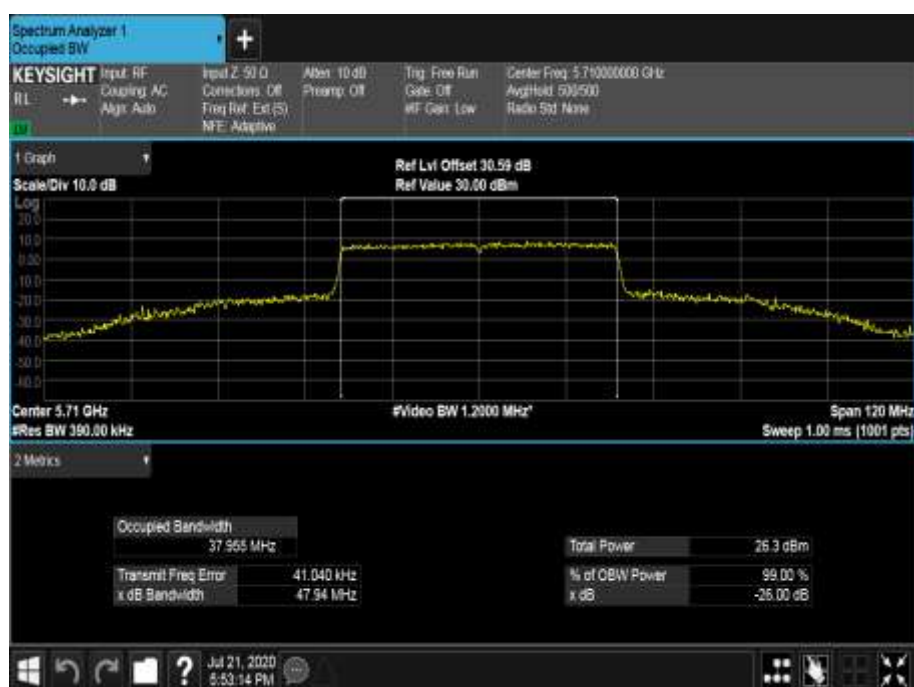
Figure 679 - 5710 MHz - 99% Occupied Bandwidth
