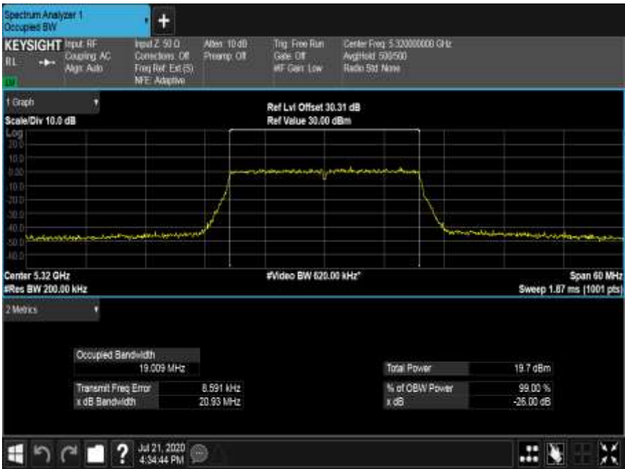
Figure 533 - 5320 MHz - 99% Occupied Bandwidth
