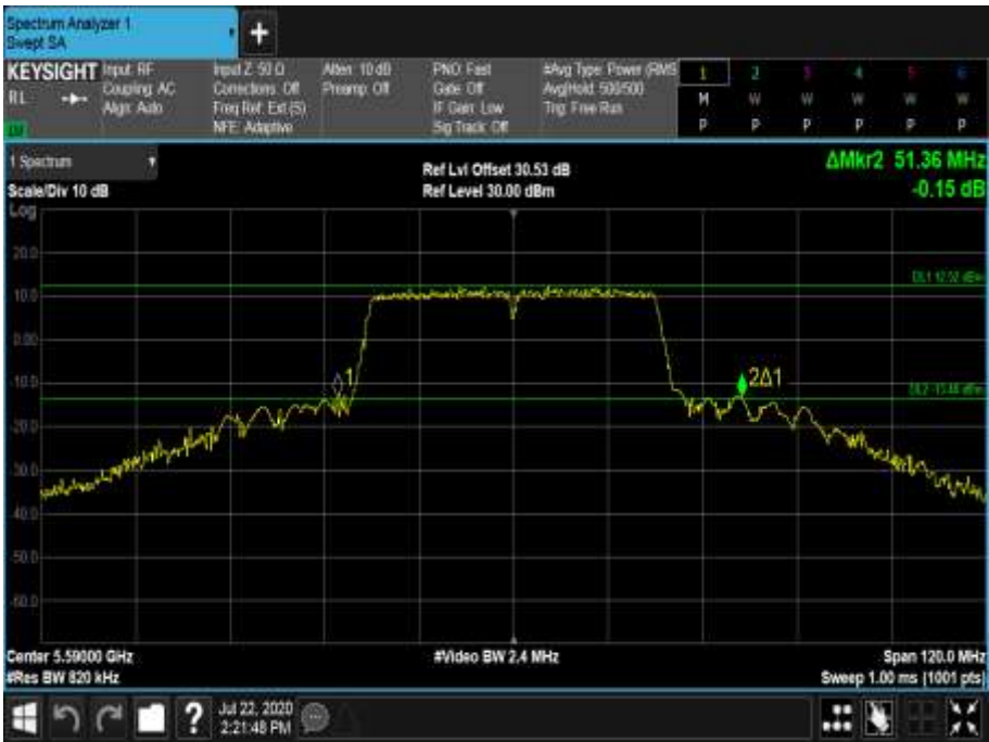
Figure 650 - 5590 MHz - 26 dB Emission Bandwidth
