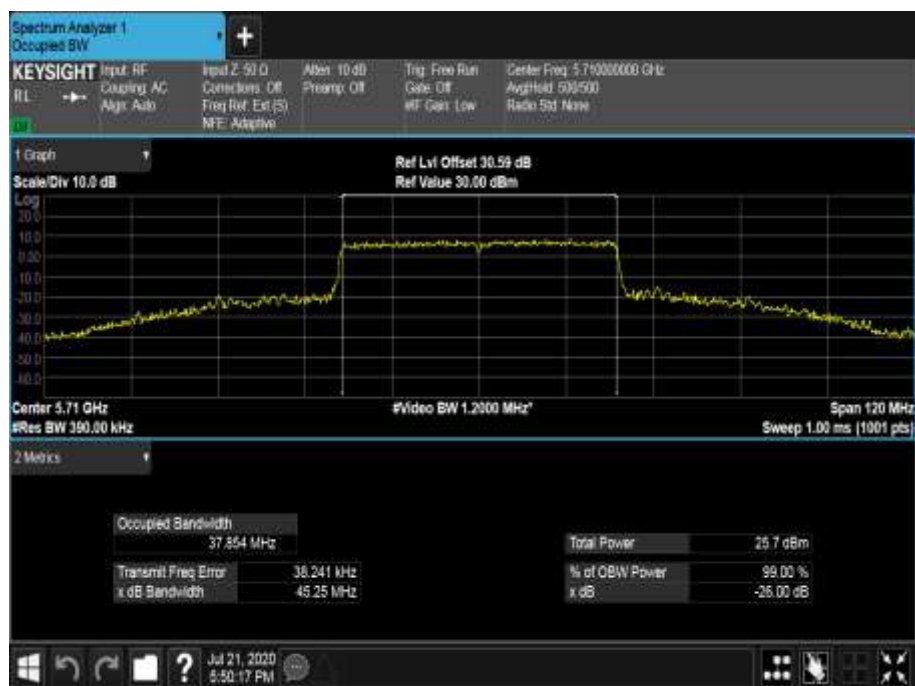
Figure 671 - 5710 MHz - 99% Occupied Bandwidth
