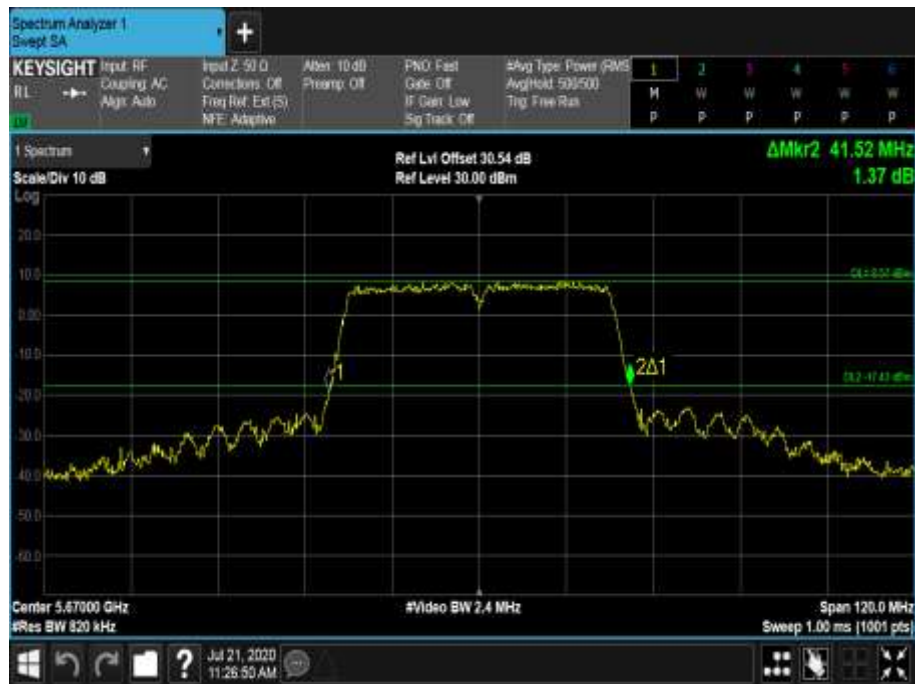
Figure 652 - 5670 MHz - 26 dB Emission Bandwidth
