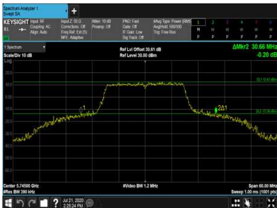
Figure 744 - 5745 MHz - 26 dB Emission Bandwidth
