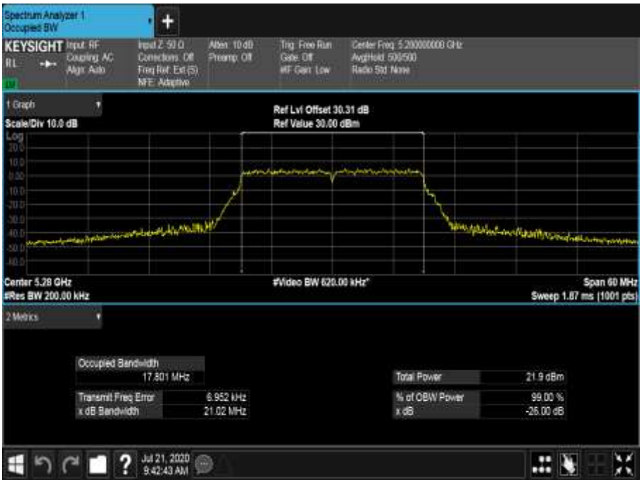
Figure 519 - 5280 MHz - 99% Occupied Bandwidth
