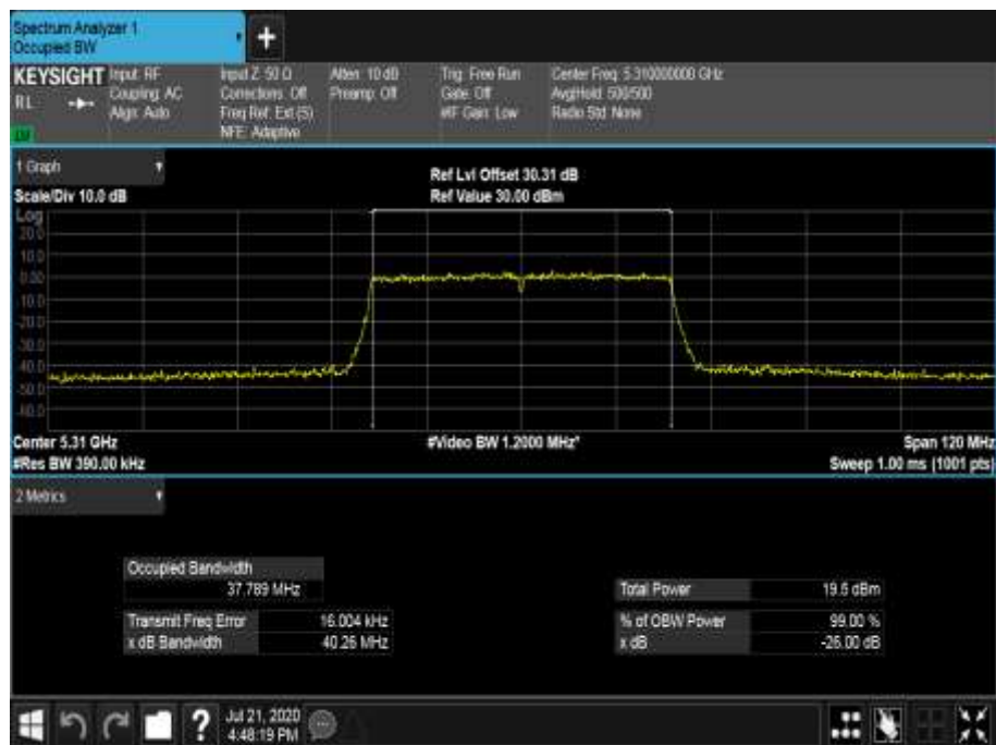
Figure 563 - 5310 MHz - 99% Occupied Bandwidth
