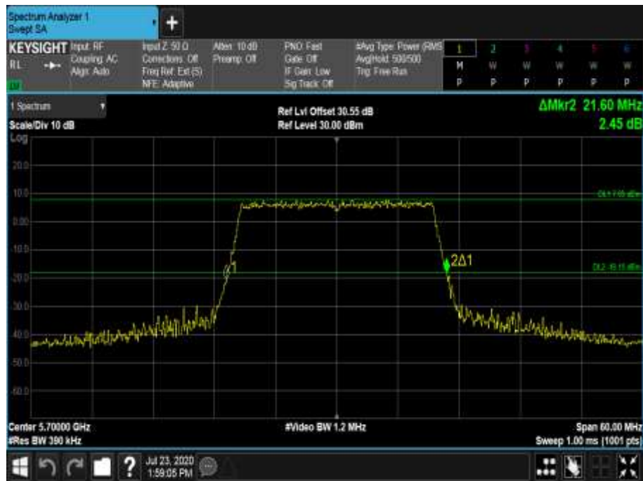
Figure 612 - 5700 MHz - 26 dB Emission Bandwidth
