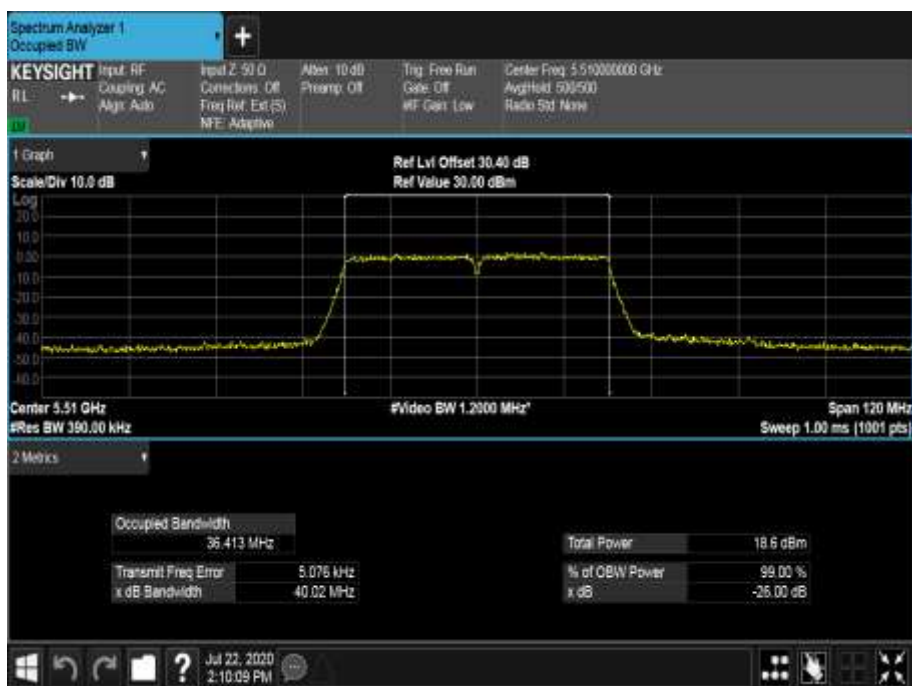
Figure 641 - 5510 MHz - 99% Occupied Bandwidth
