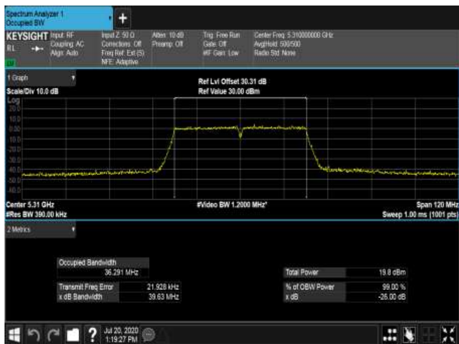
Figure 543 - 5310 MHz - 99% Occupied Bandwidth
