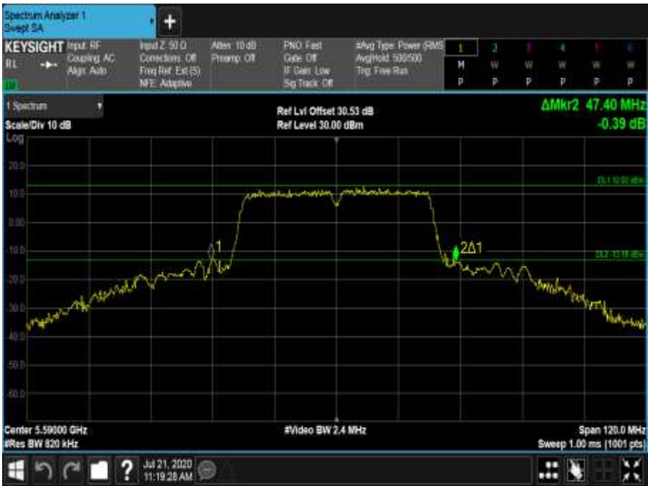
Figure 642 - 5590 MHz - 26 dB Emission Bandwidth
