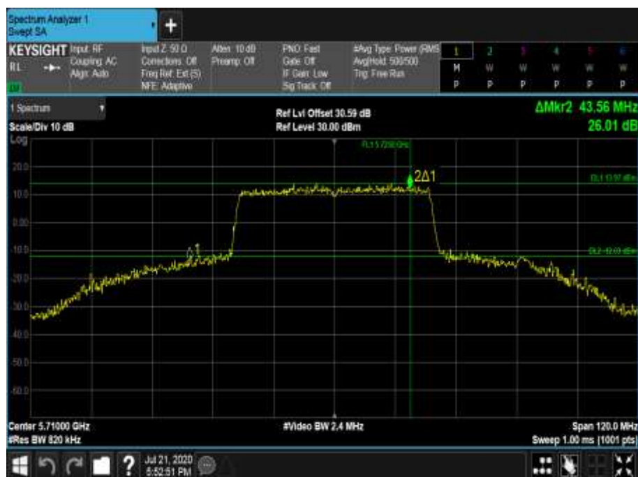
Figure 678 - 5710 MHz - 26 dB Emission Bandwidth
