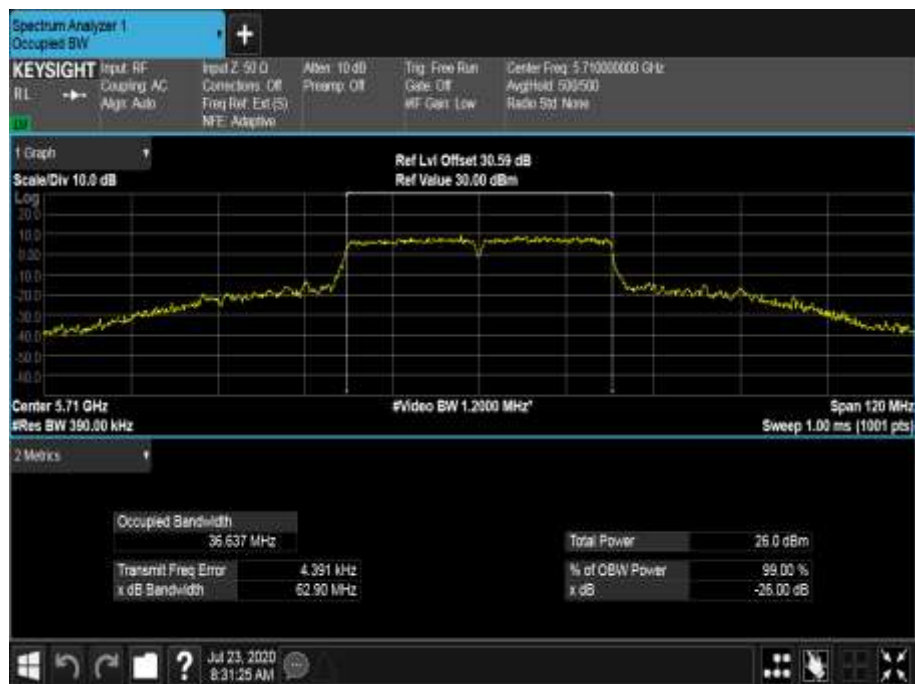
Figure 639 - 5710 MHz - 99% Occupied Bandwidth
