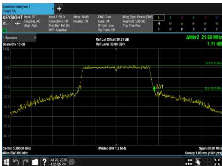
Figure 524 - 5280 MHz - 26 dB Emission Bandwidth
