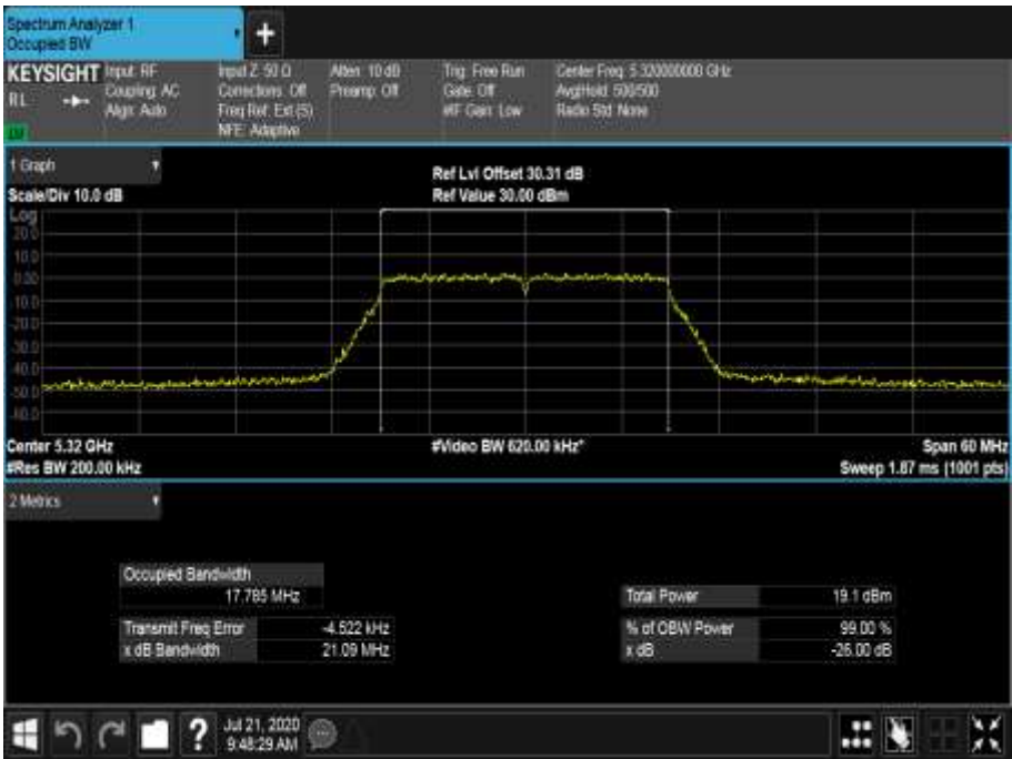
Figure 521 - 5320 MHz - 99% Occupied Bandwidth
