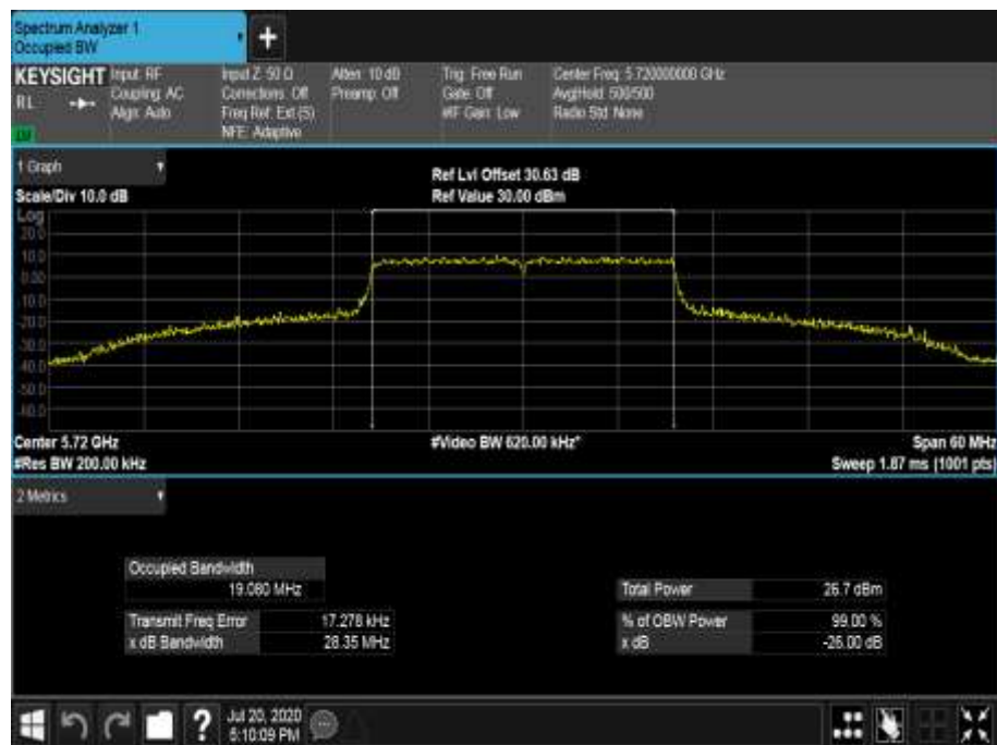
Figure 754 - 5720 MHz - 99% Occupied Bandwidth
