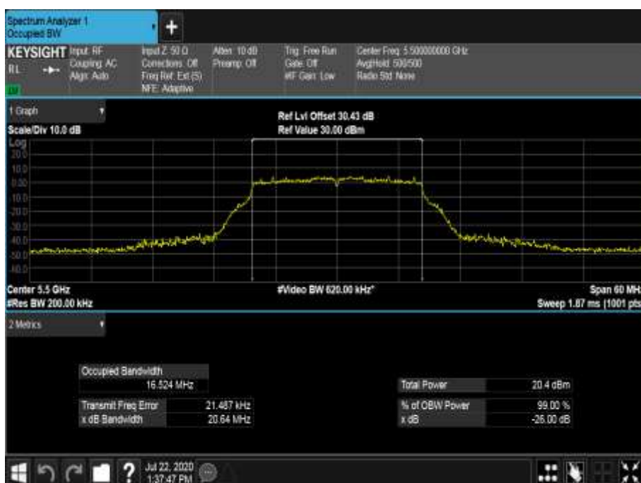
Figure 577 - 5500 MHz - 99% Occupied Bandwidth
