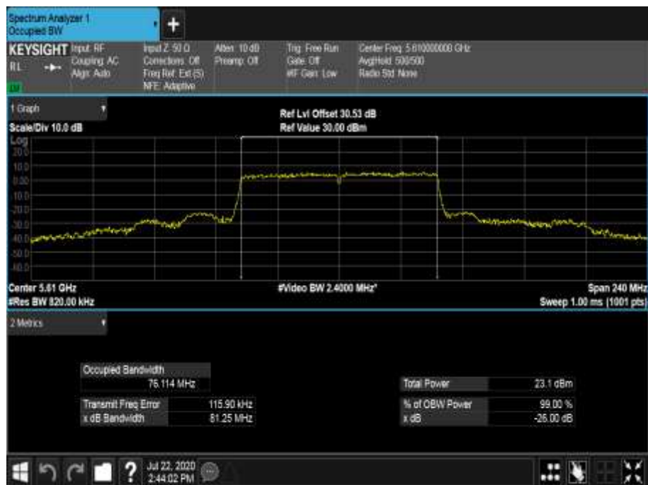
Figure 695 - 5610 MHz - 99% Occupied Bandwidth
