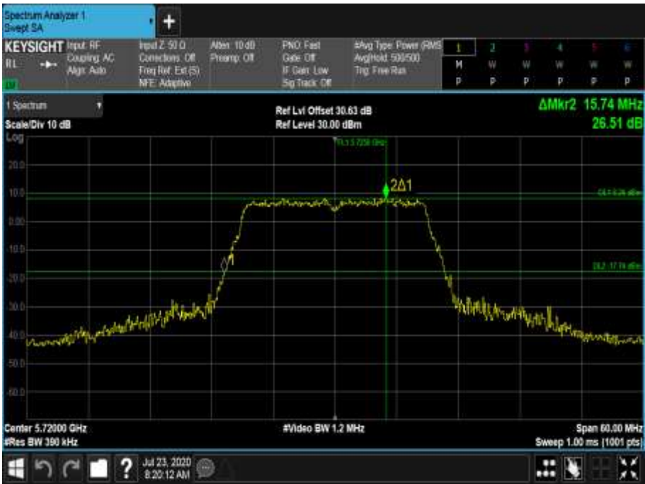
Figure 598 - 5720 MHz - 26 dB Emission Bandwidth
