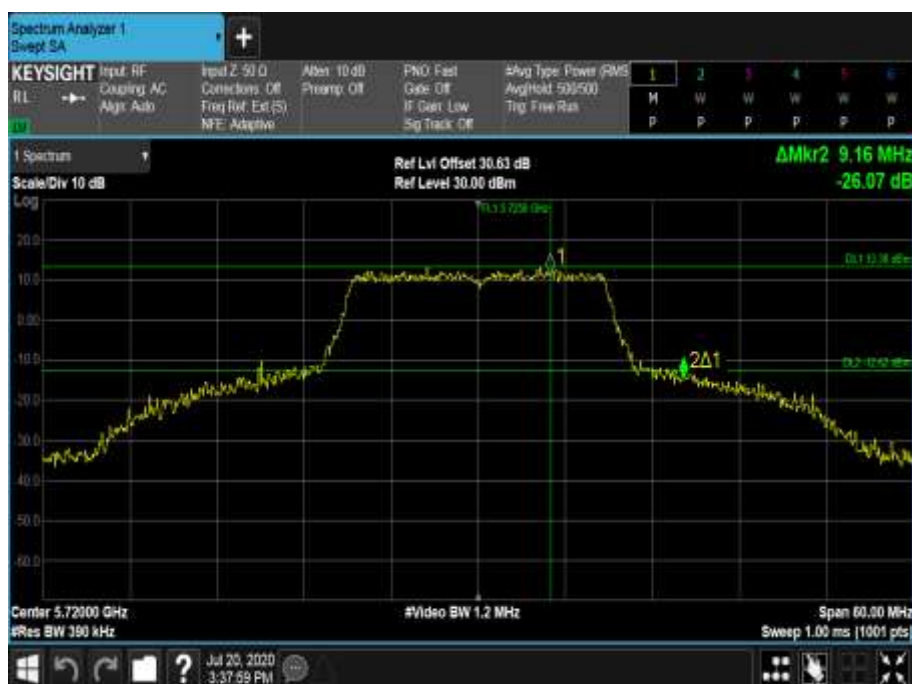
Figure 716 - 5720 MHz - 6 dB DTS Bandwidth
