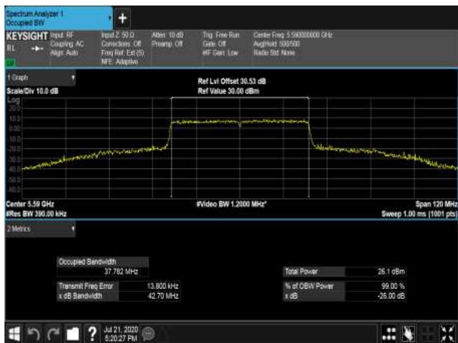
Figure 675 - 5590 MHz - 99% Occupied Bandwidth
