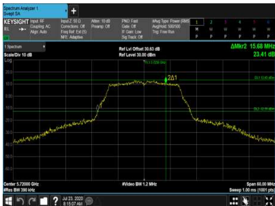
Figure 582 - 5720 MHz - 26 dB Emission Bandwidth
