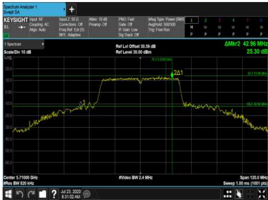
Figure 638 - 5710 MHz - 26 dB Emission Bandwidth
