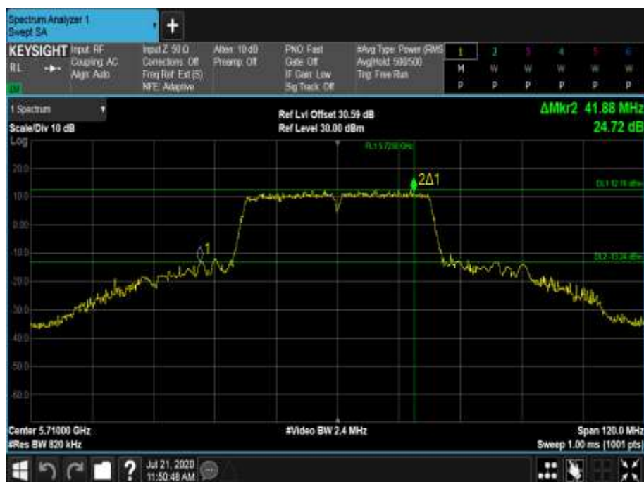
Figure 646 - 5710 MHz - 26 dB Emission Bandwidth
