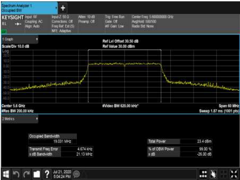
Figure 627 - 5600 MHz - 99% Occupied Bandwidth
