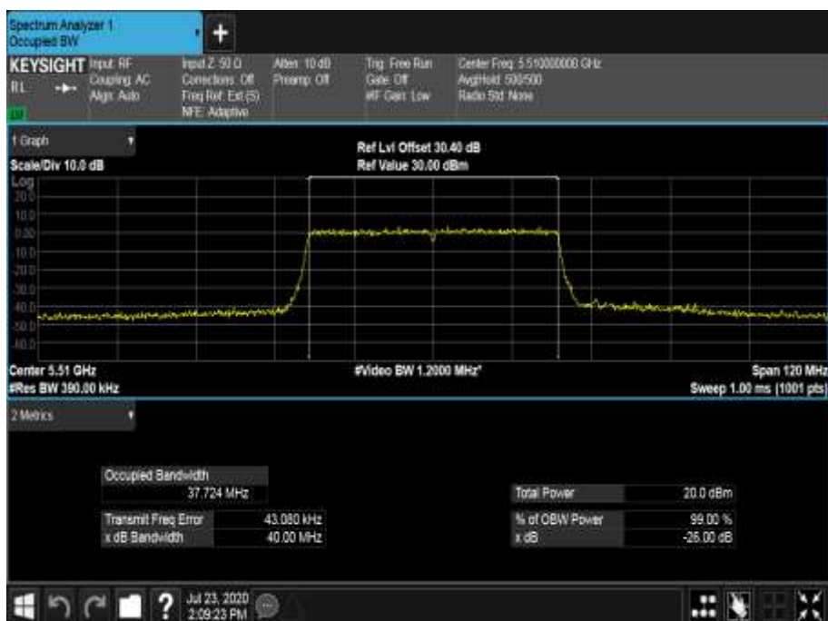
Figure 657 - 5510 MHz - 99% Occupied Bandwidth
