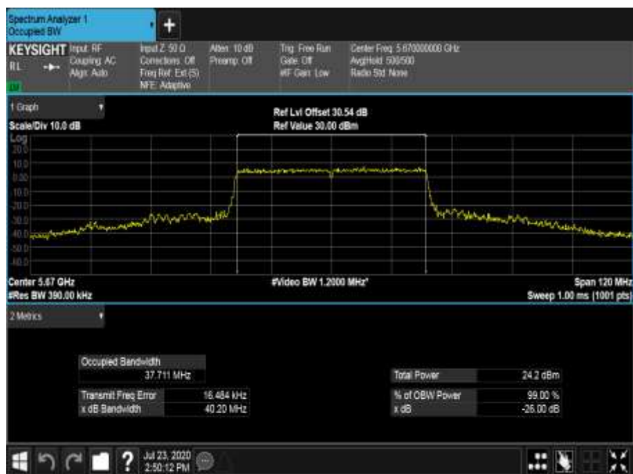
Figure 661 - 5670 MHz - 99% Occupied Bandwidth
