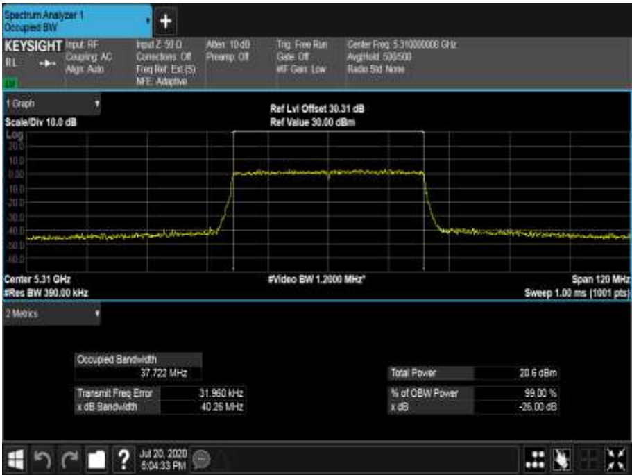
Figure 555 - 5310 MHz - 99% Occupied Bandwidth
