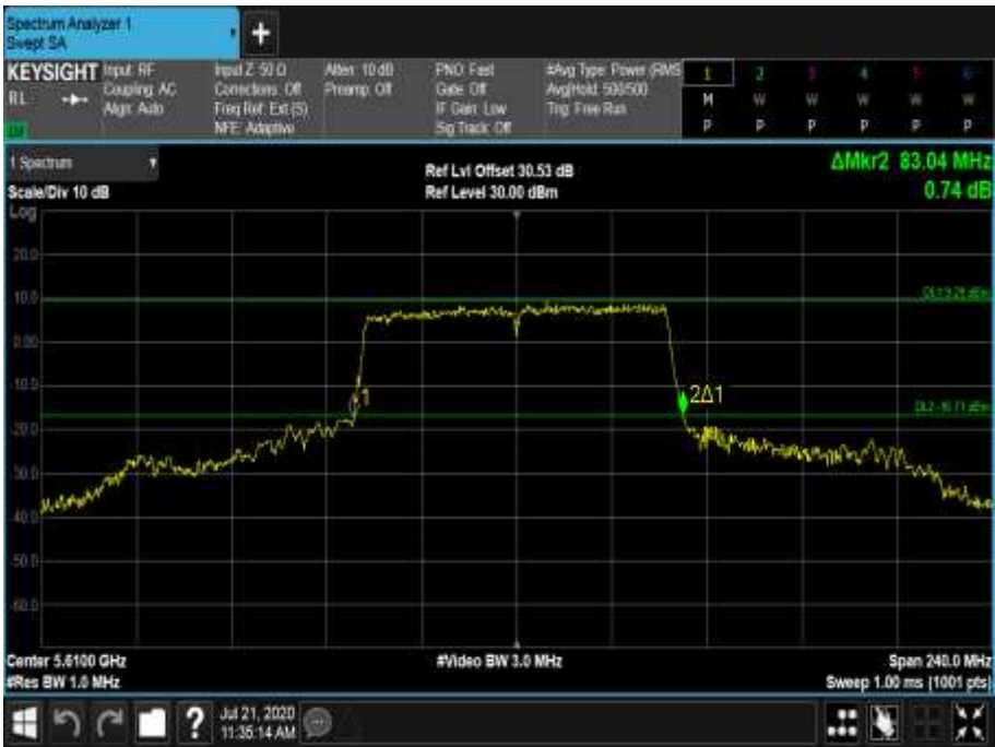
Figure 688 - 5610 MHz - 26 dB Emission Bandwidth
