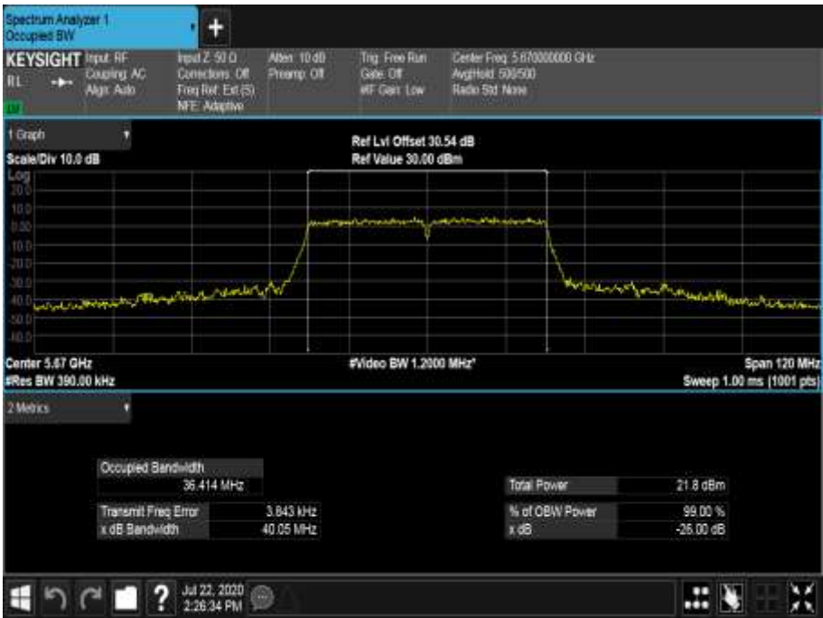
Figure 645 - 5670 MHz - 99% Occupied Bandwidth
