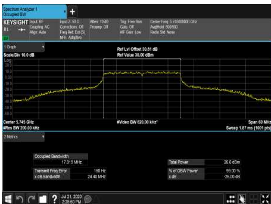
Figure 745 - 5745 MHz - 99% Occupied Bandwidth
