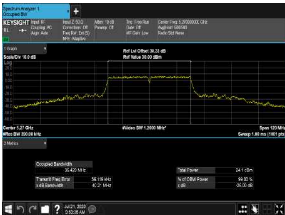
Figure 549 - 5270 MHz - 99% Occupied Bandwidth
