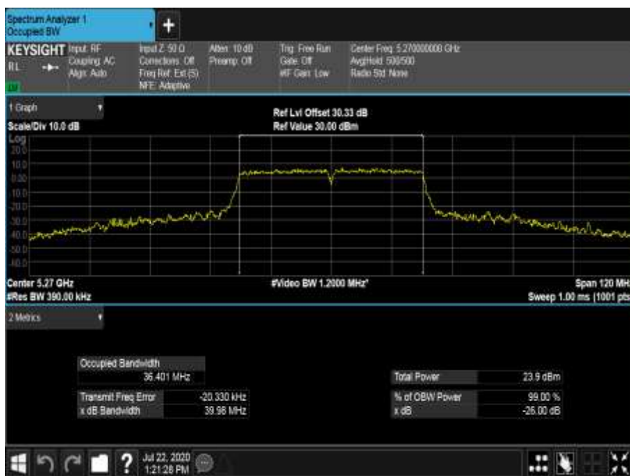
Figure 545 - 5270 MHz - 99% Occupied Bandwidth
