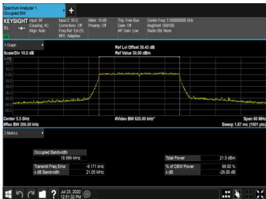
Figure 617 - 5500 MHz - 99% Occupied Bandwidth
