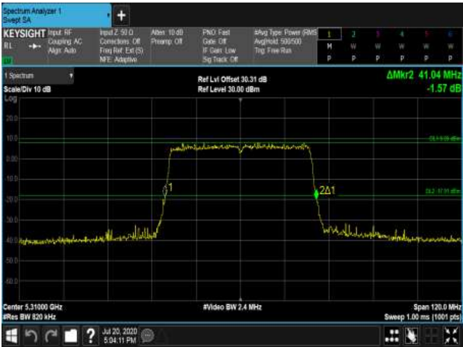
Figure 554 - 5310 MHz - 26 dB Emission Bandwidth
