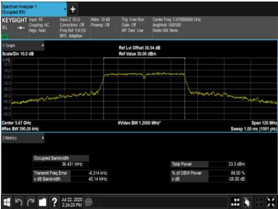
Figure 637 - 5670 MHz - 99% Occupied Bandwidth
