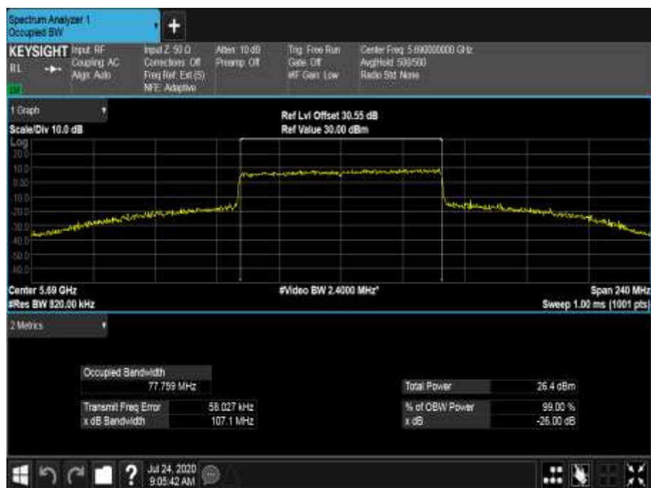
Figure 703 - 5690 MHz - 99% Occupied Bandwidth
