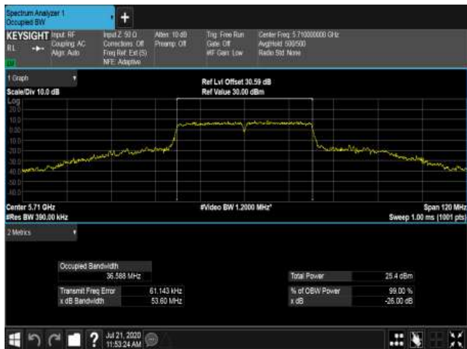
Figure 655 - 5710 MHz - 99% Occupied Bandwidth
