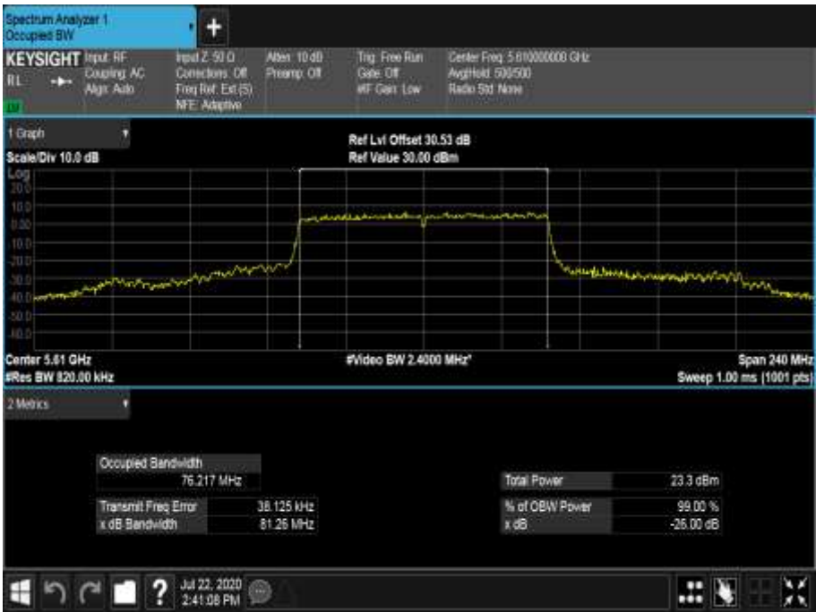
Figure 689 - 5610 MHz - 99% Occupied Bandwidth
