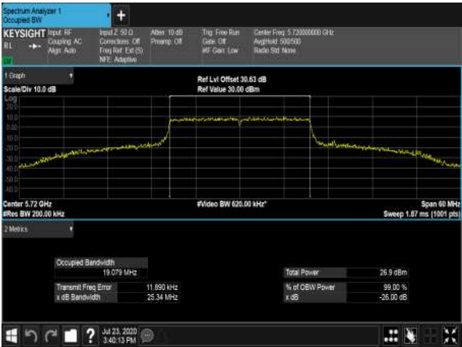
Figure 615 - 5720 MHz - 99% Occupied Bandwidth
