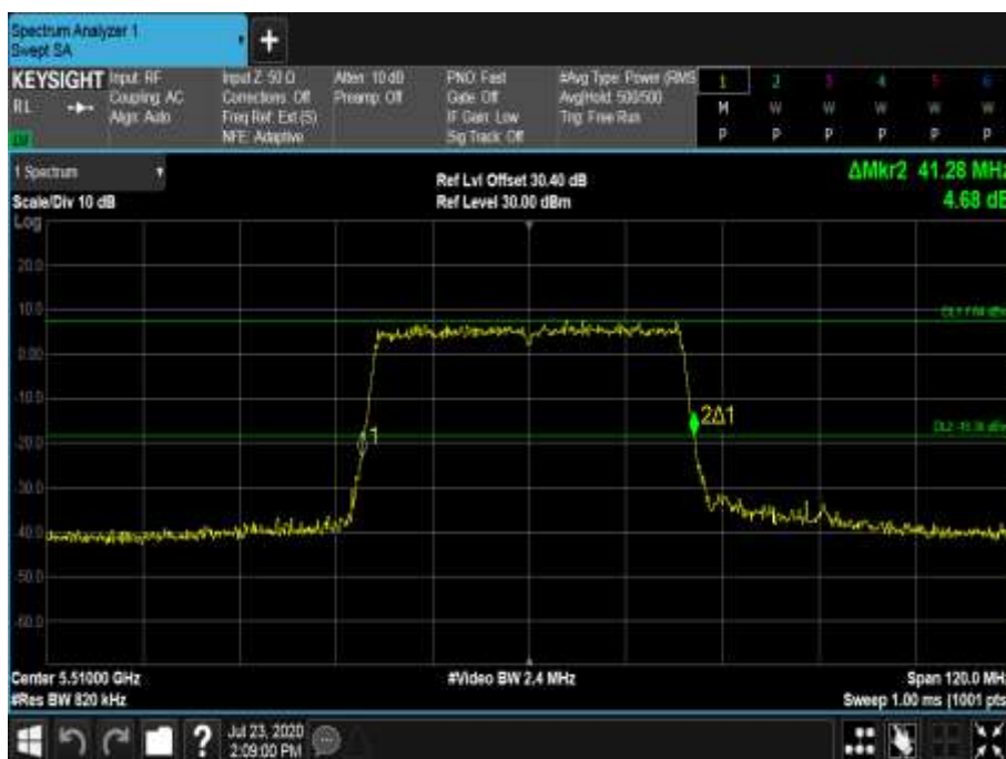
Figure 656 - 5510 MHz - 26 dB Emission Bandwidth
