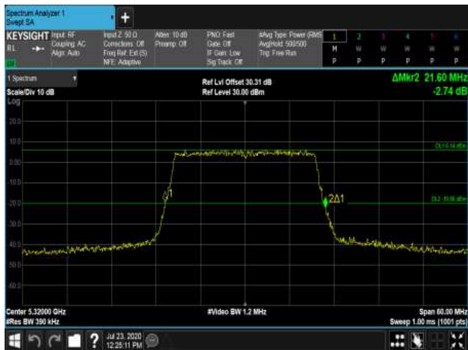
Figure 538 - 5320 MHz - 26 dB Emission Bandwidth
