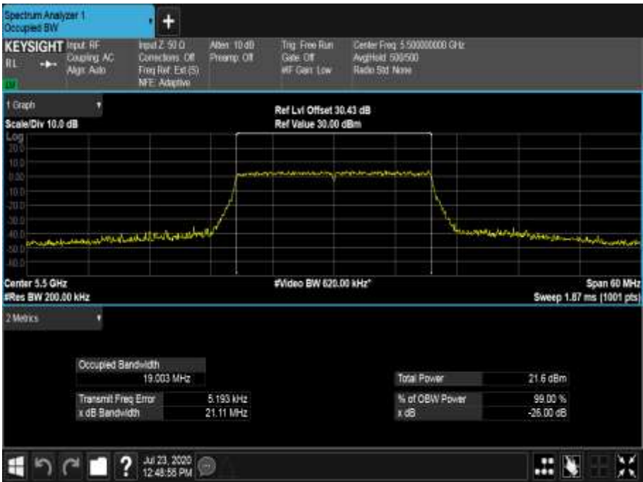
Figure 609 - 5500 MHz - 99% Occupied Bandwidth
