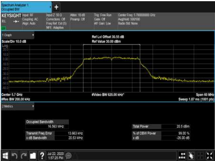
Figure 581 - 5700 MHz - 99% Occupied Bandwidth
