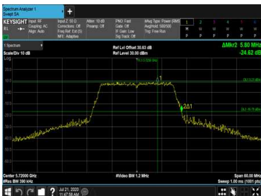
Figure 741 - 5720 MHz - 26 dB Emission Bandwidth
