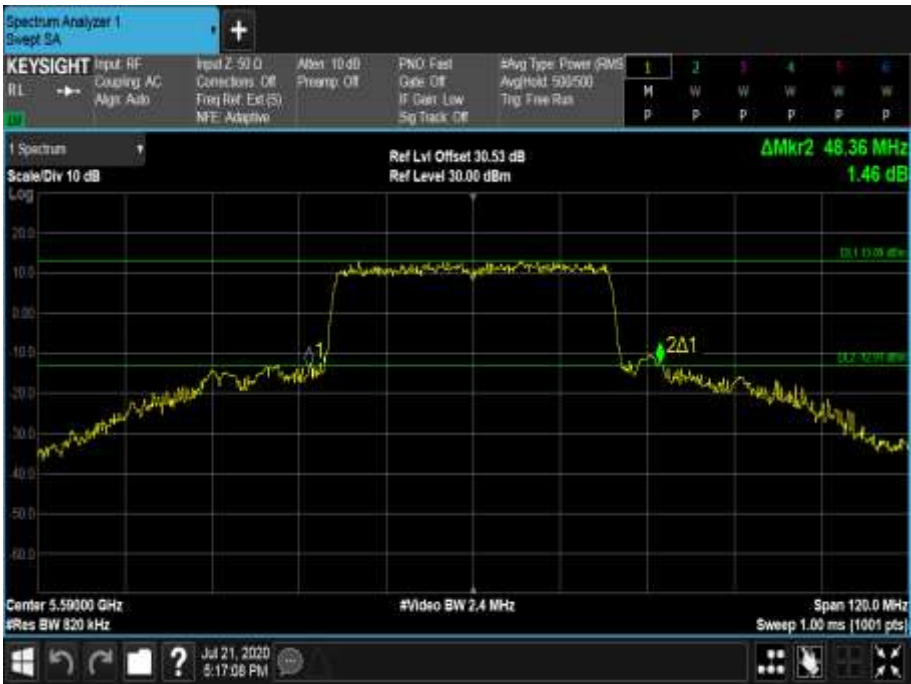
Figure 666 - 5590 MHz - 26 dB Emission Bandwidth
