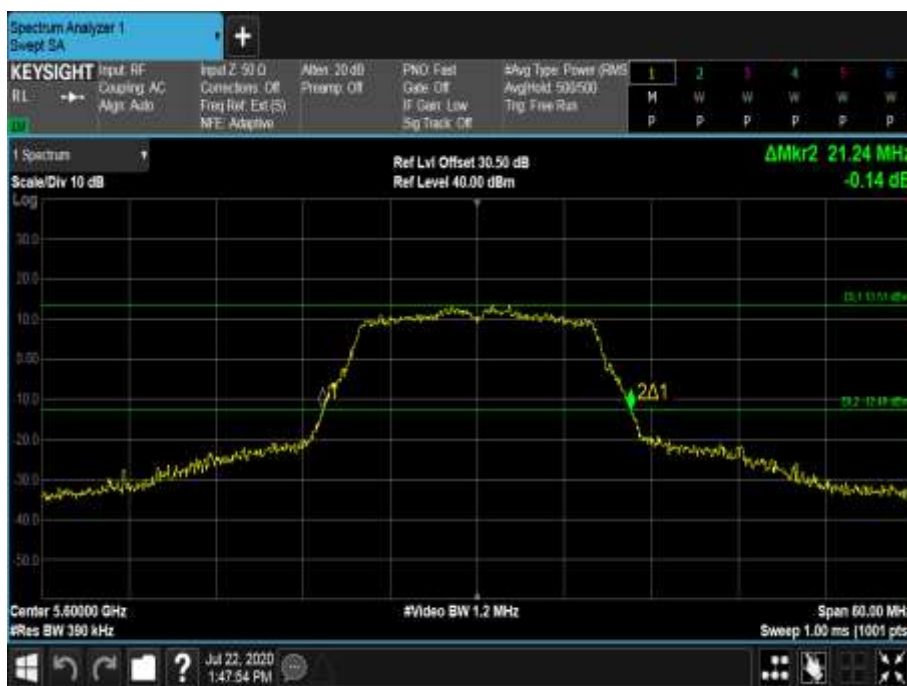
Figure 578 - 5600 MHz - 26 dB Emission Bandwidth
