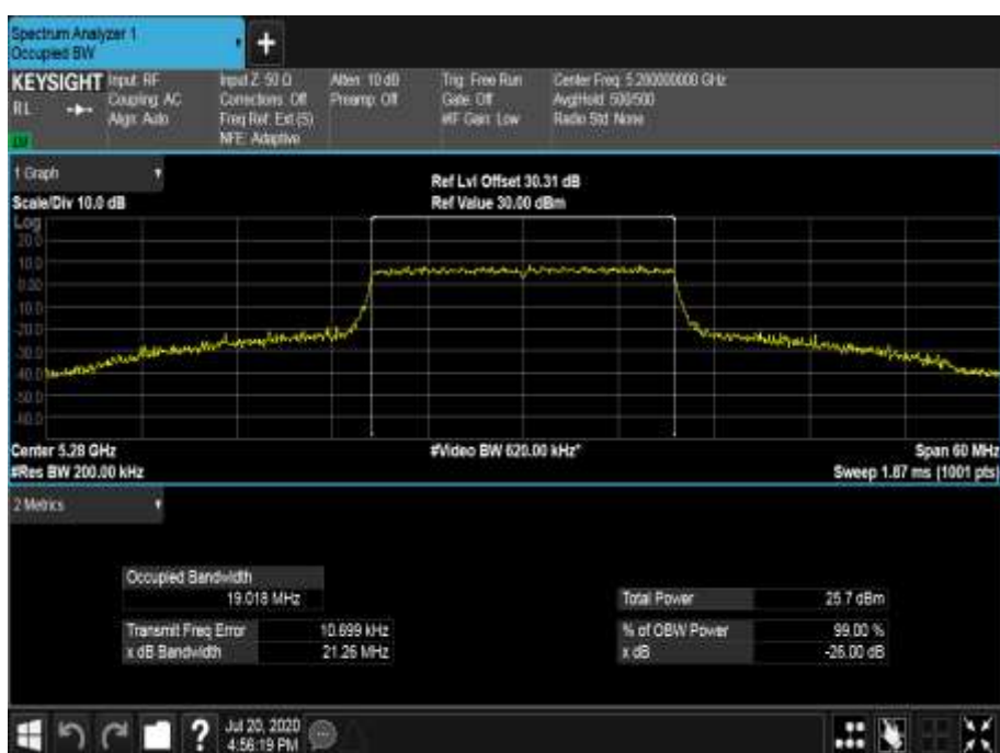
Figure 525 - 5280 MHz - 99% Occupied Bandwidth
