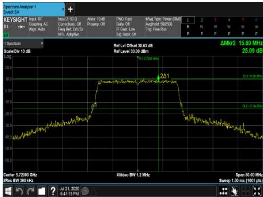
Figure 630 - 5720 MHz - 26 dB Emission Bandwidth
