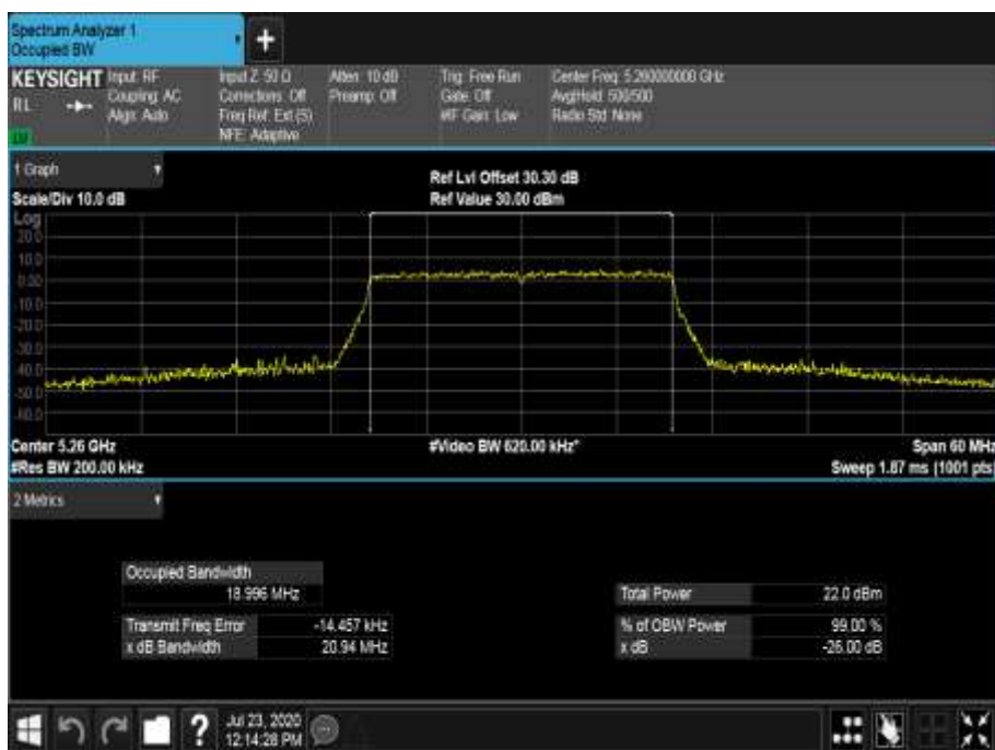
Figure 535 - 5260 MHz - 99% Occupied Bandwidth
