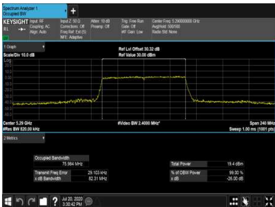
Figure 565 - 5290 MHz - 99% Occupied Bandwidth
