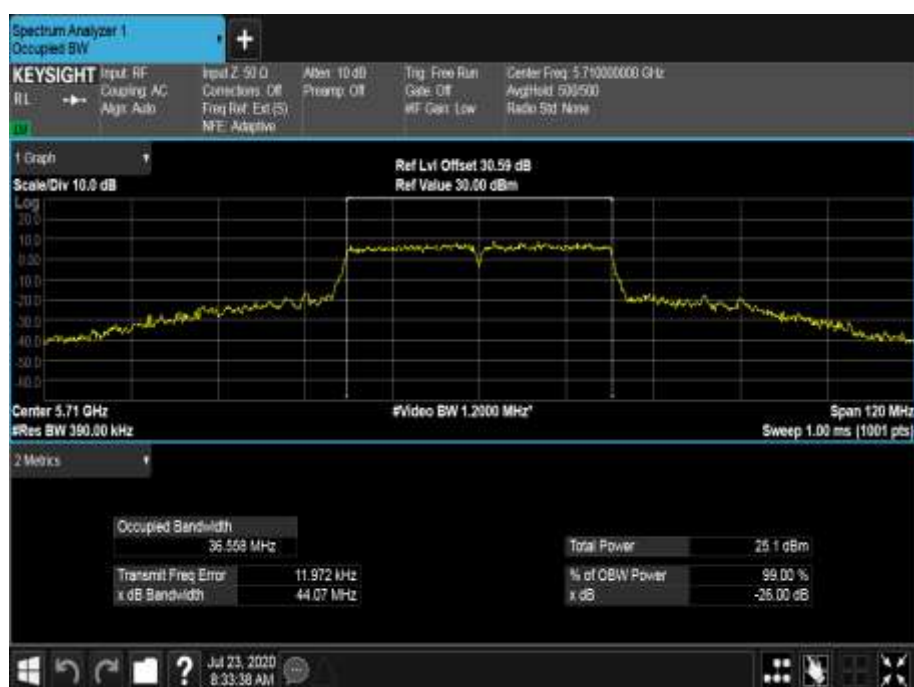
Figure 647 - 5710 MHz - 99% Occupied Bandwidth
