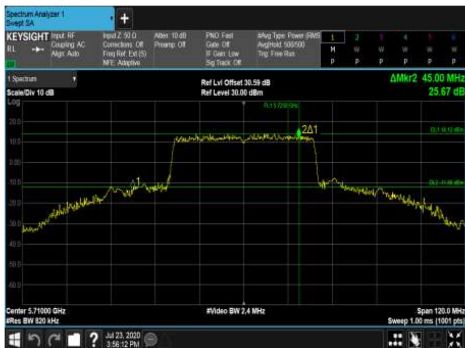
Figure 662 - 5710 MHz - 26 dB Emission Bandwidth
