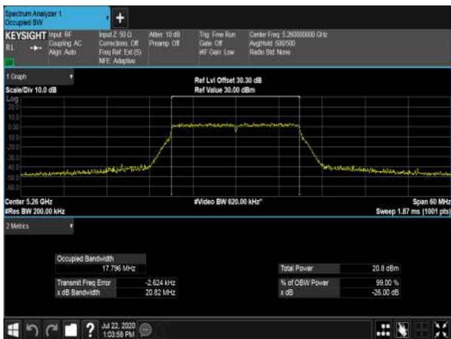
Figure 511 - 5260 MHz - 99% Occupied Bandwidth
