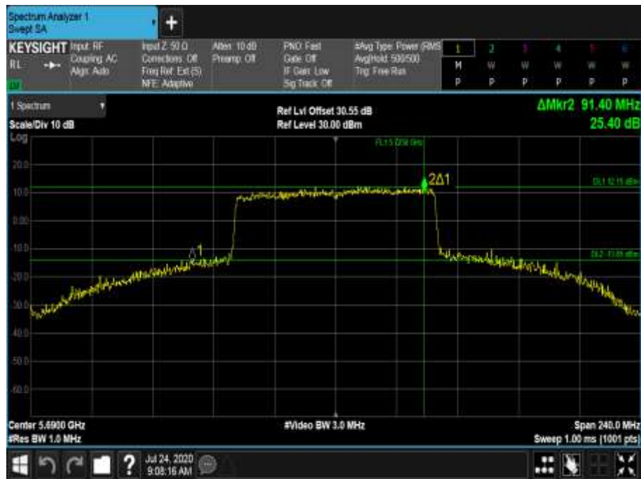
Figure 708 - 5690 MHz - 26 dB Emission Bandwidth
