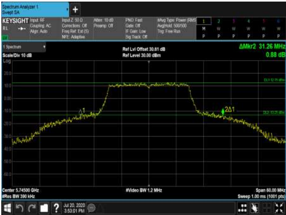
Figure 720 - 5745 MHz - 26 dB Emission Bandwidth
