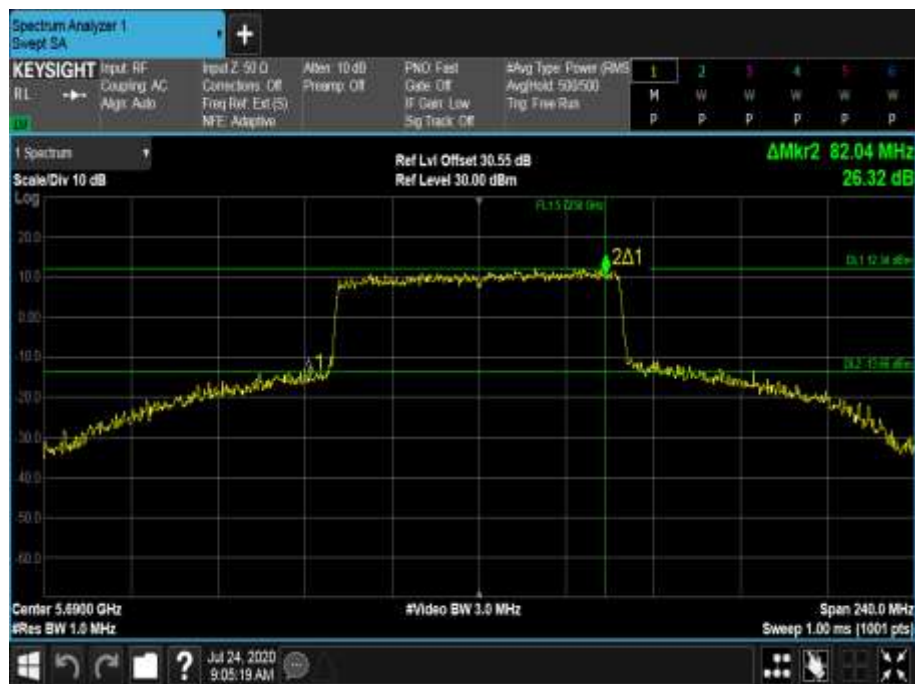
Figure 702 - 5690 MHz - 26 dB Emission Bandwidth
