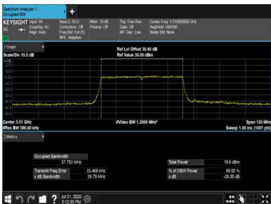
Figure 665 - 5510 MHz - 99% Occupied Bandwidth
