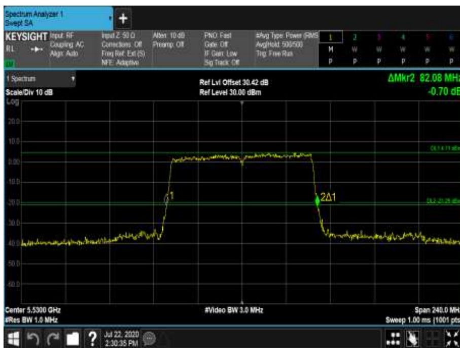
Figure 680 - 5530 MHz - 26 dB Emission Bandwidth
