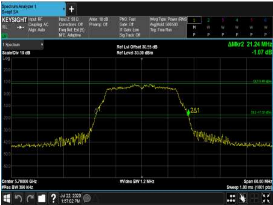
Figure 580 - 5700 MHz - 26 dB Emission Bandwidth
