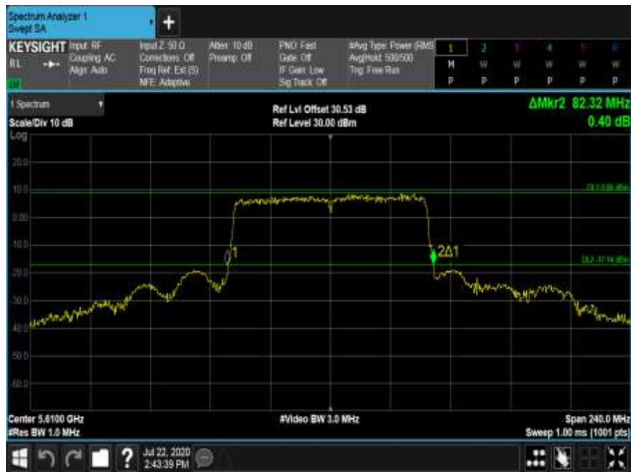
Figure 694 - 5610 MHz - 26 dB Emission Bandwidth
