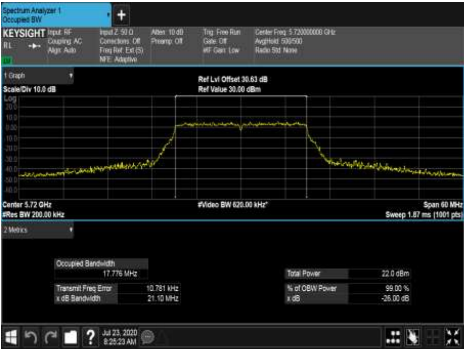
Figure 730 - 5720 MHz - 99% Occupied Bandwidth
