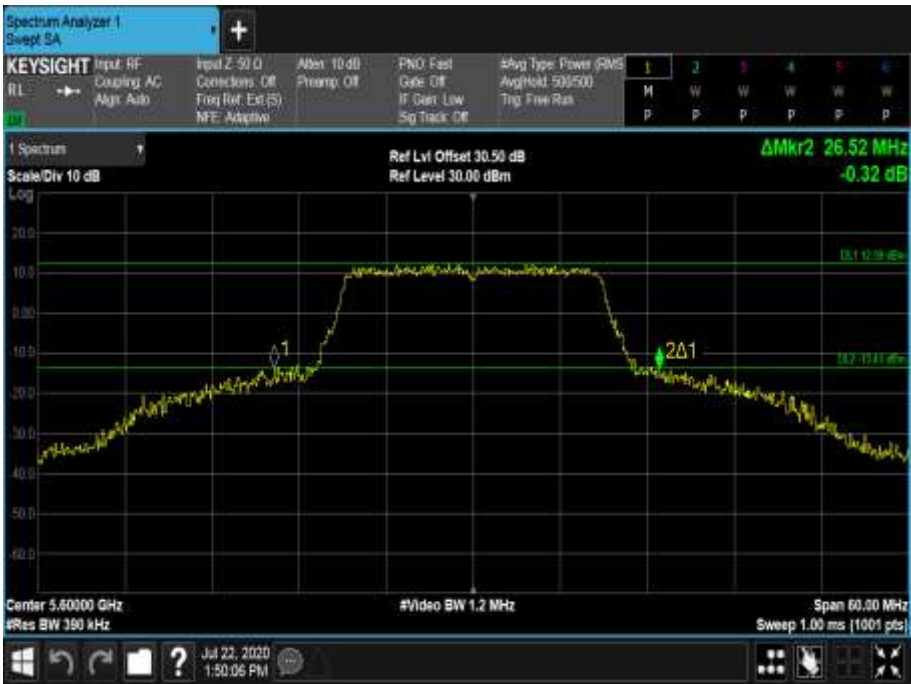
Figure 586 - 5600 MHz - 26 dB Emission Bandwidth
