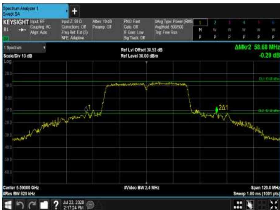
Figure 634 - 5590 MHz - 26 dB Emission Bandwidth
