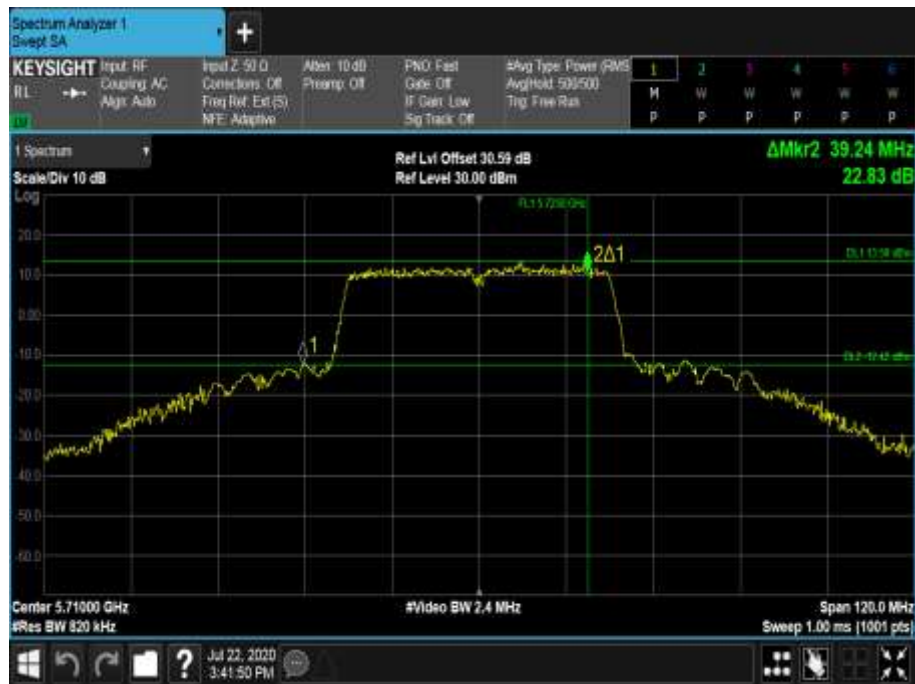
Figure 654 - 5710 MHz - 26 dB Emission Bandwidth
