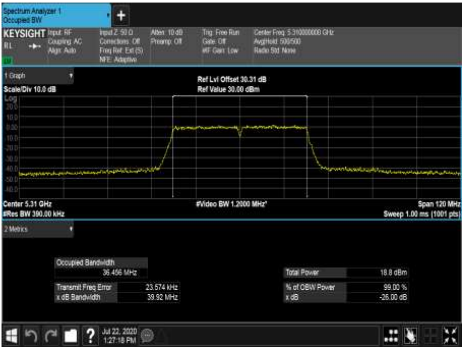
Figure 547 - 5310 MHz - 99% Occupied Bandwidth
