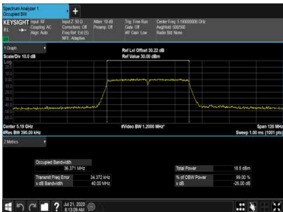
Figure 371 - 5190 MHz - 99% Occupied Bandwidth
