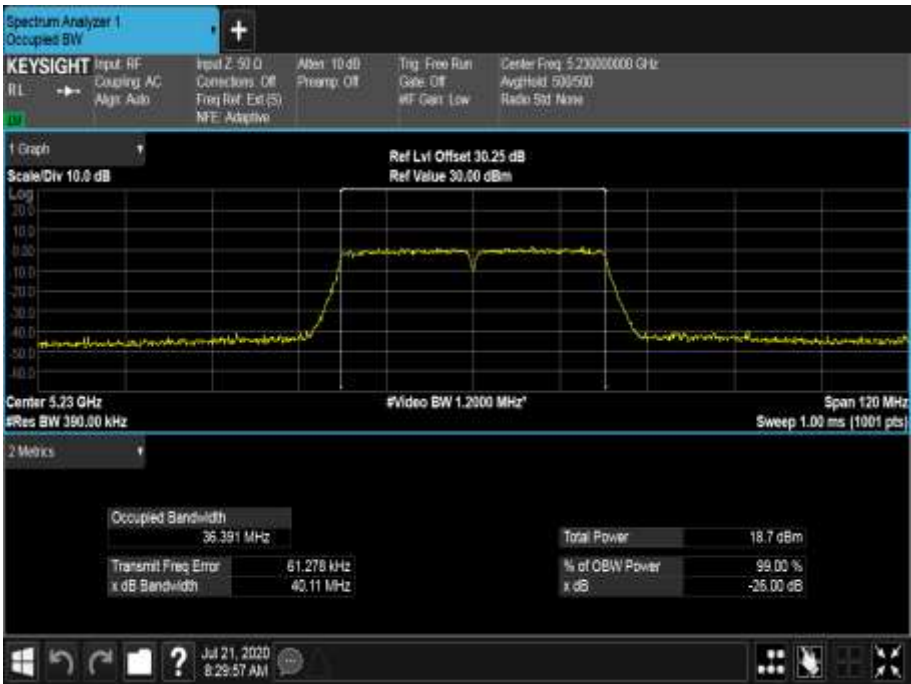
Figure 377 - 5230 MHz - 99% Occupied Bandwidth
