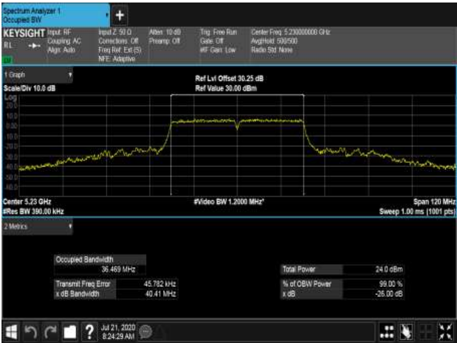
Figure 373 - 5230 MHz - 99% Occupied Bandwidth
