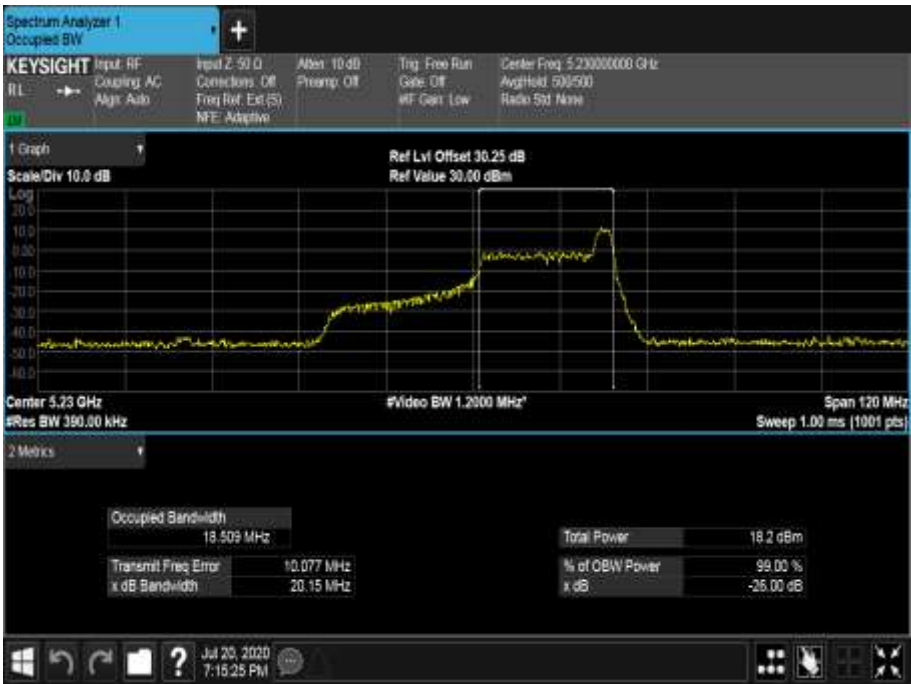
Figure 397 - 5230 MHz - 99% Occupied Bandwidth
