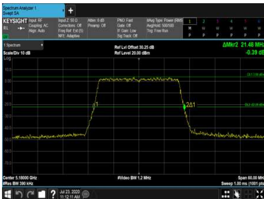
Figure 324 - 5180 MHz - 26 dB Emission Bandwidth
