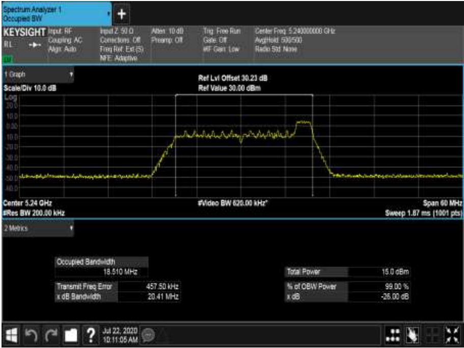
Figure 347 - 5240 MHz - 99% Occupied Bandwidth
