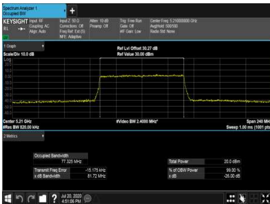
Figure 465 - 5210 MHz - 99% Occupied Bandwidth
