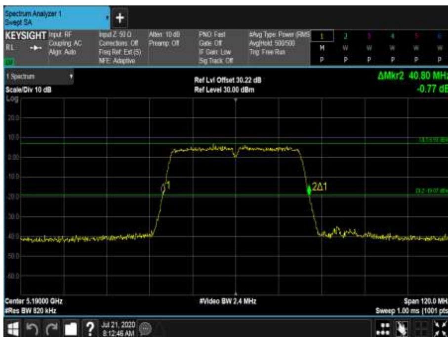
Figure 370 - 5190 MHz - 26 dB Emission Bandwidth
