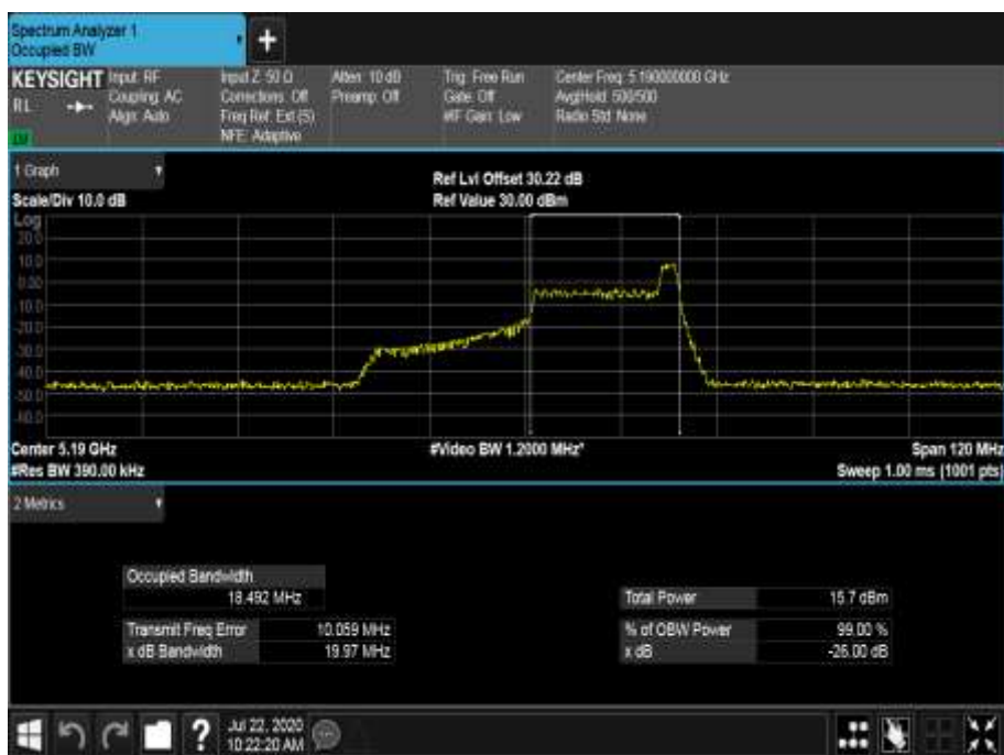
Figure 443 - 5190 MHz - 99% Occupied Bandwidth
