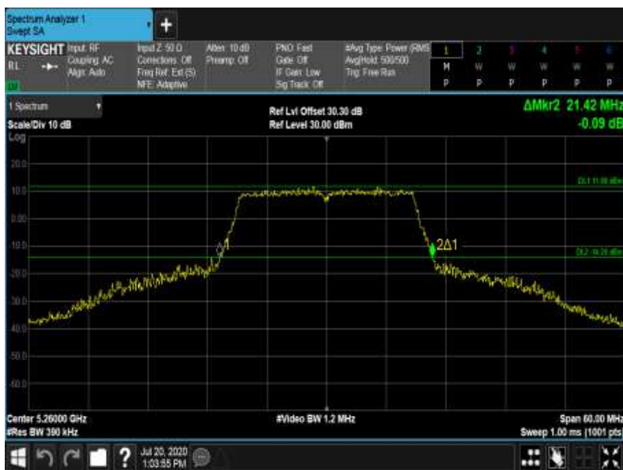
Figure 504 - 5260 MHz - 26 dB Emission Bandwidth
