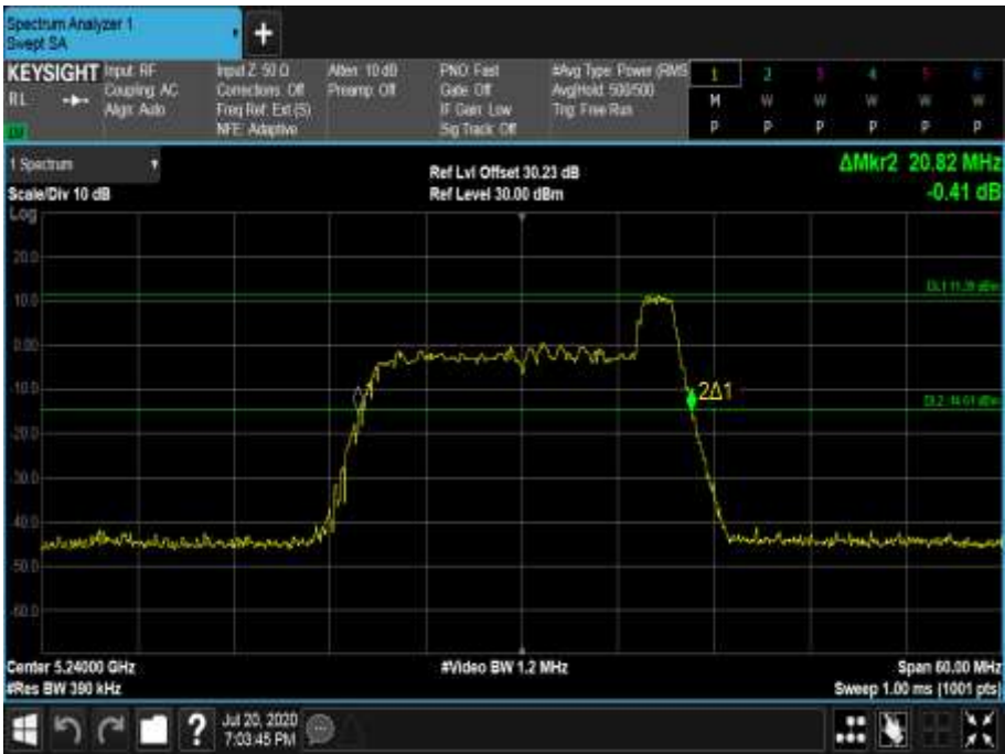
Figure 274 - 5240 MHz - 26 dB Emission Bandwidth
