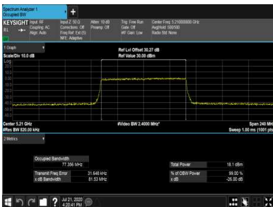
Figure 489 - 5210 MHz - 99% Occupied Bandwidth
