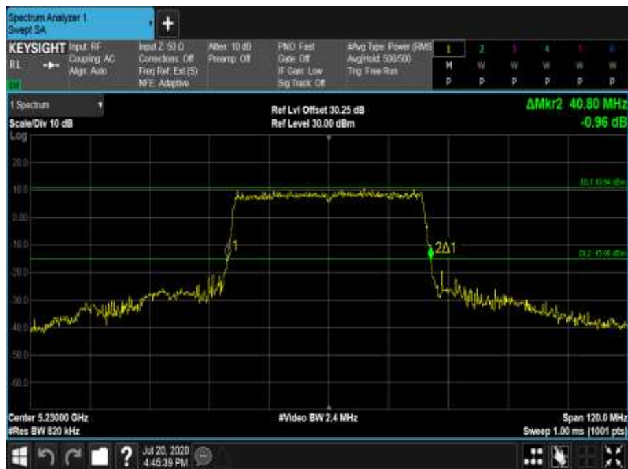
Figure 384 - 5230 MHz - 26 dB Emission Bandwidth
