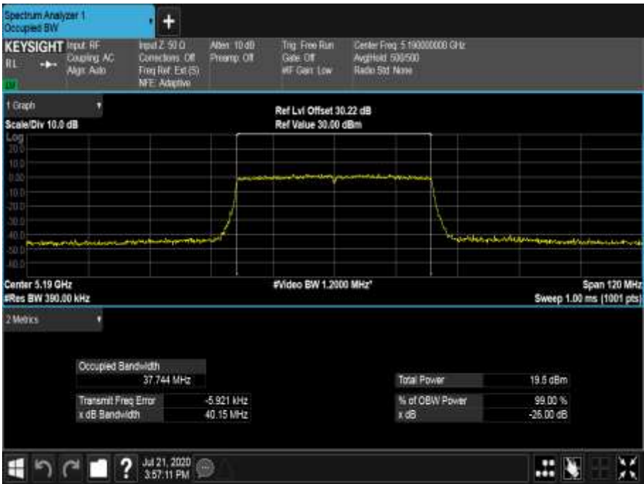
Figure 431 - 5190 MHz - 99% Occupied Bandwidth
