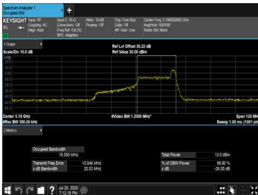
Figure 399 - 5190 MHz - 99% Occupied Bandwidth
