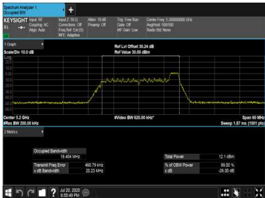
Figure 279 - 5200 MHz - 99% Occupied Bandwidth
