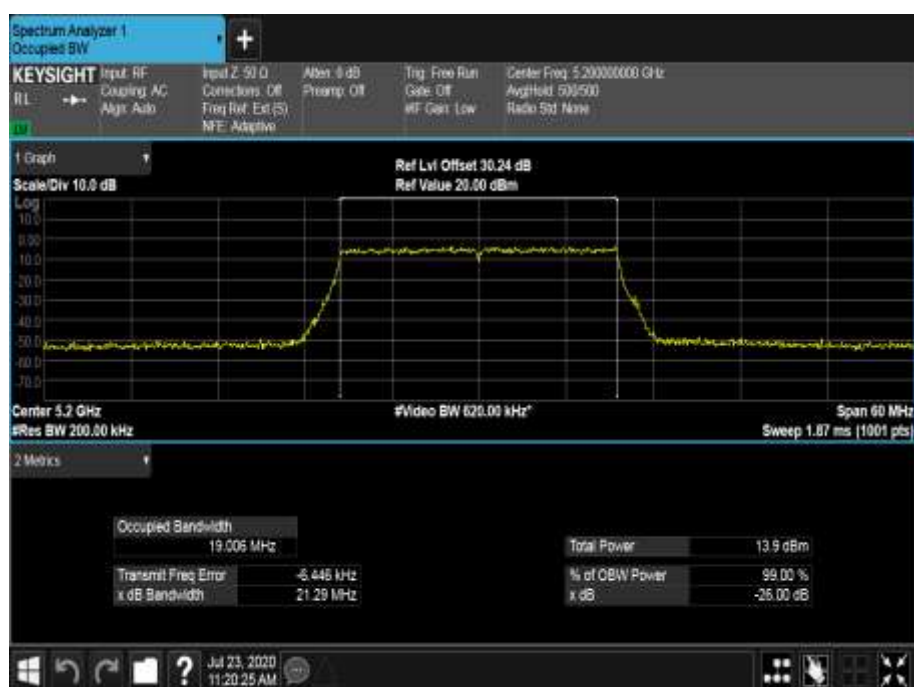
Figure 291 - 5200 MHz - 99% Occupied Bandwidth
