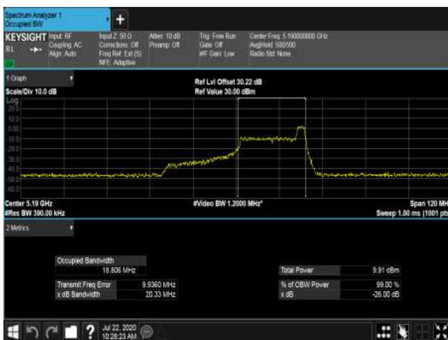
Figure 447 - 5190 MHz - 99% Occupied Bandwidth
