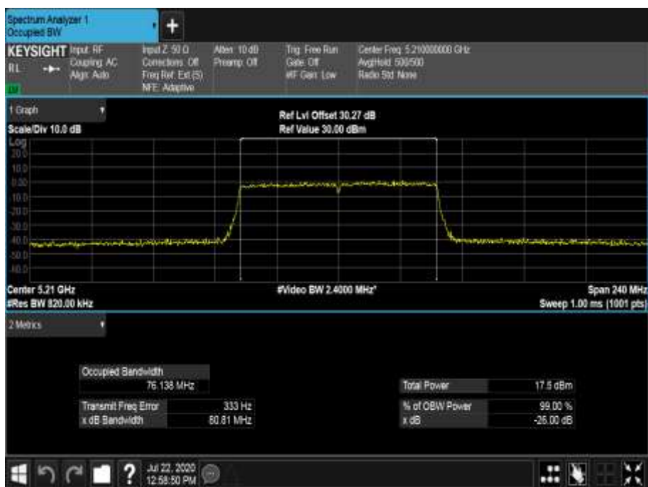
Figure 457 - 5210 MHz - 99% Occupied Bandwidth
