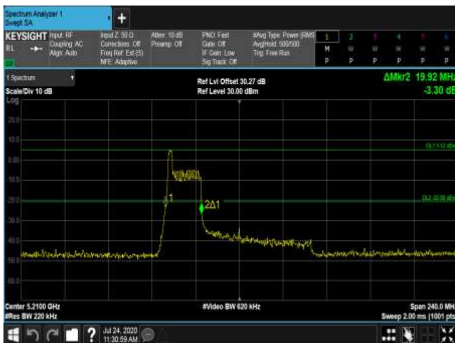
Figure 478 - 5210 MHz - 26 dB Emission Bandwidth
