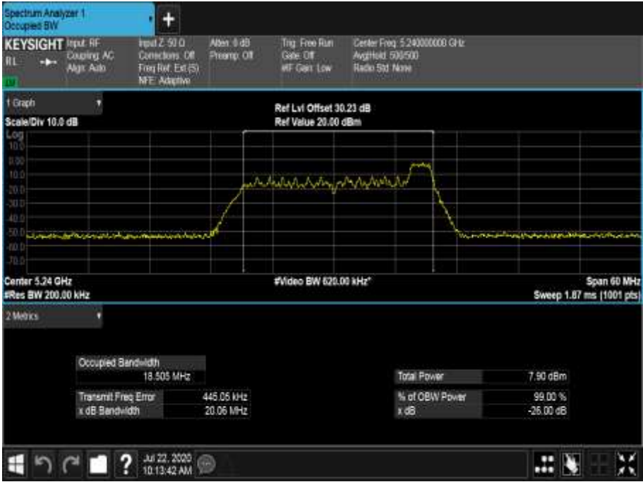
Figure 317 - 5240 MHz - 99% Occupied Bandwidth
