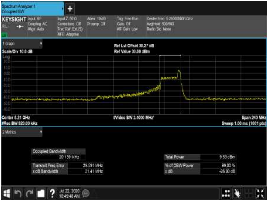
Figure 485 - 5210 MHz - 99% Occupied Bandwidth
