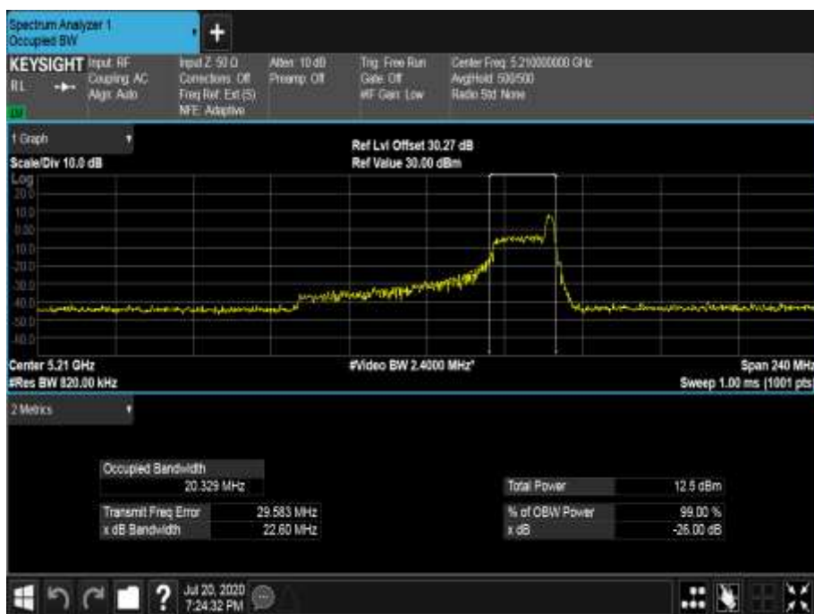
Figure 473 - 5210 MHz - 99% Occupied Bandwidth
