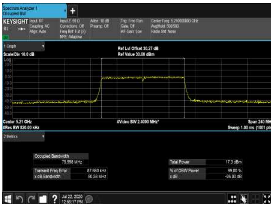
Figure 459 - 5210 MHz - 99% Occupied Bandwidth
