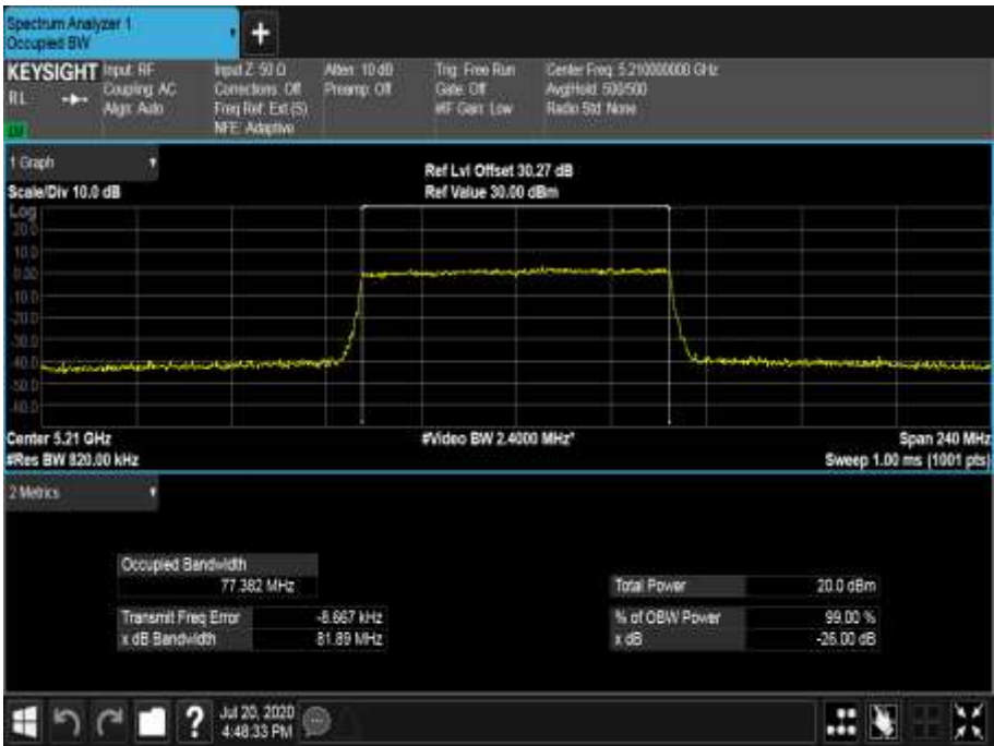
Figure 463 - 5210 MHz - 99% Occupied Bandwidth
