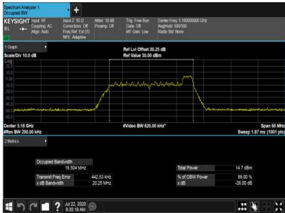
Figure 343 - 5180 MHz - 99% Occupied Bandwidth
