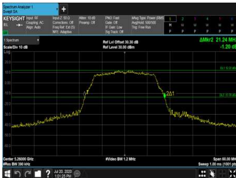
Figure 498 - 5260 MHz - 26 dB Emission Bandwidth
