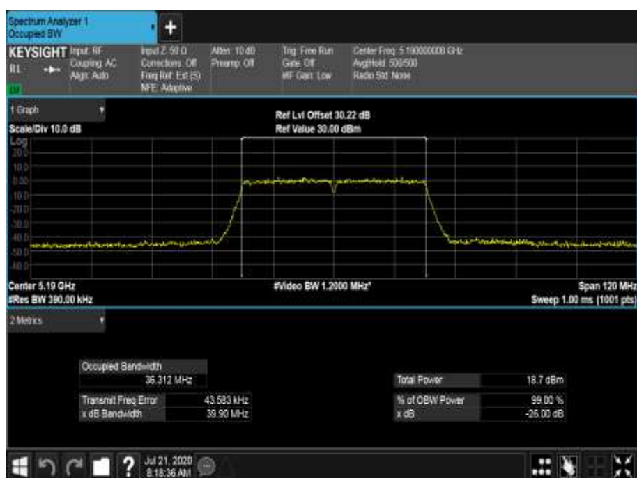
Figure 375 - 5190 MHz - 99% Occupied Bandwidth
