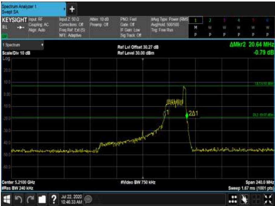
Figure 494 - 5210 MHz - 26 dB Emission Bandwidth
