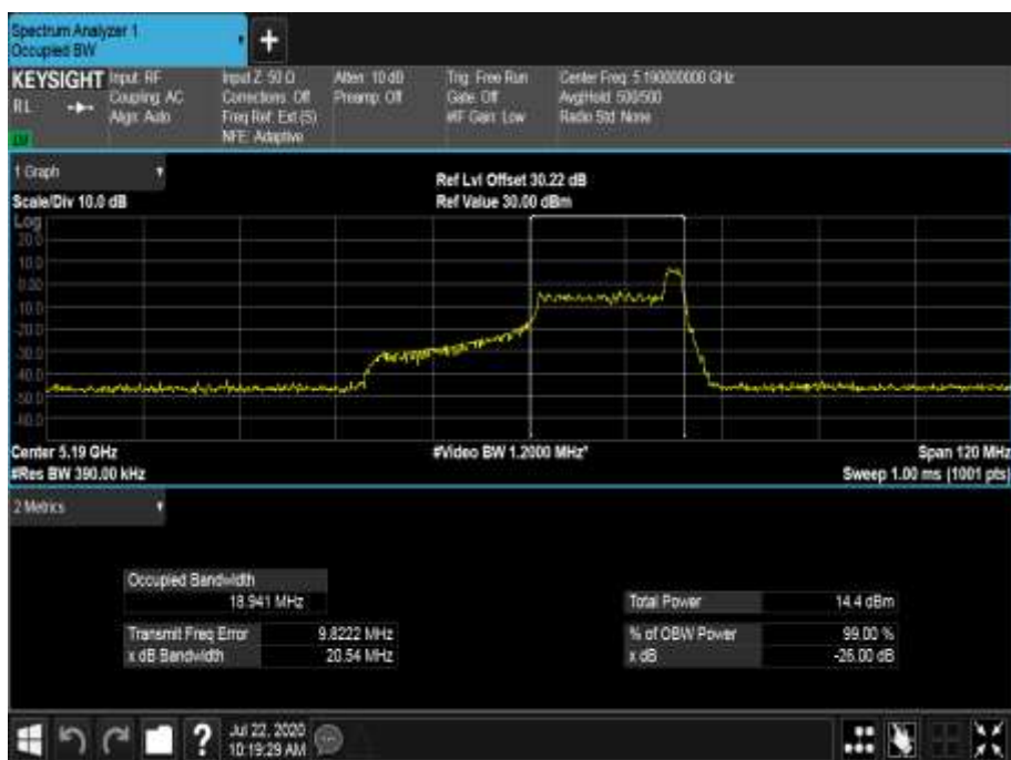
Figure 419 - 5190 MHz - 99% Occupied Bandwidth
