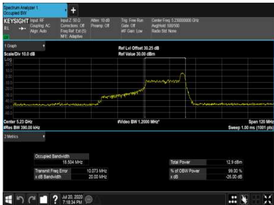
Figure 401 - 5230 MHz - 99% Occupied Bandwidth
