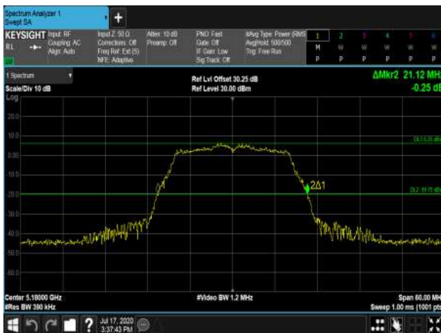
Figure 204 - 5180 MHz - 26 dB Emission Bandwidth
