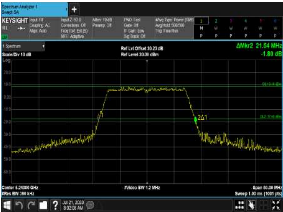
Figure 238 - 5240 MHz - 26 dB Emission Bandwidth
