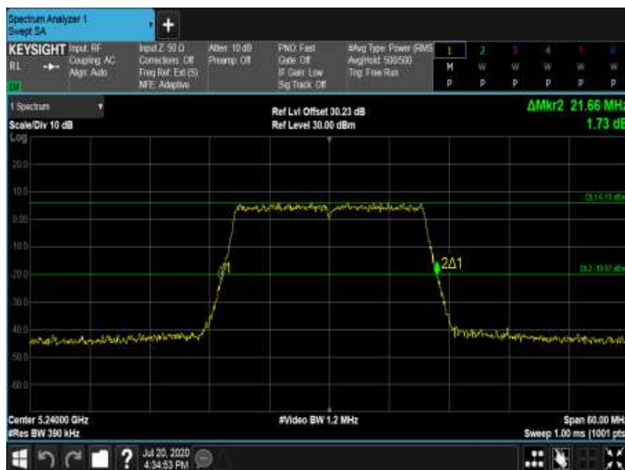
Figure 256 - 5240 MHz - 26 dB Emission Bandwidth
