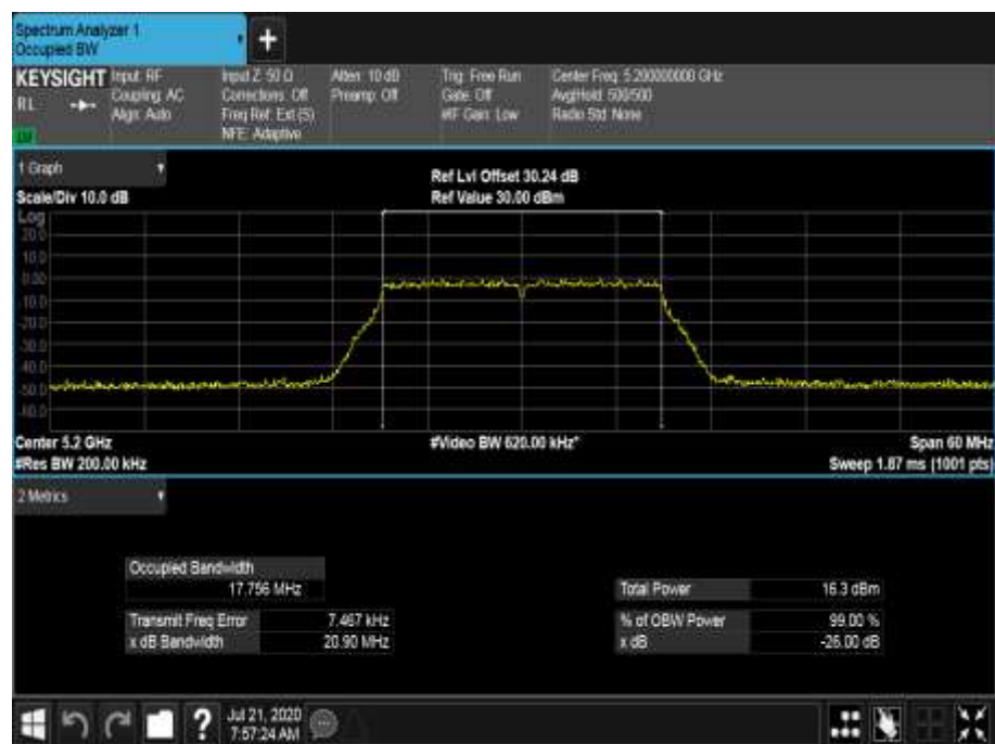
Figure 243 - 5200 MHz - 99% Occupied Bandwidth
