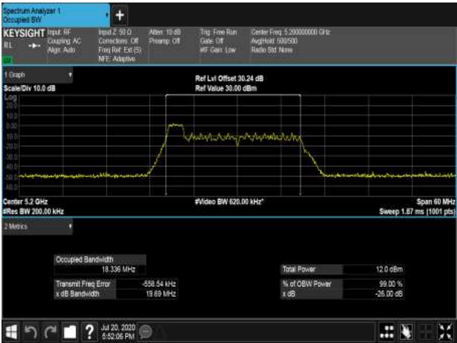
Figure 267 - 5200 MHz - 99% Occupied Bandwidth
