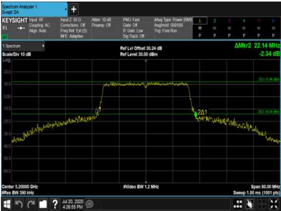
Figure 248 - 5200 MHz - 26 dB Emission Bandwidth
