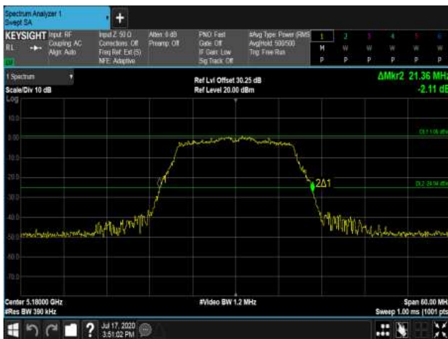
Figure 216 - 5180 MHz - 26 dB Emission Bandwidth
