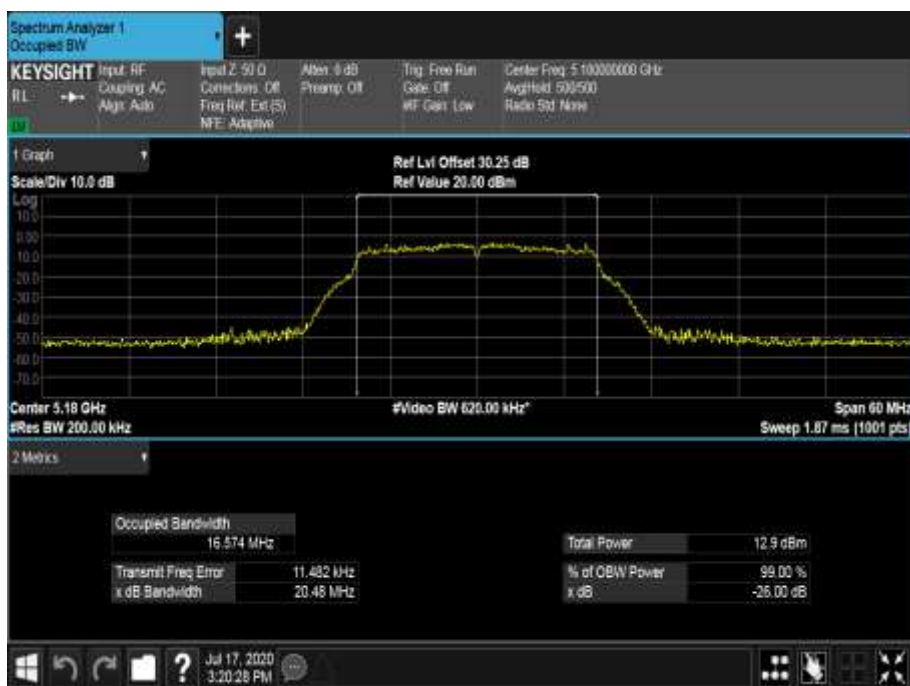
Figure 211 - 5180 MHz - 99% Occupied Bandwidth
