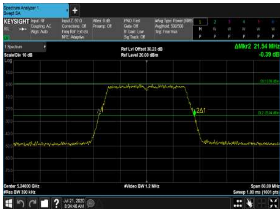
Figure 232 - 5240 MHz - 26 dB Emission Bandwidth
