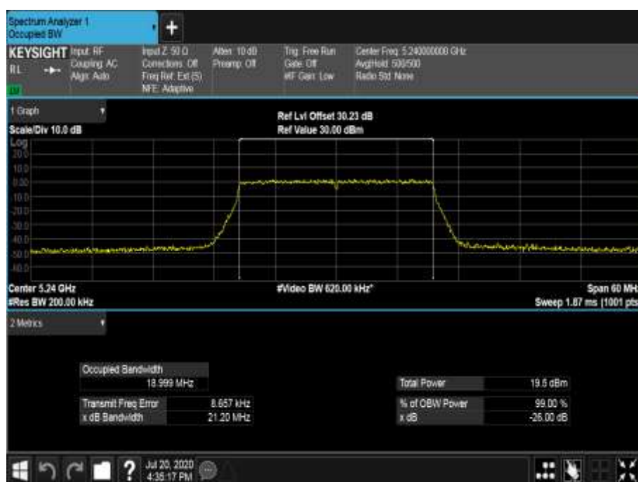
Figure 257 - 5240 MHz - 99% Occupied Bandwidth
