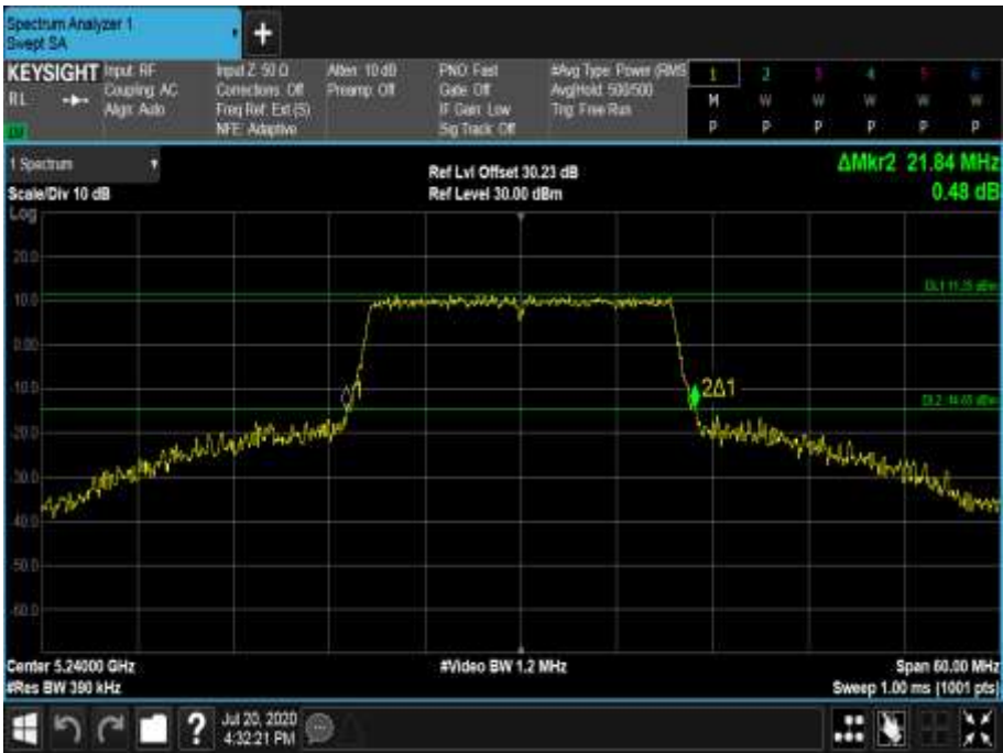
Figure 250 - 5240 MHz - 26 dB Emission Bandwidth
