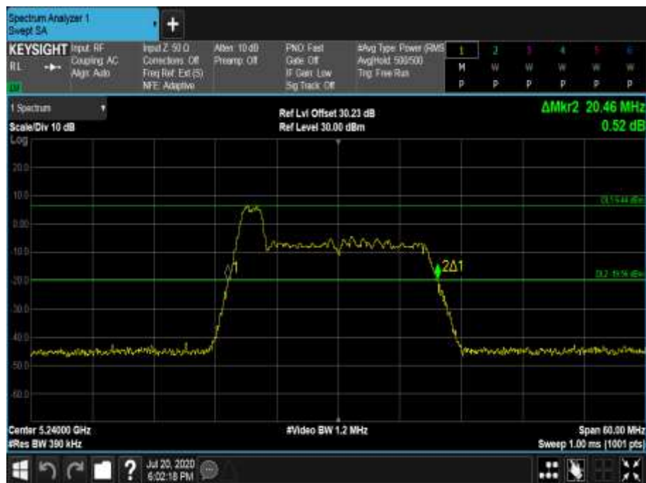
Figure 268 - 5240 MHz - 26 dB Emission Bandwidth
