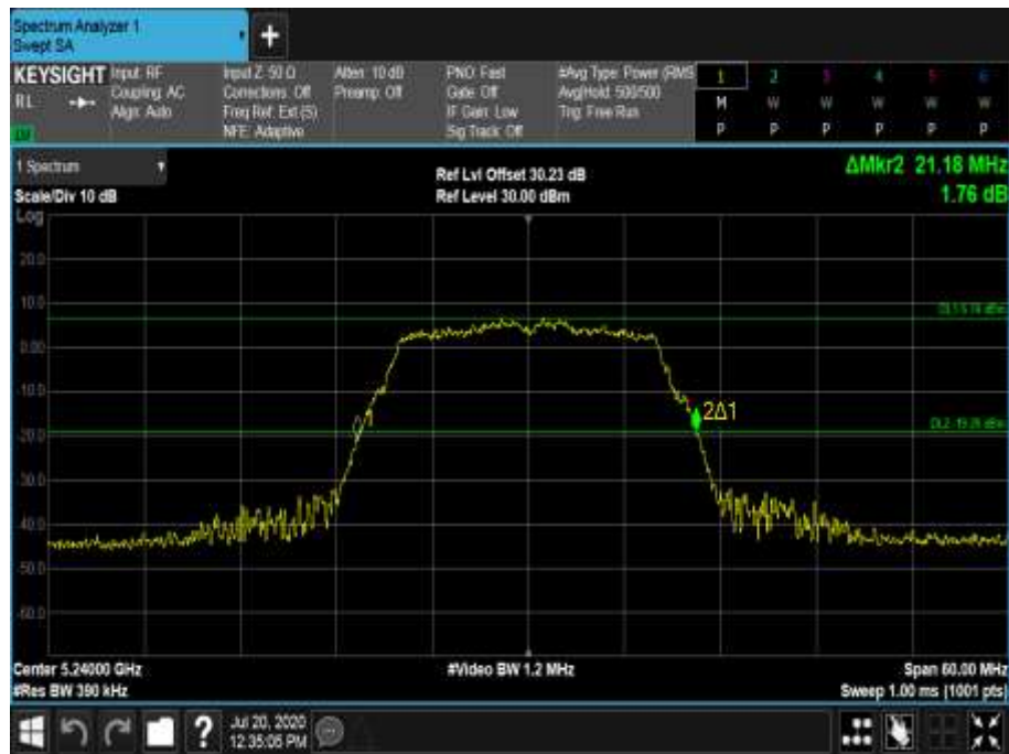
Figure 208 - 5240 MHz - 26 dB Emission Bandwidth
