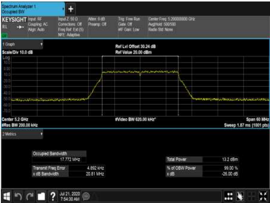
Figure 231 - 5200 MHz - 99% Occupied Bandwidth
