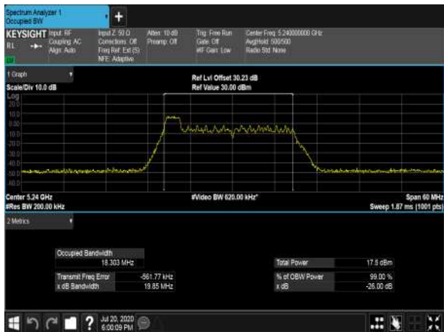
Figure 263 - 5240 MHz - 99% Occupied Bandwidth
