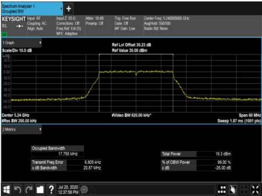
Figure 221 - 5240 MHz - 99% Occupied Bandwidth
