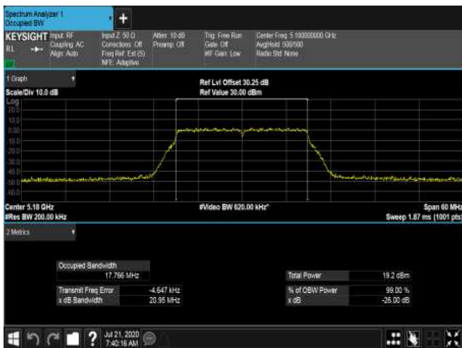
Figure 235 - 5180 MHz - 99% Occupied Bandwidth
