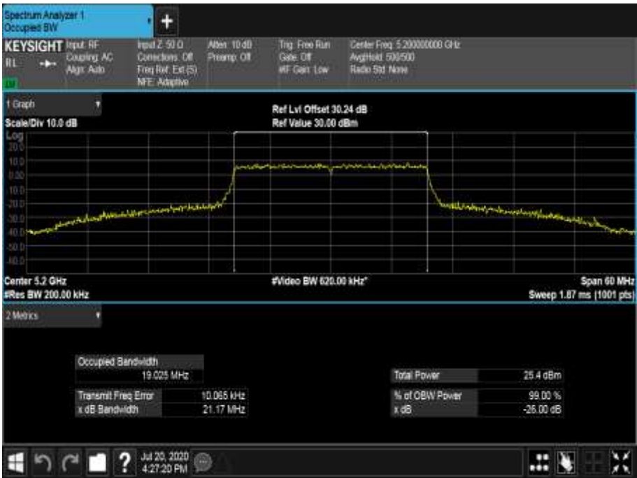
Figure 249 - 5200 MHz - 99% Occupied Bandwidth
