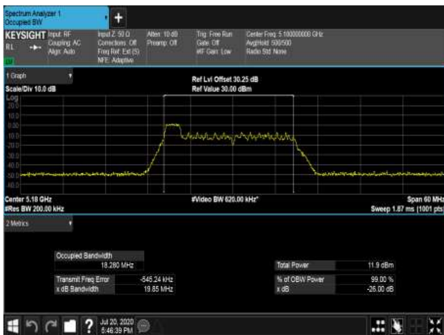
Figure 265 - 5180 MHz - 99% Occupied Bandwidth
