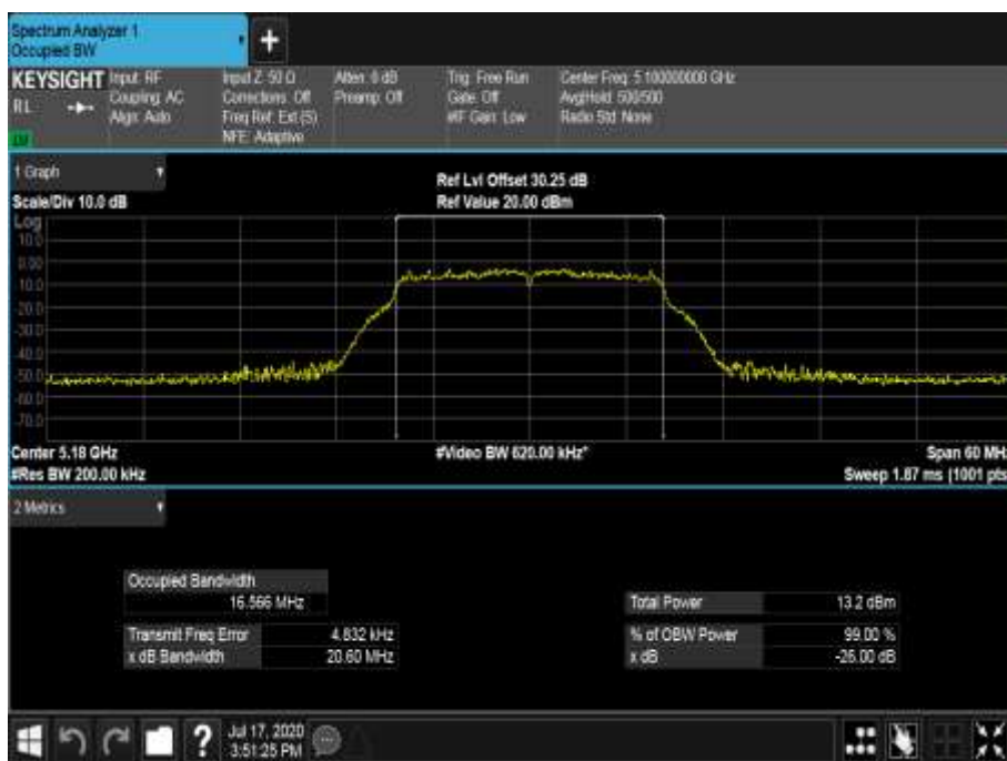
Figure 217 - 5180 MHz - 99% Occupied Bandwidth
