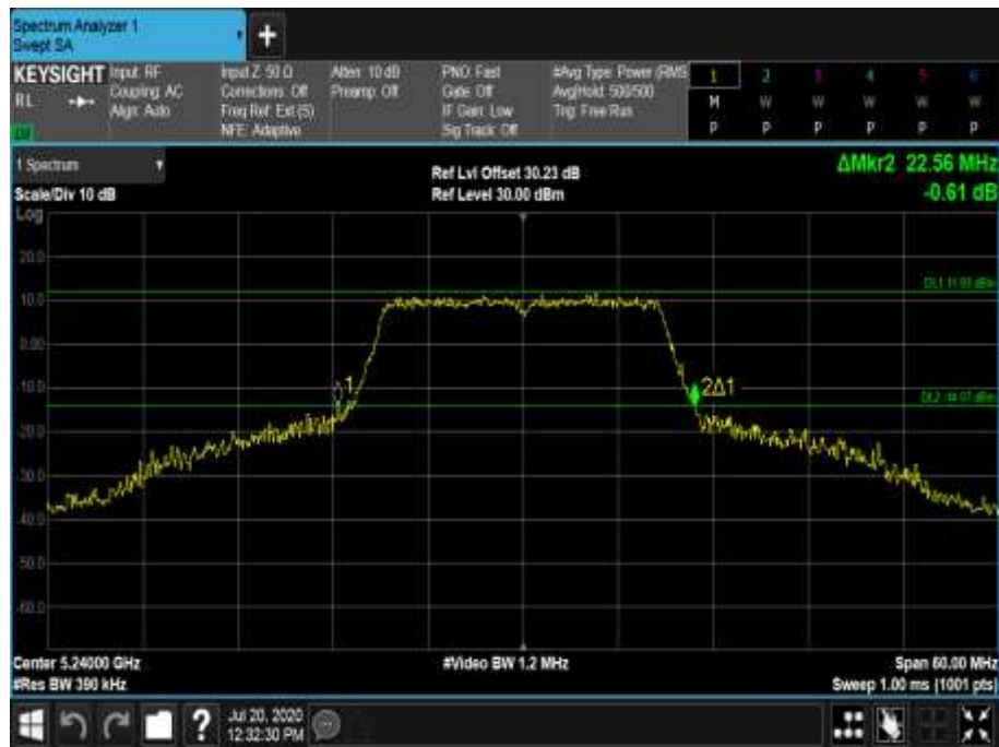
Figure 214 - 5240 MHz - 26 dB Emission Bandwidth
