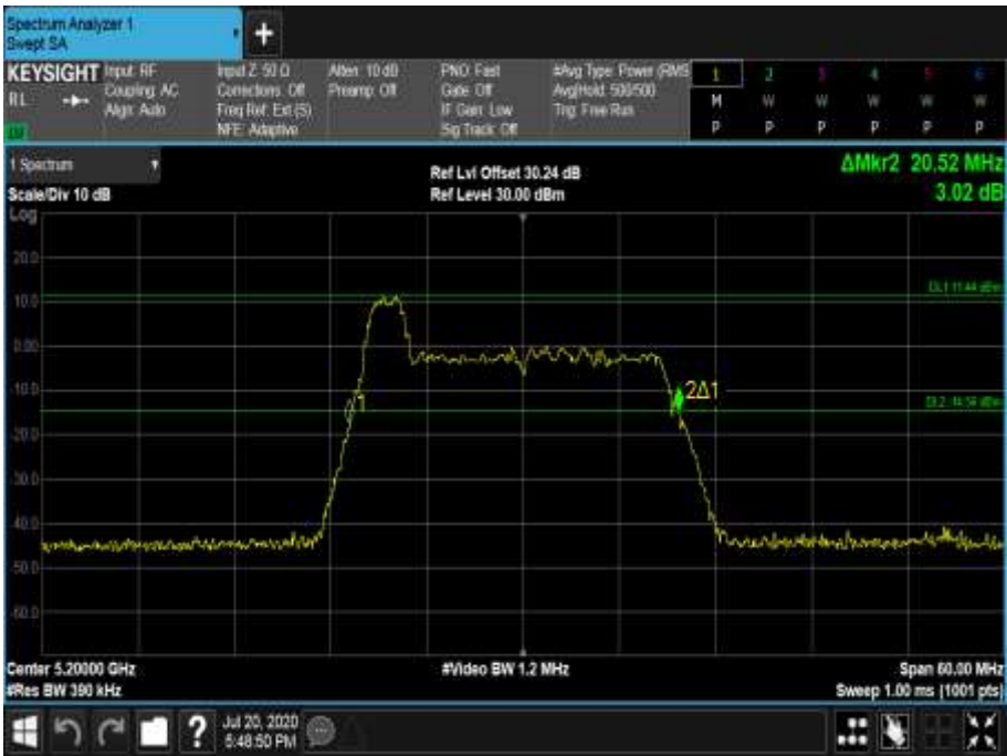
Figure 260 - 5200 MHz - 26 dB Emission Bandwidth
