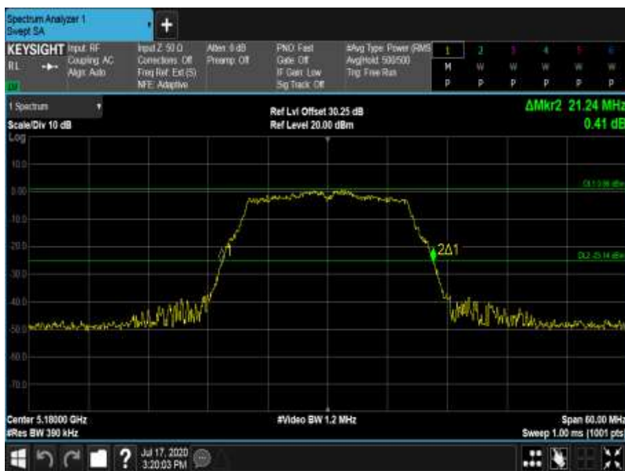
Figure 210 - 5180 MHz - 26 dB Emission Bandwidth
