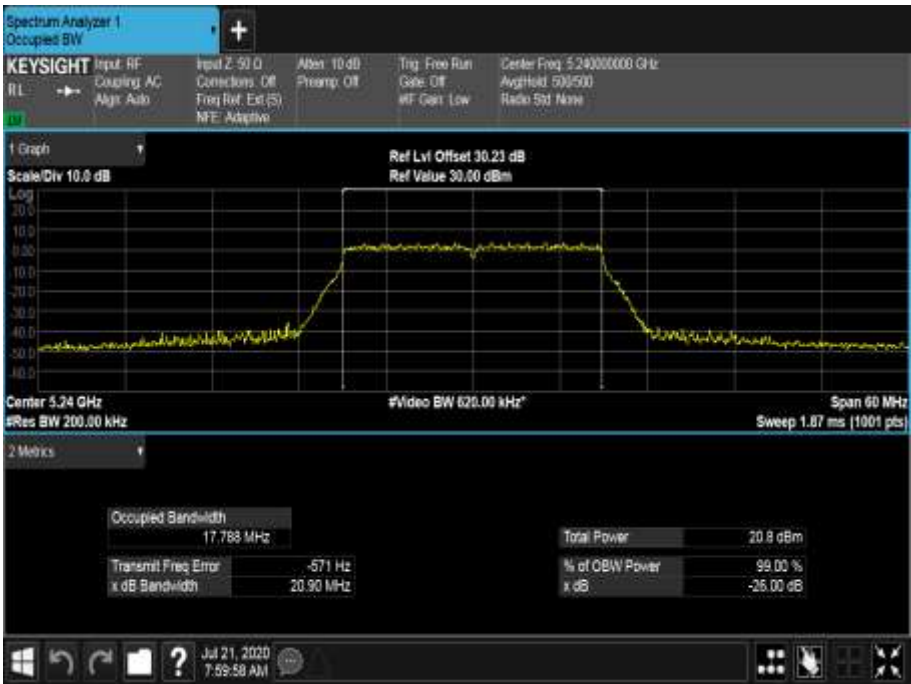
Figure 227 - 5240 MHz - 99% Occupied Bandwidth
