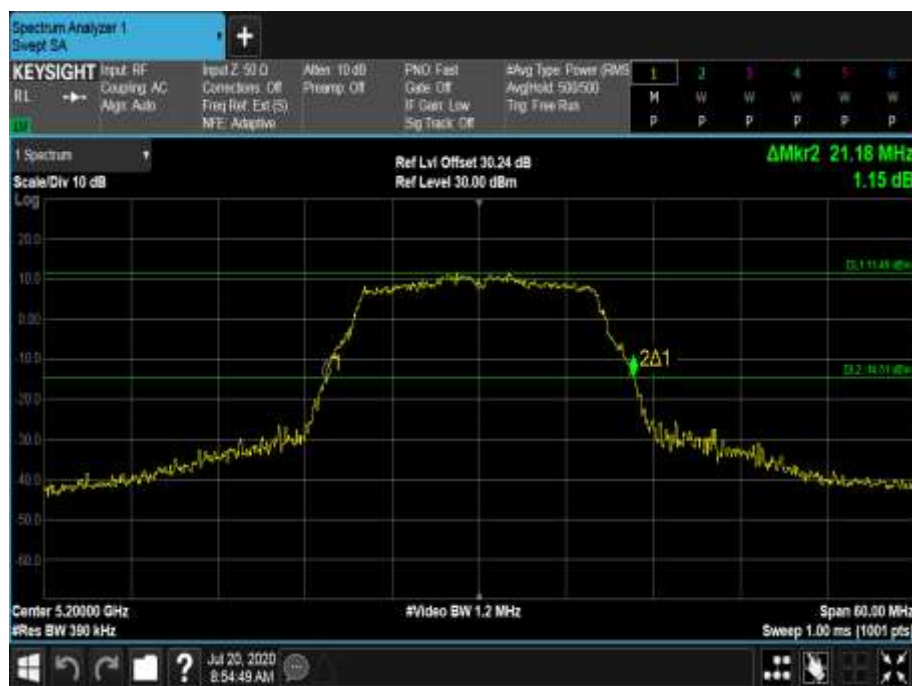
Figure 200 - 5200 MHz - 26 dB Emission Bandwidth
