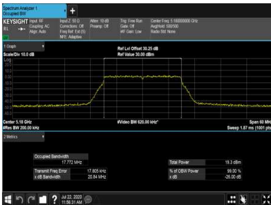
Figure 223 - 5180 MHz - 99% Occupied Bandwidth
