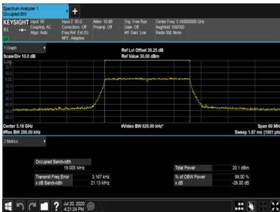
Figure 247 - 5180 MHz - 99% Occupied Bandwidth
