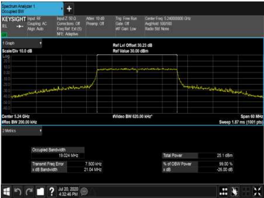
Figure 251 - 5240 MHz - 99% Occupied Bandwidth
