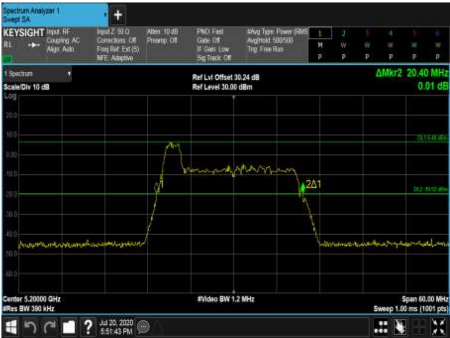
Figure 266 - 5200 MHz - 26 dB Emission Bandwidth
