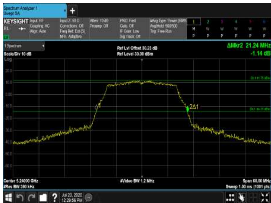
Figure 202 - 5240 MHz - 26 dB Emission Bandwidth
