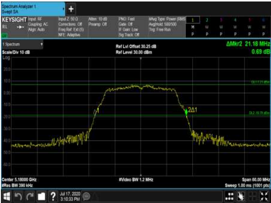
Figure 198 - 5180 MHz - 26 dB Emission Bandwidth
