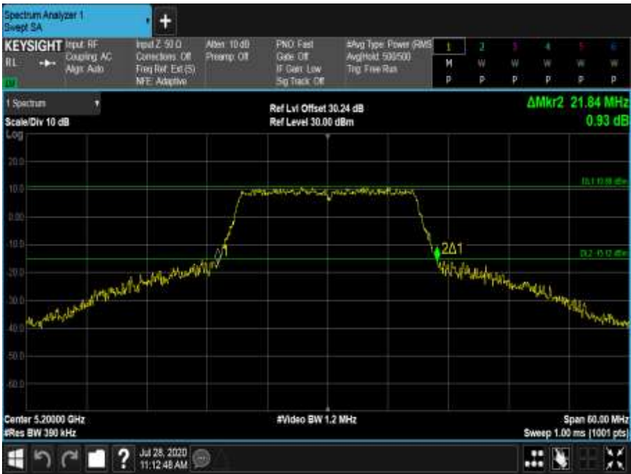
Figure 212 - 5200 MHz - 26 dB Emission Bandwidth
