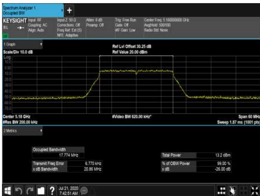
Figure 229 - 5180 MHz - 99% Occupied Bandwidth
