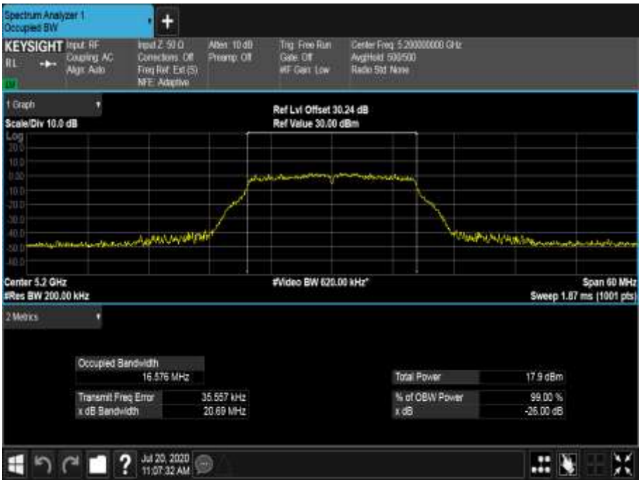
Figure 207 - 5200 MHz - 99% Occupied Bandwidth
