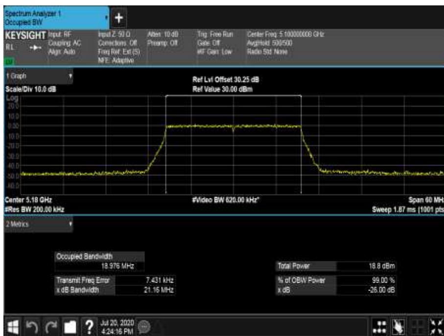
Figure 253 - 5180 MHz - 99% Occupied Bandwidth
