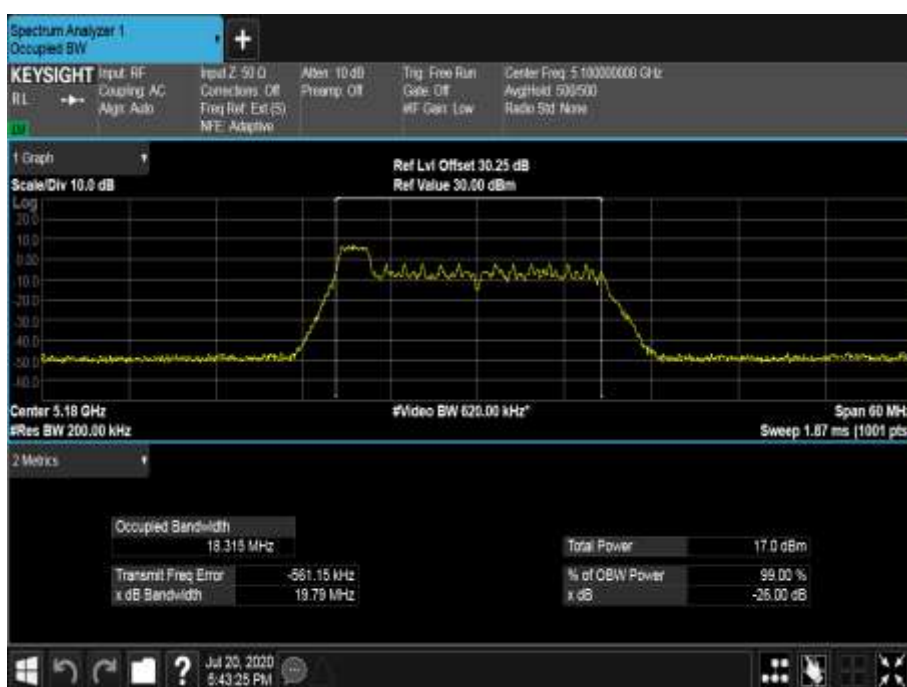
Figure 259 - 5180 MHz - 99% Occupied Bandwidth
