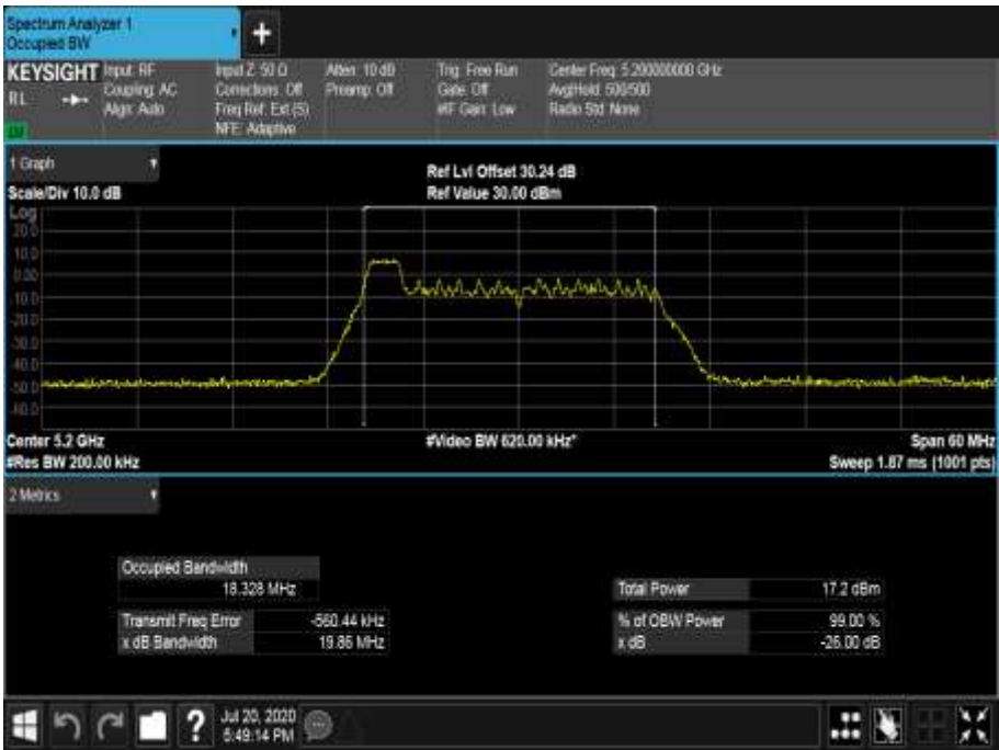
Figure 261 - 5200 MHz - 99% Occupied Bandwidth
