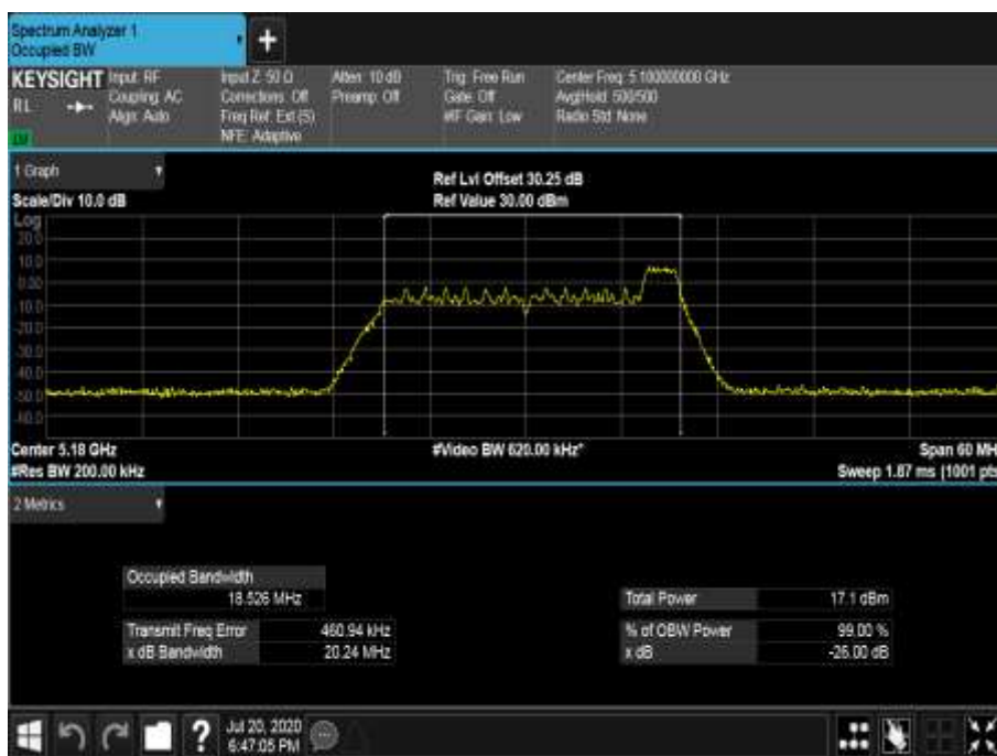
Figure 271 - 5180 MHz - 99% Occupied Bandwidth
