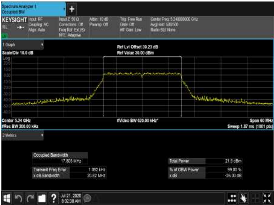
Figure 239 - 5240 MHz - 99% Occupied Bandwidth
