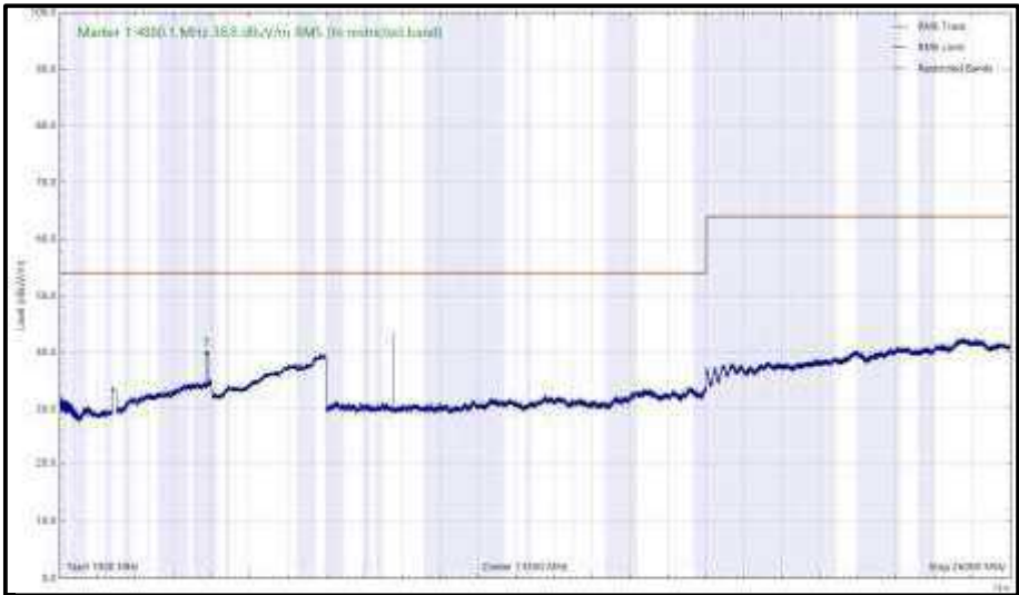
Figure 305 - 2440 MHz (CH17), LE1M, iPA, Core 1, 1 GHz to 26 GHz, Vertical (RMS)
