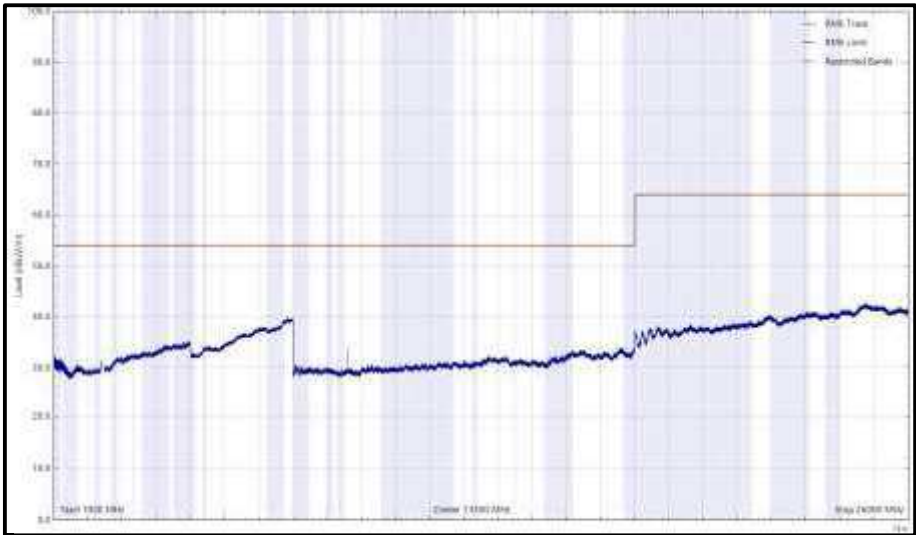
Figure 285 - 2402 MHz (CH0), LE1M, iPA, Core 0, 1 GHz to 26 GHz, Vertical (RMS)
