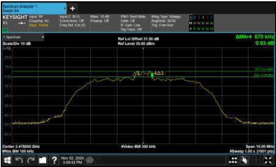
Figure 96 - Core 1 HDR8 2478 MHz (CH76) 6 dB Bandwidth
