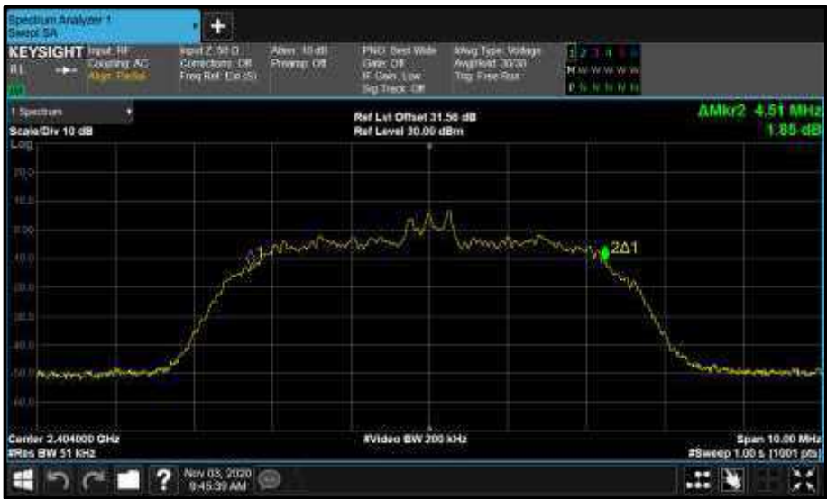
Figure 85 - Core 2 HDR8 2404 MHz (CH2) 99% Bandwidth
