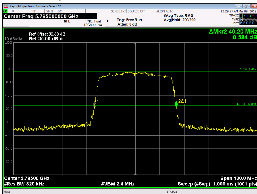
Figure 328 - 5795 MHz - 26 dB Emission Bandwidth
