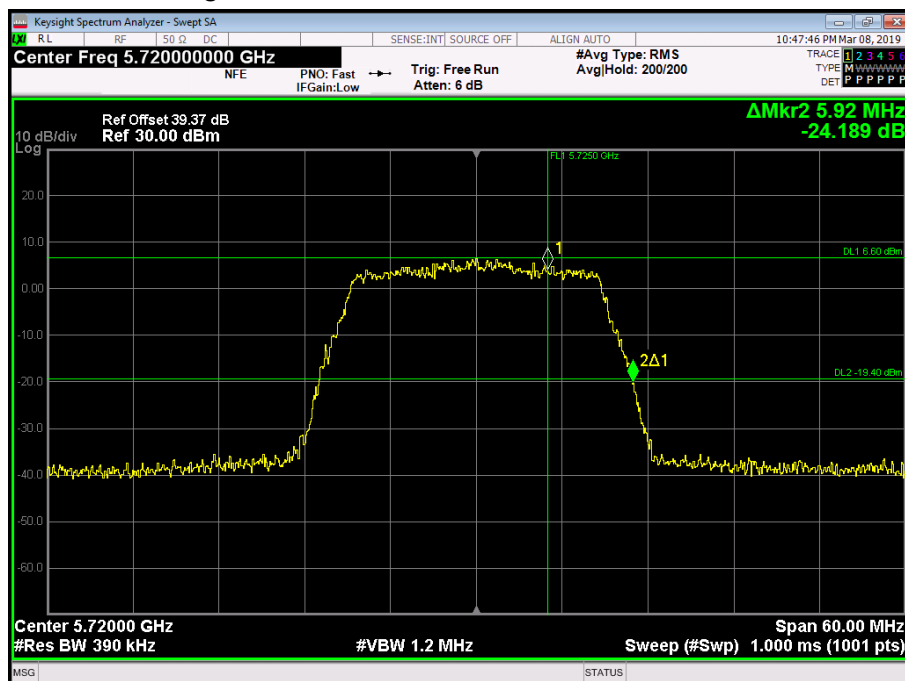
Figure 298 - 5720 MHz - 26 dB Emission Bandwidth
