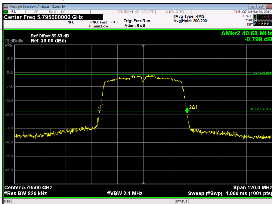
Figure 346 - 5795 MHz - 26 dB Emission Bandwidth
