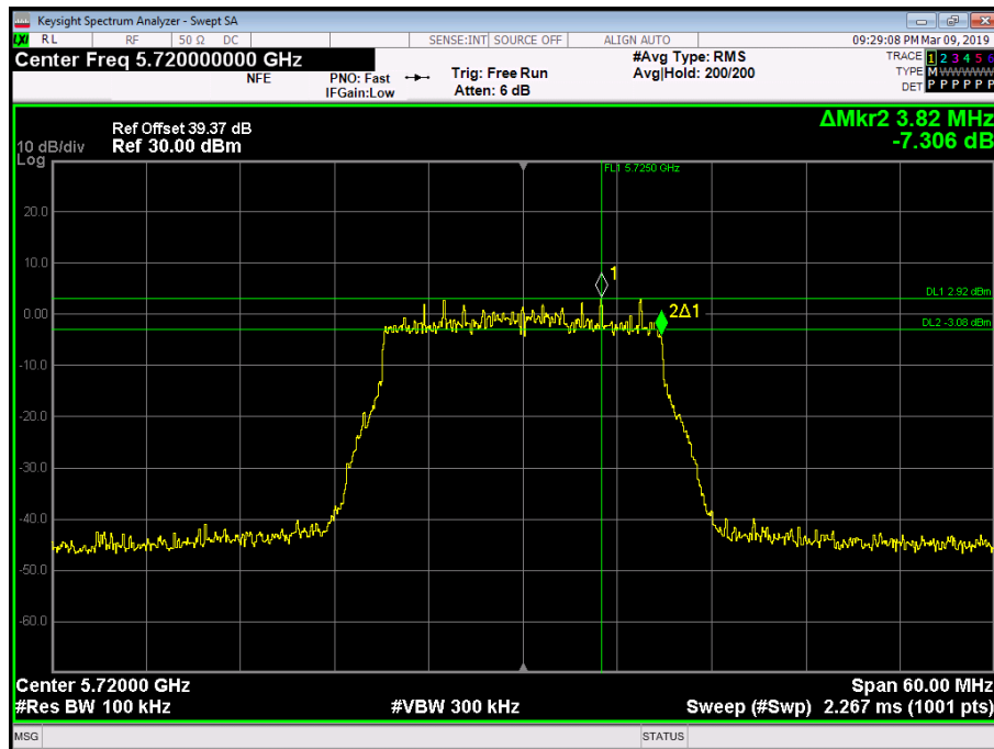
Figure 297 - 5720 MHz - 6 dB DTS Bandwidth
