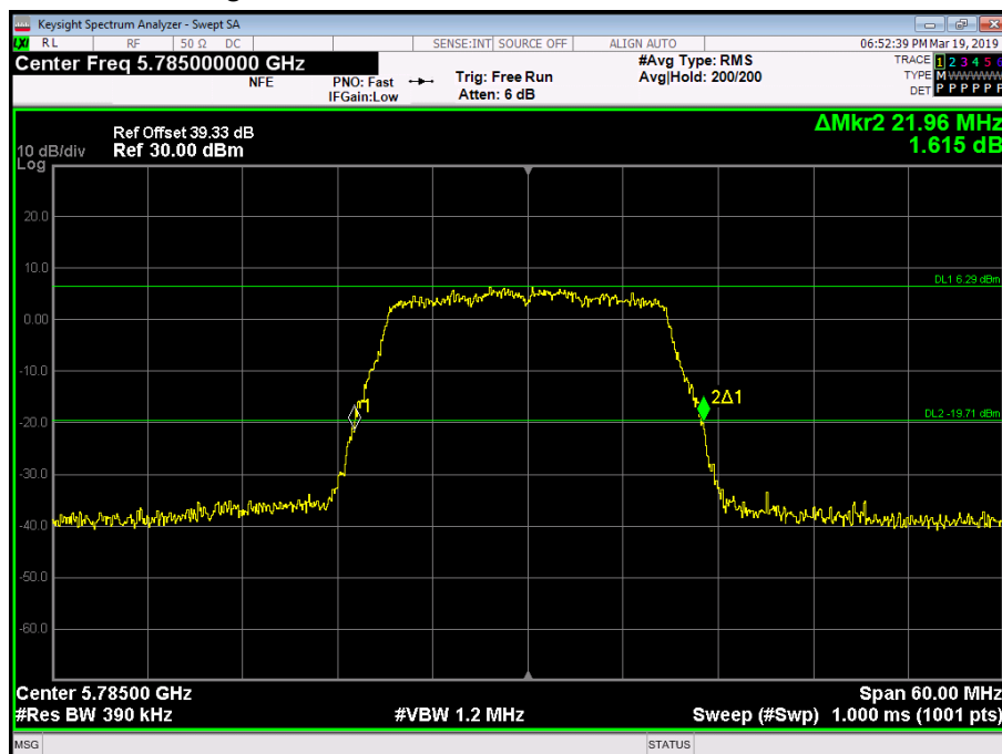
Figure 316 - 5785 MHz - 26 dB Emission Bandwidth
