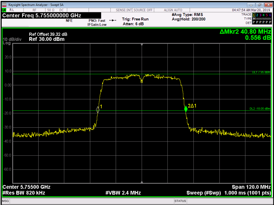
Figure 343 - 5755 MHz - 26 dB Emission Bandwidth
