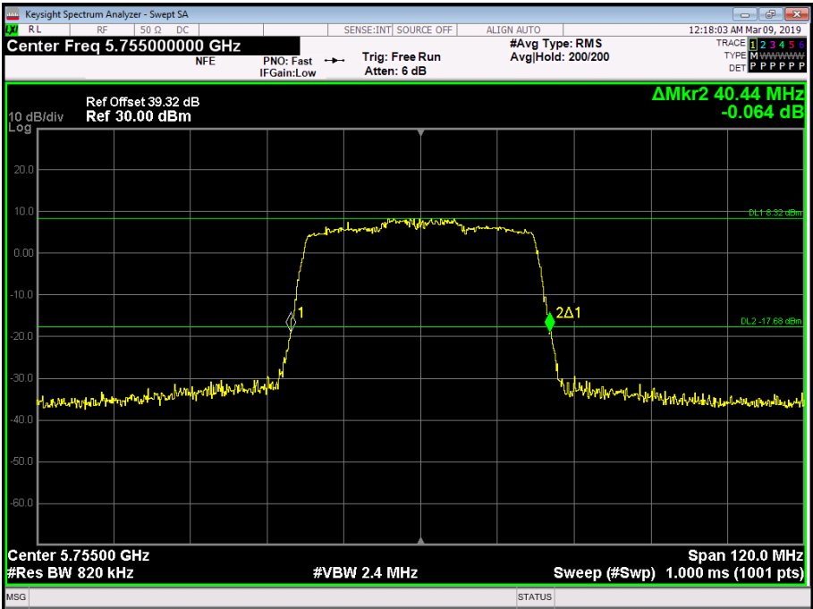
Figure 325 - 5755 MHz - 26 dB Emission Bandwidth
