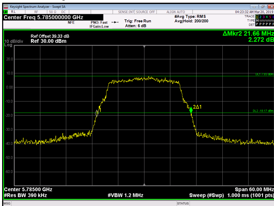
Figure 268 - 5785 MHz - 26 dB Emission Bandwidth
