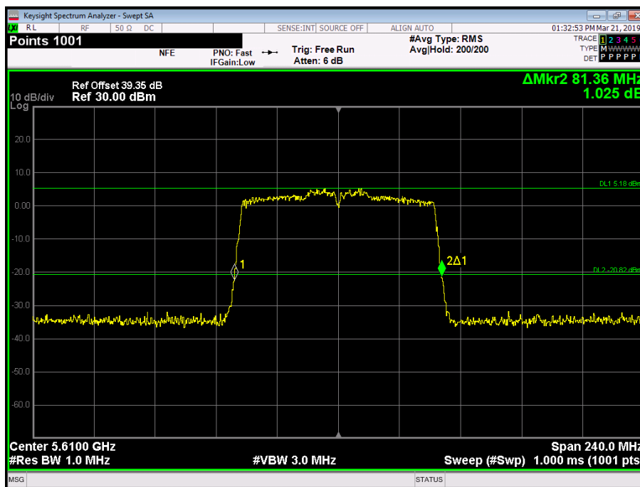
Figure 257 - 5610 MHz - 26 dB Emission Bandwidth
