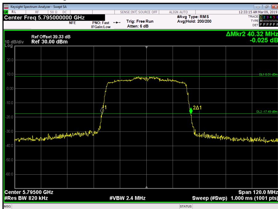
Figure 337 - 5795 MHz - 26 dB Emission Bandwidth
