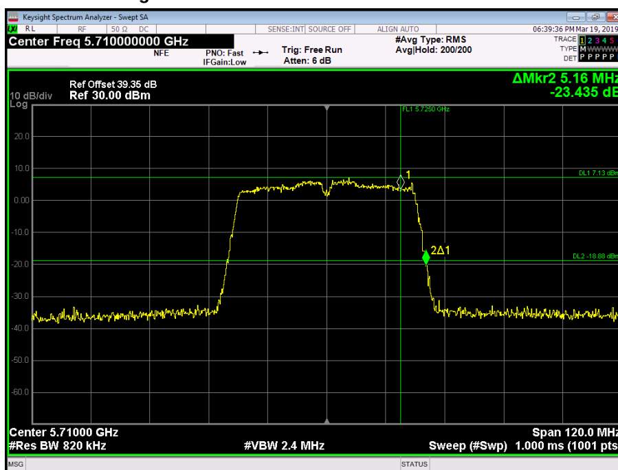
Figure 349 - 5710 MHz - 26 dB Emission Bandwidth
