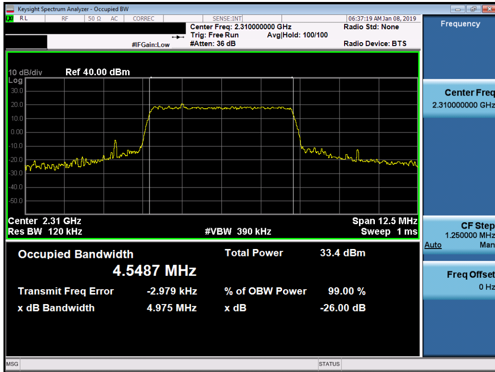
Plot 7-79. Occupied Bandwidth Plot (Band 30 - 5.0MHz QPSK - Full RB Configuration)
