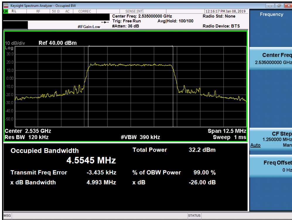
Plot 7-87. Occupied Bandwidth Plot (Band 7 - 5.0MHz 64-QAM - Full RB Configuration)
