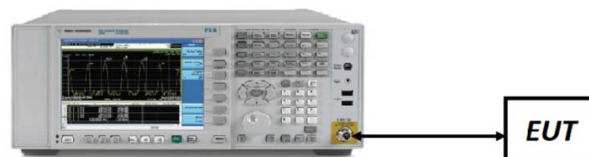
Figure 7-1. Test Instrument & Measurement Setup
