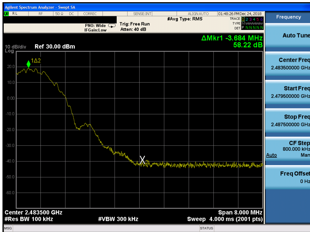
Plot 7-44. Band Edge Plot ANT 1 (Bluetooth (LE), 2Mbps ePA – Ch. 39)
