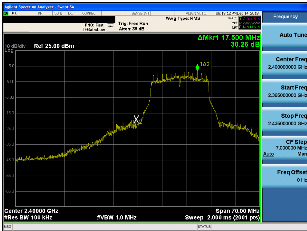
Plot 7-65. Band Edge Plot SISO CORE 1 (802.11g- Ch. 1)
