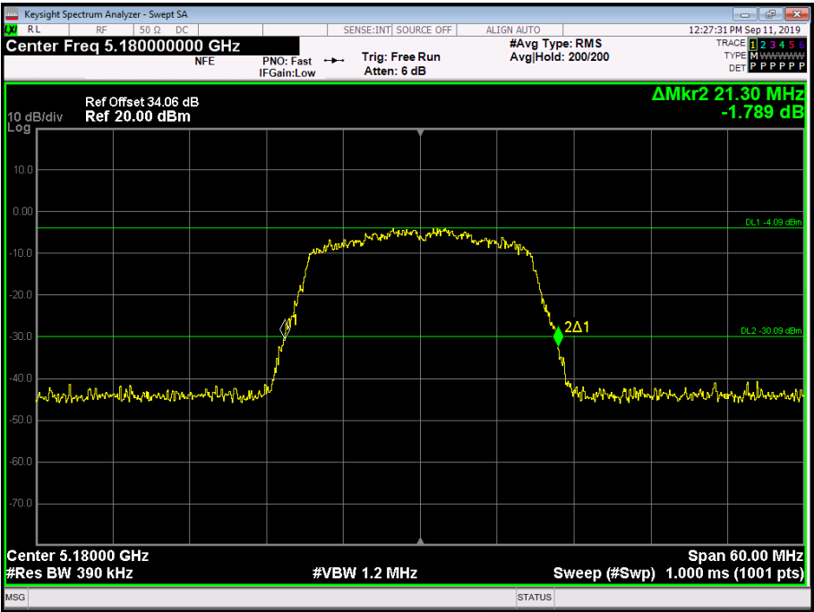
Figure 183 - 5180 MHz - 26 dB Emission Bandwidth
