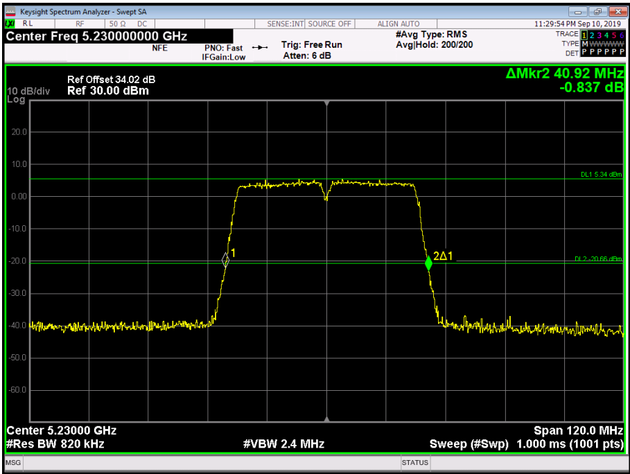
Figure 135 - 5230 MHz - 26 dB Emission Bandwidth
