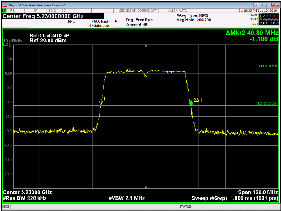
Figure 195 - 5230 MHz - 26 dB Emission Bandwidth
