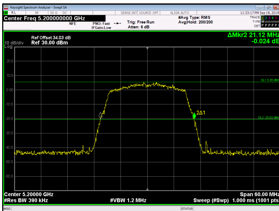
Figure 179 - 5200 MHz - 26 dB Emission Bandwidth
