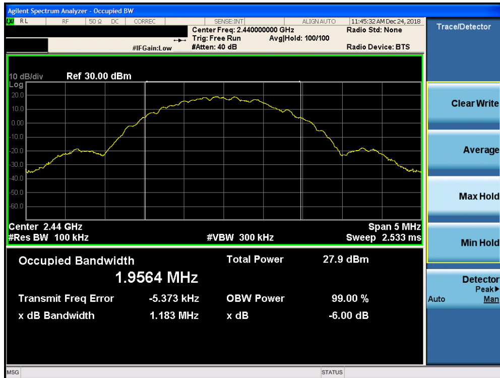
Plot 7-11. 6dB Bandwidth Plot ANT 1 (Bluetooth (LE), 2Mbps ePA – Ch. 19)
