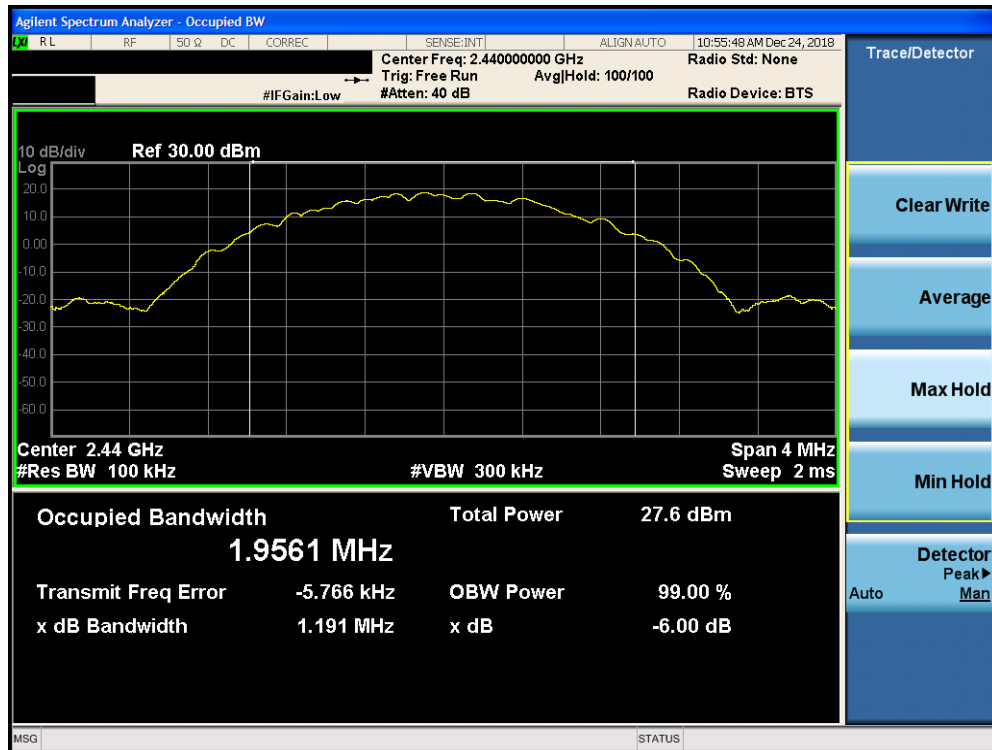
Plot 7-5. 6dB Bandwidth Plot ANT 0 (Bluetooth (LE), 2Mbps ePA – Ch. 19)
