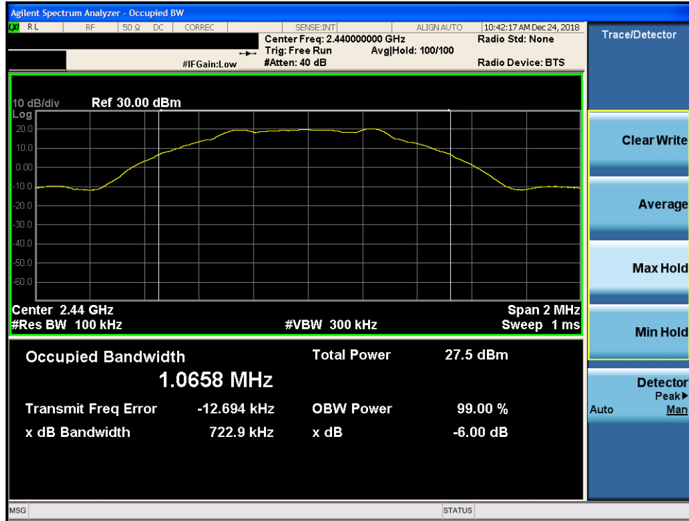
Plot 7-2. 6dB Bandwidth Plot ANT 0 (Bluetooth (LE), 1Mbps ePA – Ch. 19)
