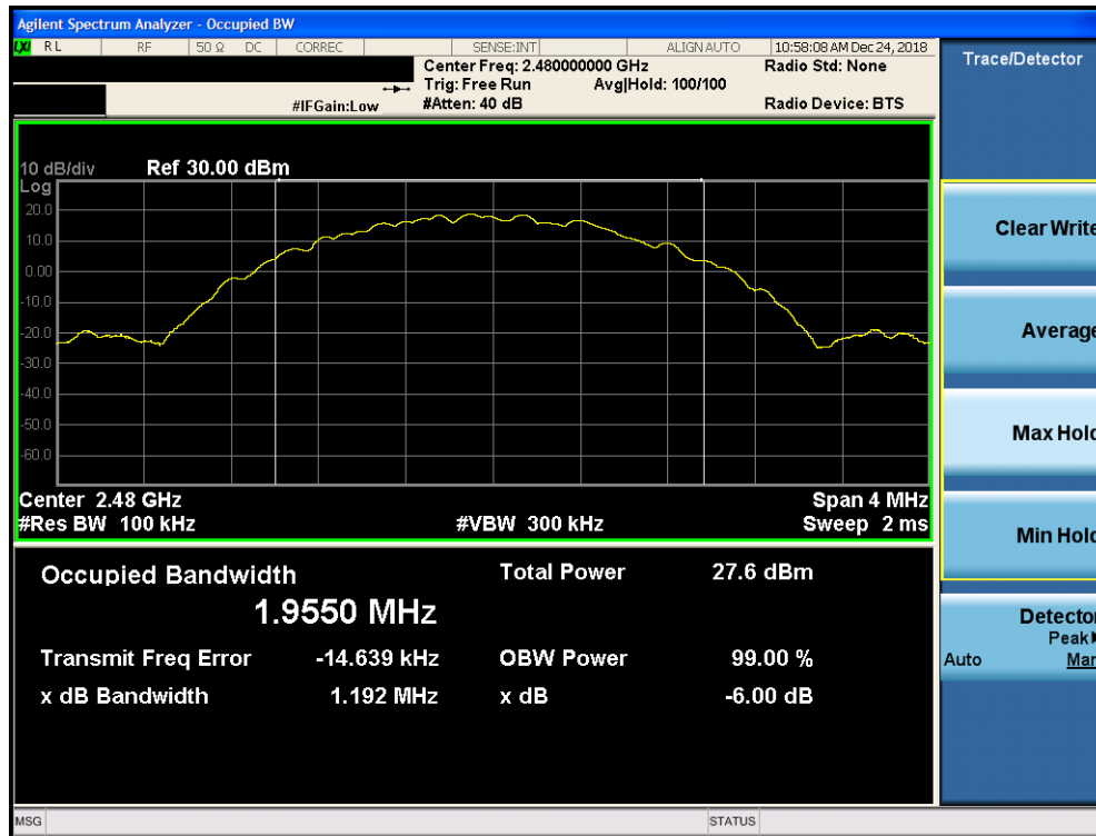
Plot 7-6. 6dB Bandwidth Plot ANT 0 (Bluetooth (LE), 2Mbps ePA – Ch. 39)
