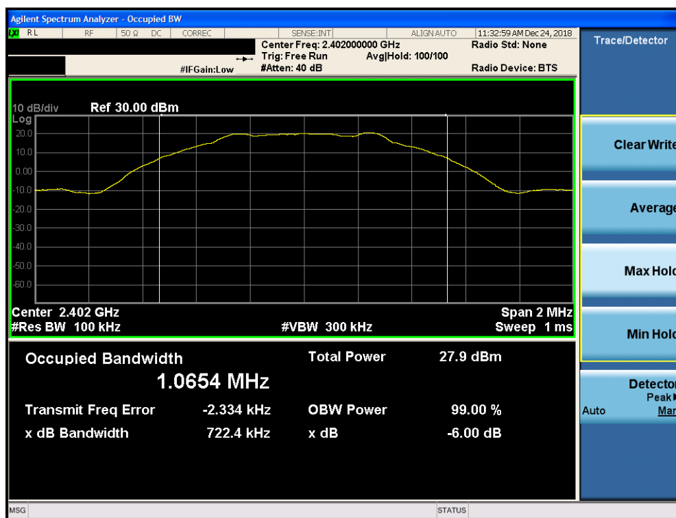
Plot 7-7. 6dB Bandwidth Plot ANT 1 (Bluetooth (LE), 1Mbps ePA – Ch. 0)
