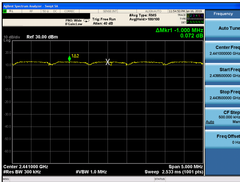
Plot 7-46. Channel Spacing Plot ANT 1 (Bluetooth, 8DPSK, ePA)
