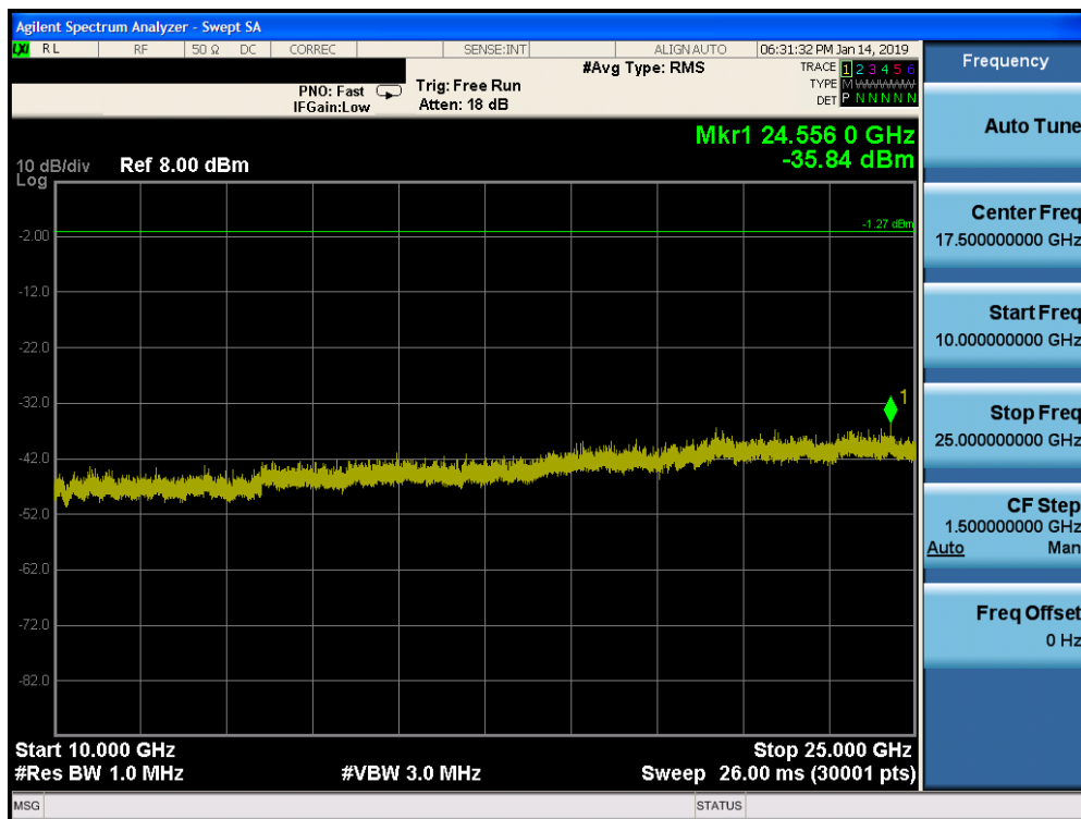
Plot 7-68. Conducted Spurious Plot ANT 0 (Bluetooth, GFSK, ePA – Ch. 0)
