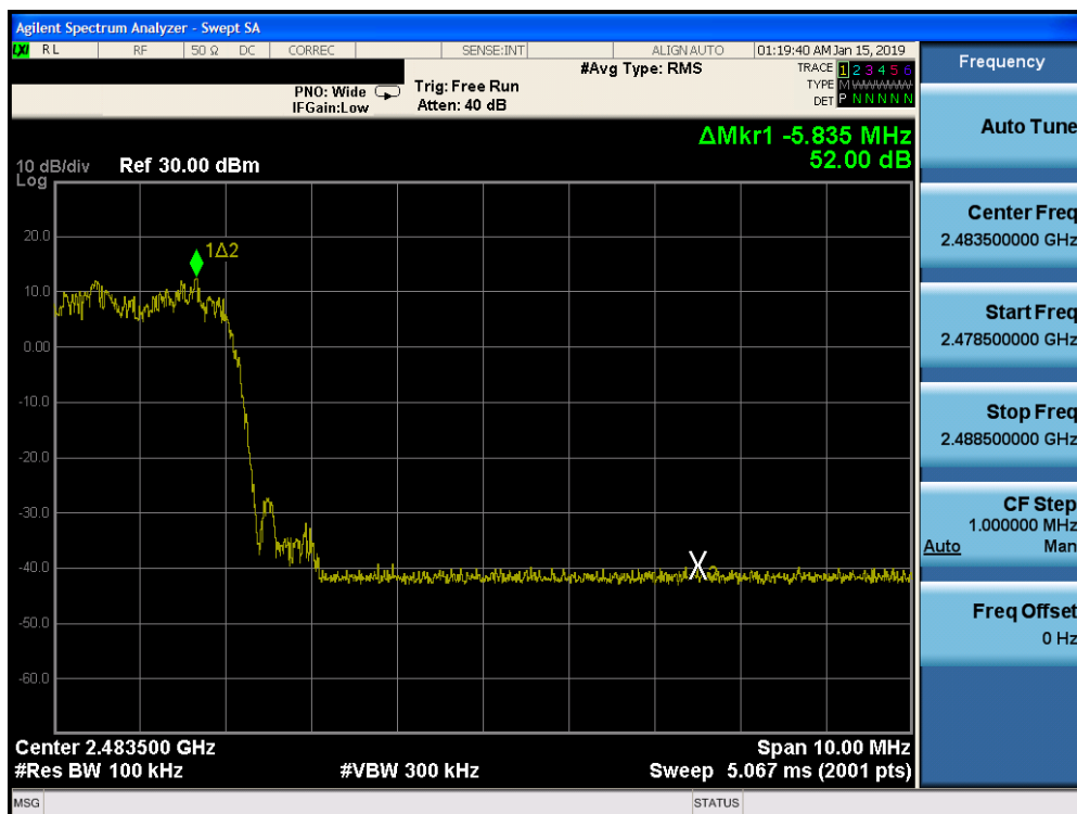
Plot 7-26. Band Edge Plot ANT 0 (Bluetooth with Hopping Enabled, 8DPSK, ePA)
