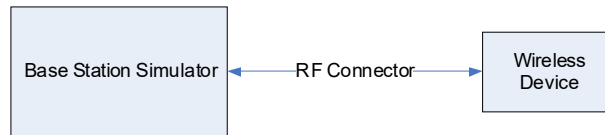
Figure 8-1 Power Measurement Setup
